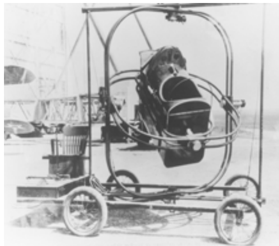
The Ruggles Orientator, developed by Maj William Ocker and Capt Carl Crane in the 1930s, was used in preflight testing to give students the feel of instrument flying. A hood was placed over the cockpit to simulate the conditions of flying at night or under nonvisual circumstances.
