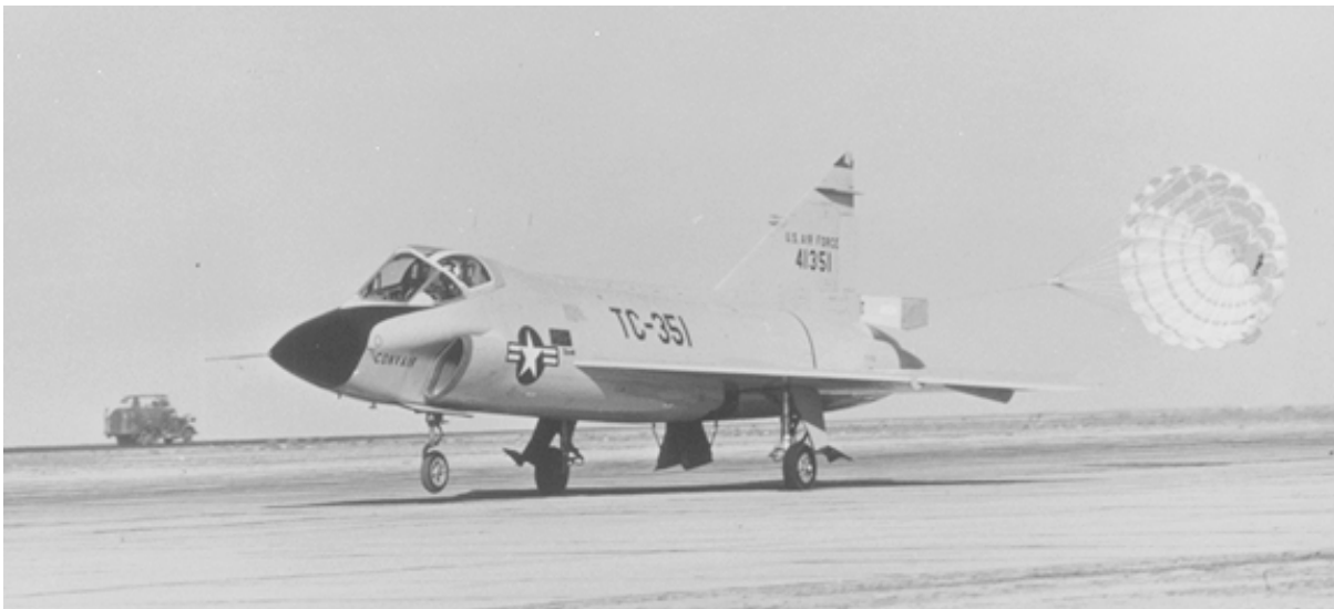
A Convair TF-102A "Delta Dagger" trainer lands at Edwards AFB, California, with a drag chute. This Perrin AFB, Texas, trainer was similar to the F-102A but had a wider front fuselage seating two side-by-side.
