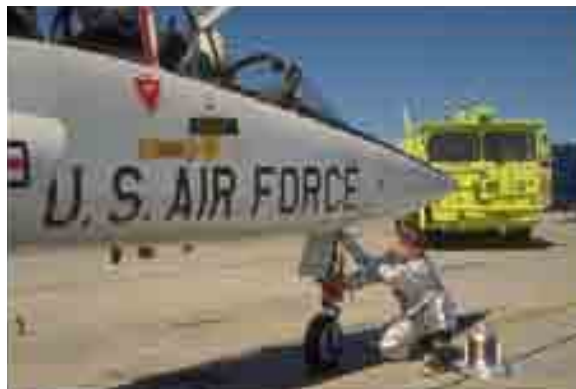
A fireman inspects the nose wheel of a T-38 after a student pilot reported "hot brakes."
