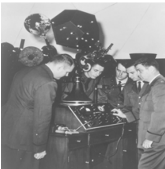
At right, the flight commander of the 3567th Navigator Training Squadron, James Connally AFB, Texas, uses a new astronomical triangle to brief celestial navigation instructors. Any portion of the heavens could be projected on the ceiling of the Spitz planetarium at James Connally for study by navigation students.
