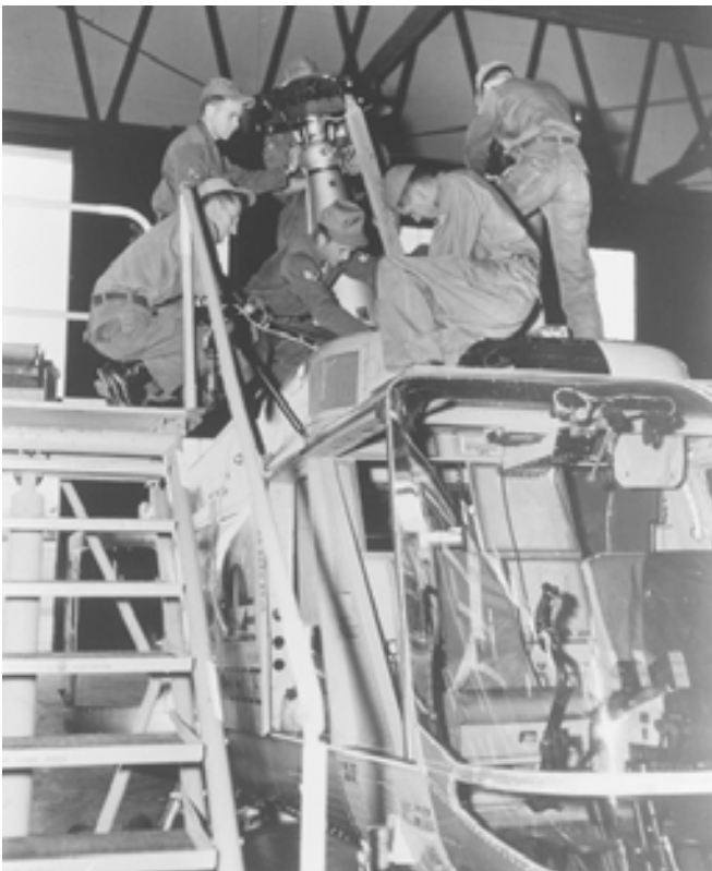
Students learn the techniques of removing an H-33 rotor blade in a helicopter maintenance course.
