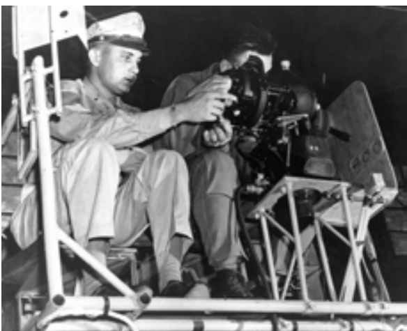
A student atop the A-2 bombing trainer receives instruction on the use of the M-series bombsight.
