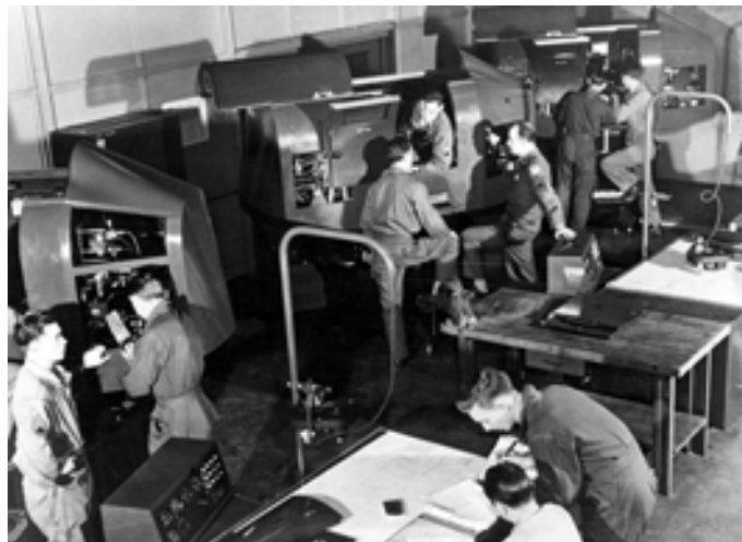
Enlisted personnel at Randolph Field, Texas, received hands-on training using the C-8 synthetic trainer
