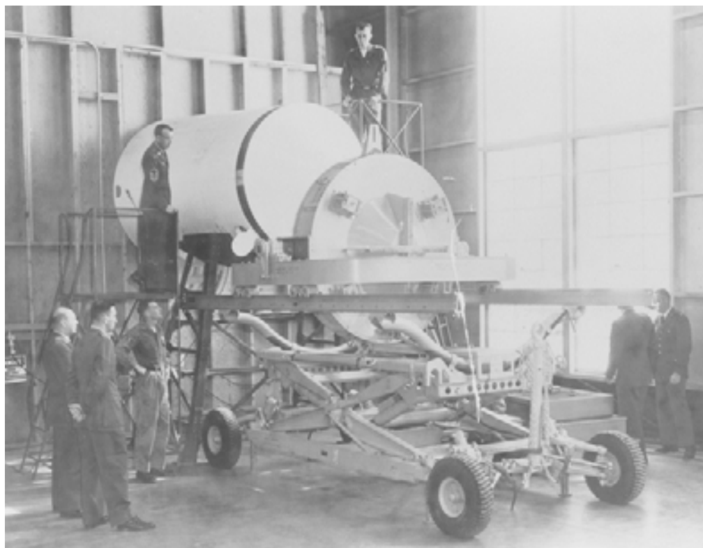
Students in nuclear weapons training at Lowry AFB, Colorado, learn to mate the re-entry vehicle to the Thor intermediate range ballistic missile.
