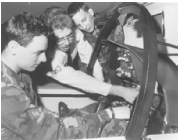
Avionics students at Sheppard AFB, Texas, perform an operations check of an F-15 avionics maintenance trainer.
