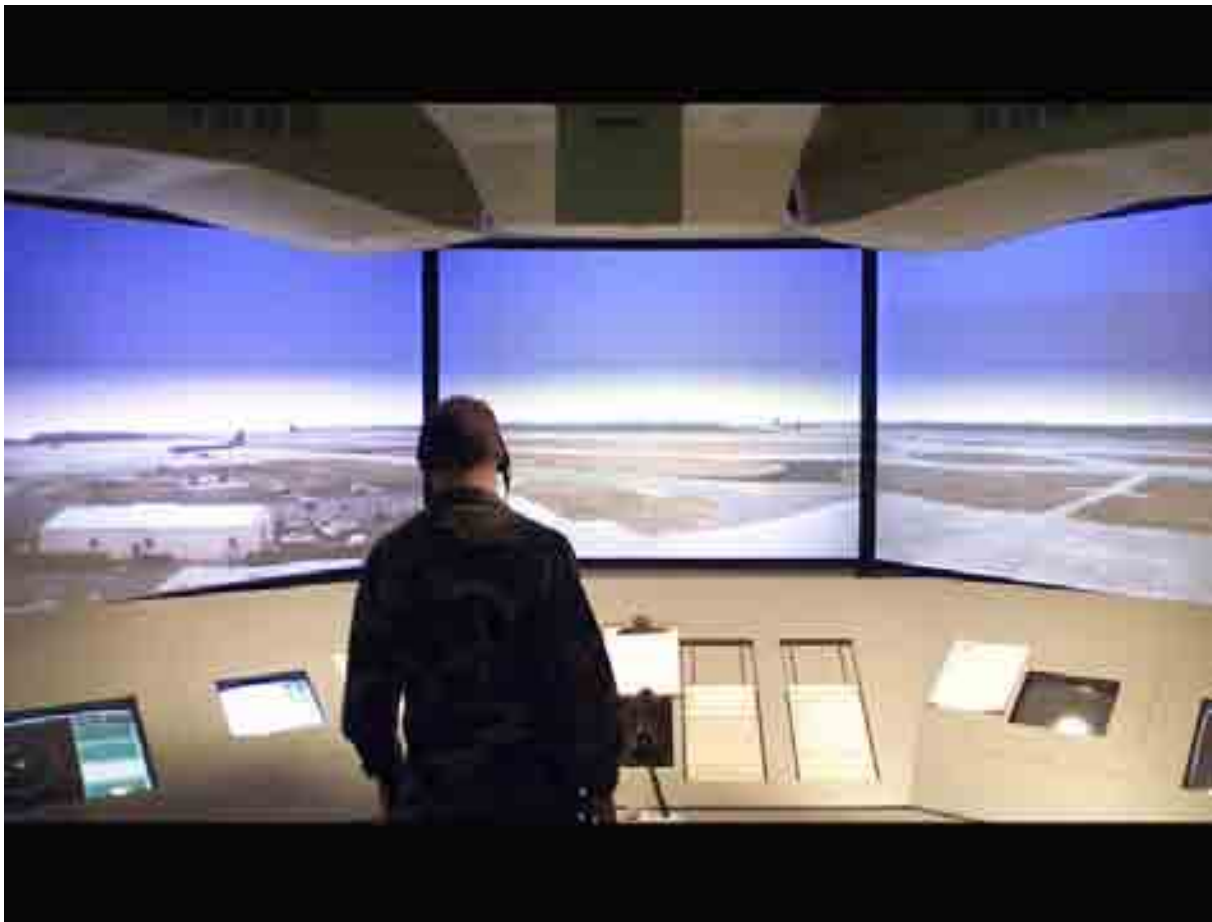
A1C Danny Zickafoose clears jets for takeoff at the notional Canyon AFB, a virtual runway created by a simulator in the air traffic control schoolhouse at Keesler.
