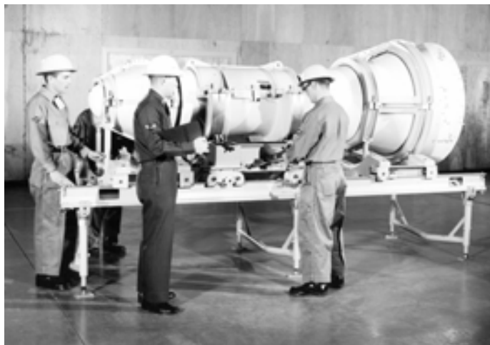
Students attending the Nuclear Weapons Specialist (Reentry Vehicles) Course at Lowry Technical Training Center, Colorado, "learn by doing" as they attach the Mark VIII warhead to the Mark III nose module.
