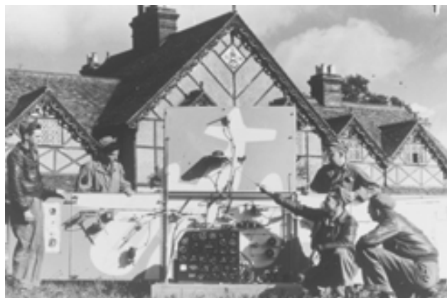
A mobile training unit instructor points out the remote compass transmitter to instrument specialists on the A-26. This training took place on an English estate.
