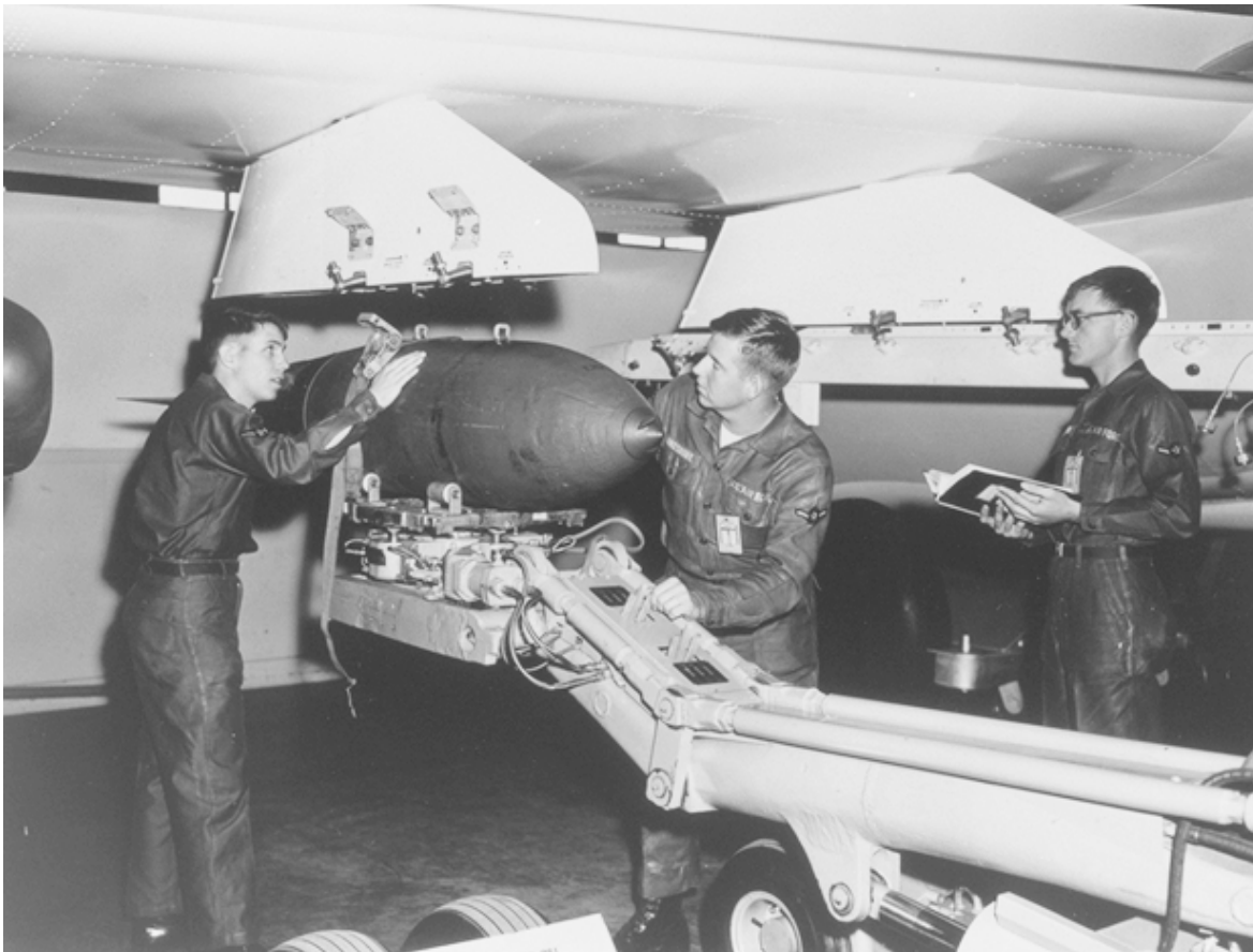
Students in the weapons mechanic course at Lowry AFB, Colorado, load a 750-pound bomb on an F-111A simulator.
