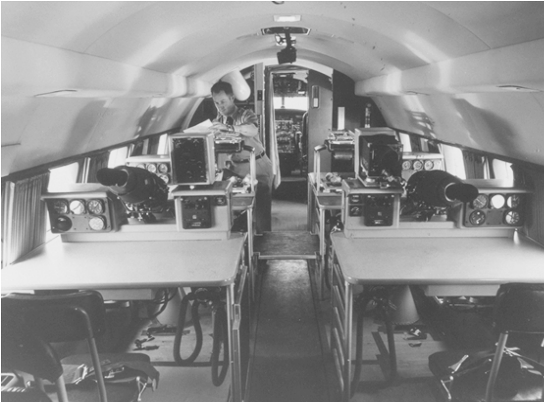
This is an interior view of the Convair T-29D, which ATC used for navigator training. The "D" model had no astrodomes and carried six students and an instructor.
