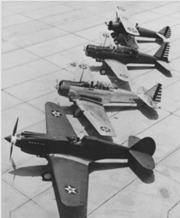
At Tuskegee Field these four aircraft were the preferred trainers during the war: top to bottom, the PT-17, primary; the BT-13, basic; the AT-6, advanced; and the P-40, transition.
