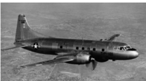
The T-29D observer trainer aircraft had stations for six students and two instructors on board the flying classroom.
