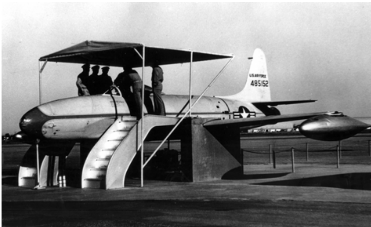
Synthetic trainers such as the F-80 Captivair were money savers, as well as time savers. Instructors considered them an excellent way for students to develop muscular and mental coordination. (In June 1947 the "P" for pursuit changed to "F" for fighter.)
