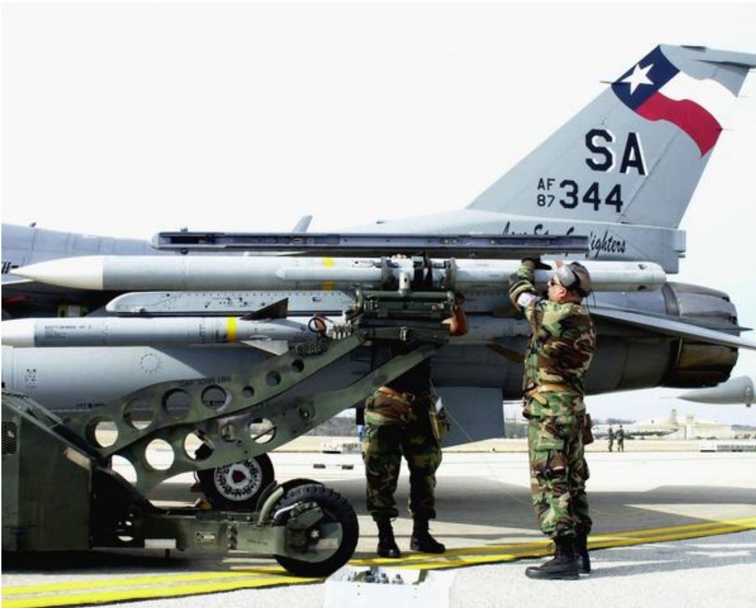
US Air Force personnel assigned to the Aircraft Generation Squadron (AGS), 149th Fighter Wing, Texas Air National Guard, secure an AIM-120 Advanced Medium Range Air-to-Air Missile (AMRAAM) onto an F-16 using a MJ-1 weapons loader at Kelly Field Annex, Lackland AFB, Texas.
