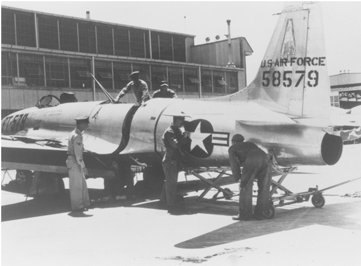
The F-80 jet mechanics training program included disassembling the fuselage to remove the power plant for the 25-hour inspection.
