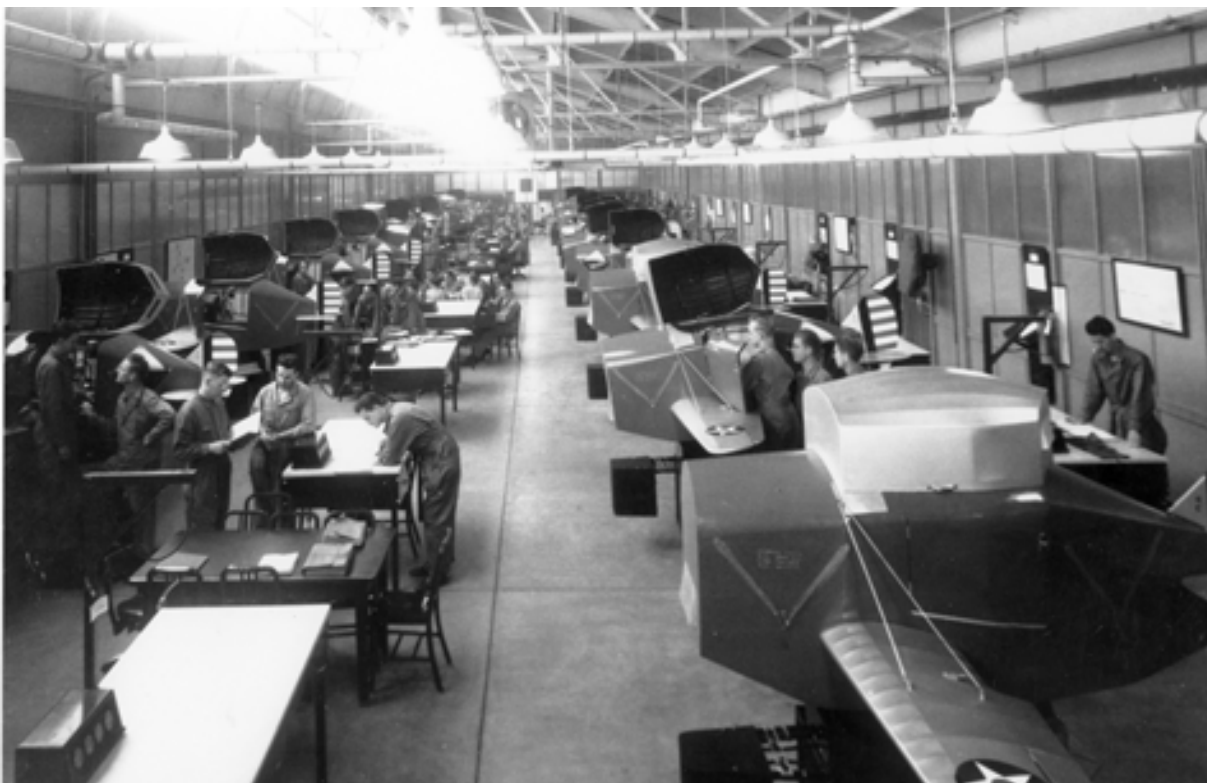
Rows of Link trainers fill this Chanute Field, Illinois, classroom. These trainers were used to teach both Link trainer operators and maintenance technicians.
