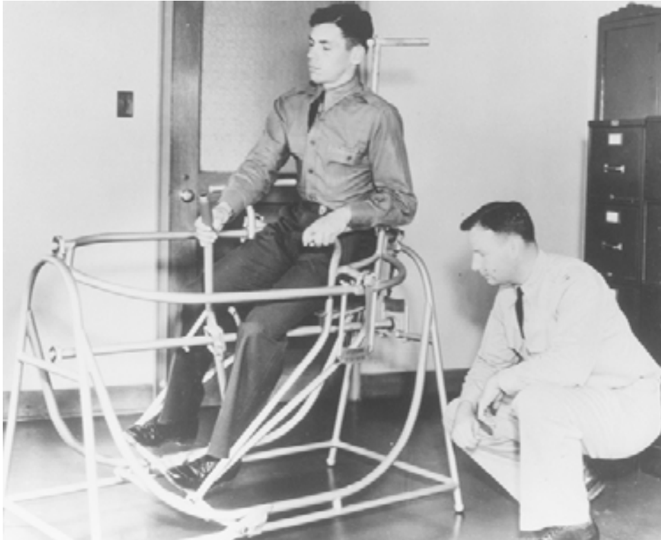
To study equilibrium, specialists at the School of Aviation Medicine, Randolph Field, Texas used the blueprints of Danish inventors to build this Danish Balancing Chair.
