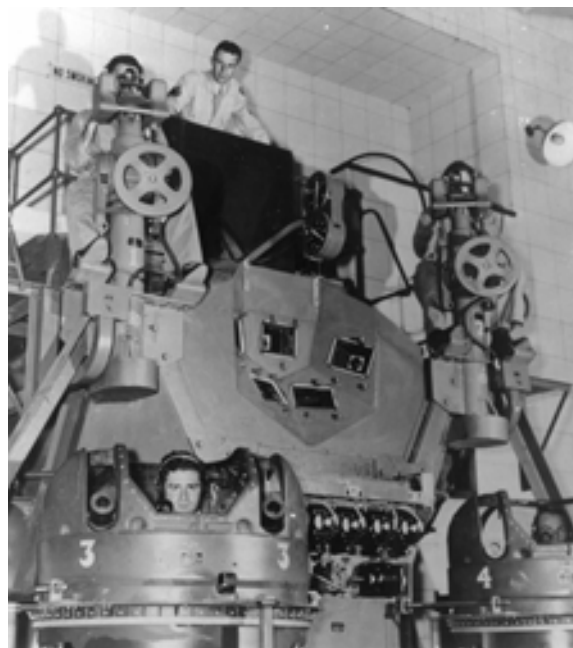
Flexible gunnery students at Harlingen Field, Texas, used a Waller Trainer to "fire" at approaching planes projected on a screen.
