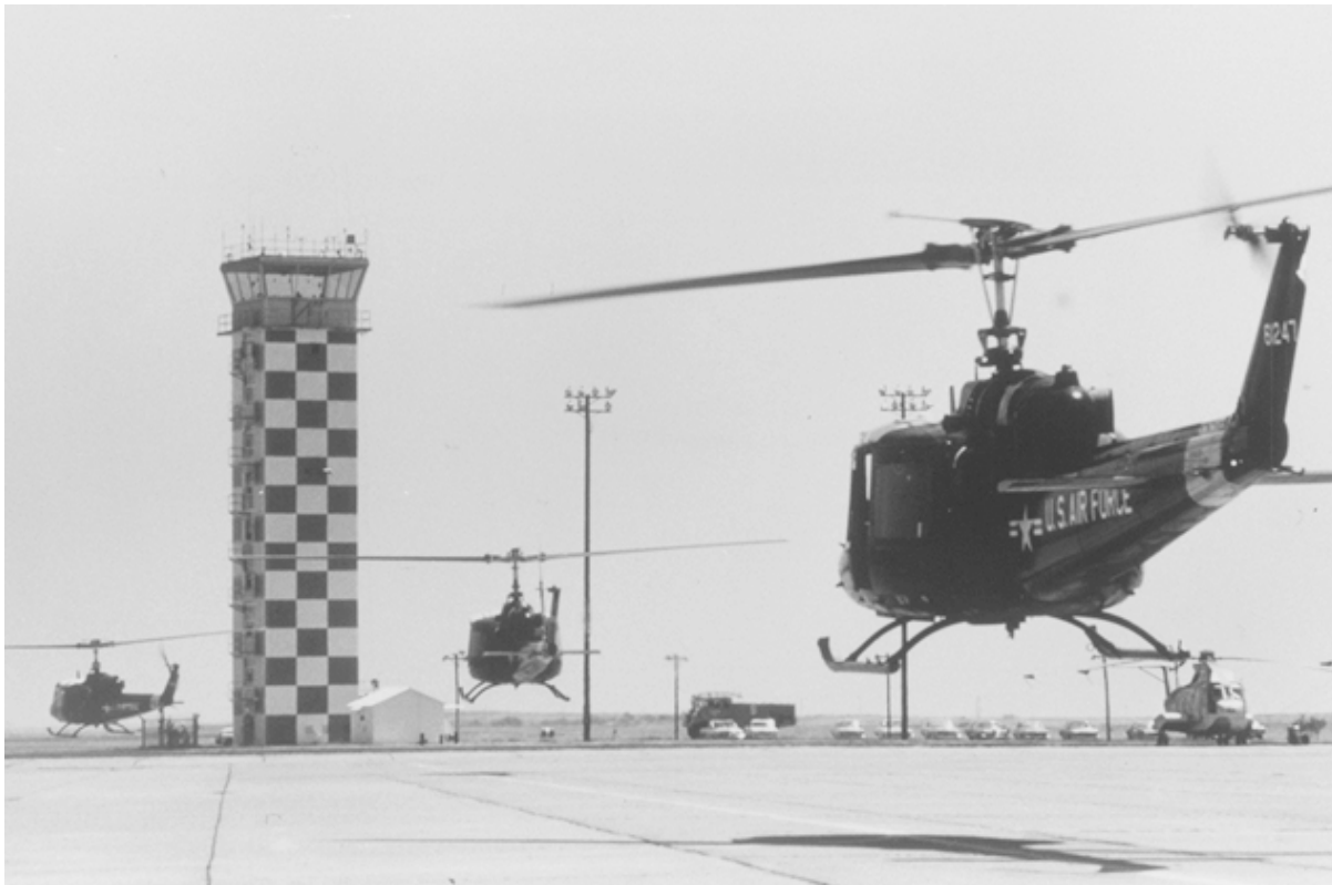
Air Training Command used the Bell TH-1F turbine-engine helicopter in its undergraduate helicopter pilot training program. When the prototype of this helicopter was ordered into production it was designated the HU-1A and named the Iroquois. The HU designation gave rise to the nickname "Huey" which was unofficial but more frequently used than Iroquois.
