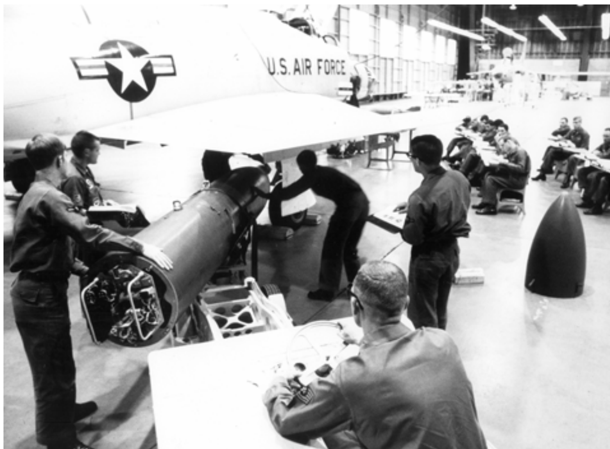
Instructors closely monitor students installing an electronics pod on an F-4D aircraft during classes at Sheppard AFB, Texas.
