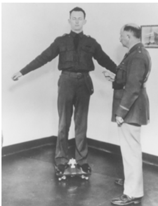
In the 1930s, the Wobblemeter was used as a screening device to check balance and orientation.
