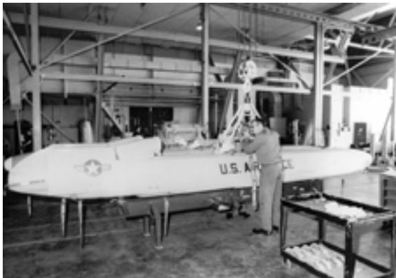
An armament student uses a laser gun to align the AGM-86B air-launched cruise missile to its mount.
