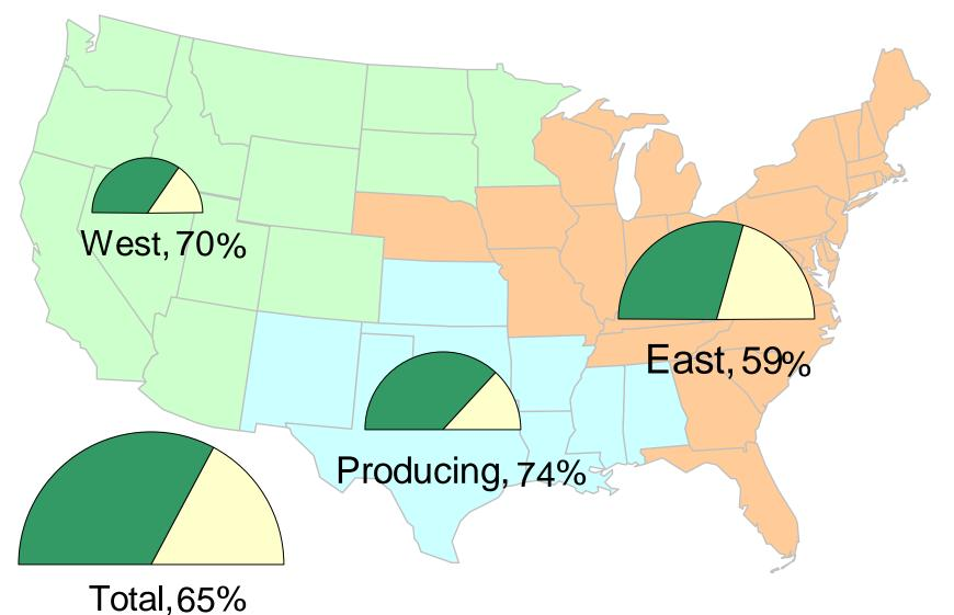
Source: Derived from EIA Storage and Estimated Working Gas Capacity data
