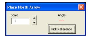
Pick the "Pick Reference" button – choose the reference file to set the rotation, this can be the alignment, the mapping, the contours or any other reference file since they are all rotated to the same degree. The North Arrow then is ready to be placed. You can change the scale of the North Arrow any time before placing.
