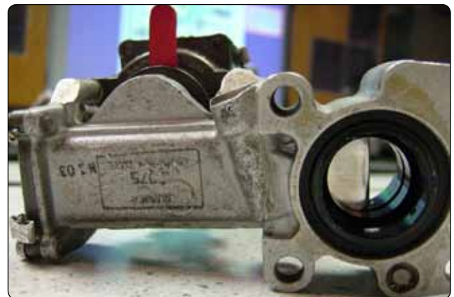
Figure 14-41. This motor-operated gate valve has a red position indicating lever that can be used by maintenance personnel to identify the position of the valve. The lever can be moved by the technician to position the valve.
