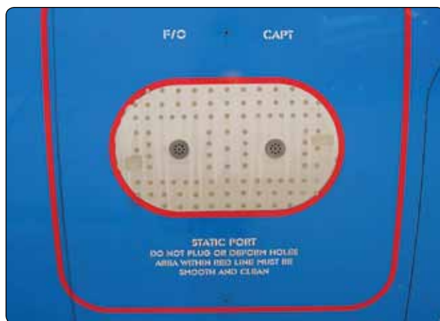
Figure 10-26. Heated primary and alternate static vents located on the sides of the fuselage.
