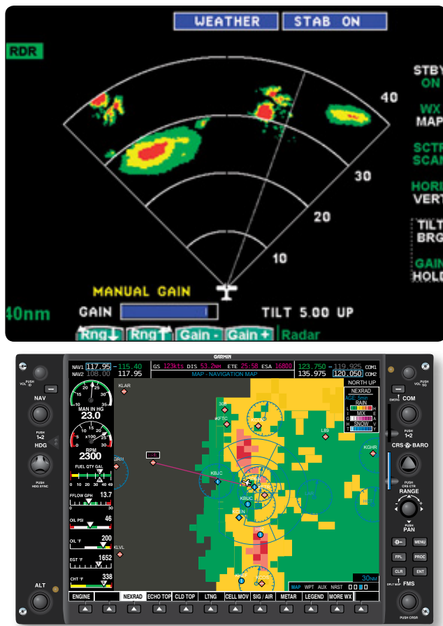
Figure 11-142. A dedicated weather radar display (top) and a multifunctional navigation display with weather radar overlay (bottom).
