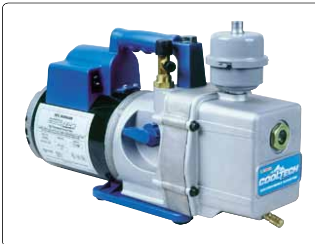
Figure 16-91. A vacuum pump is used to lower the pressure in the vapor cycle air conditioning system. This reduces the boiling point of water in the system, which vaporizes and is drawn out by the pump.
