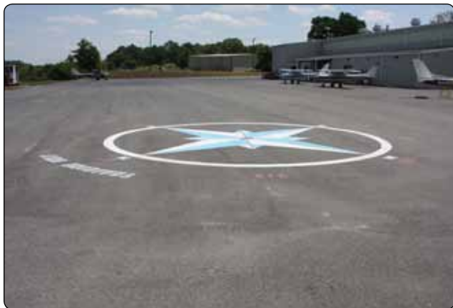
Figure 10-140. The compass rose on this airport ramp can be used to swing an aircraft magnetic compass.
