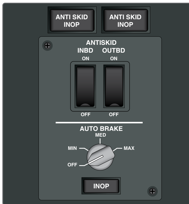
Figure 13-105. Antiskid switches in the cockpit.
