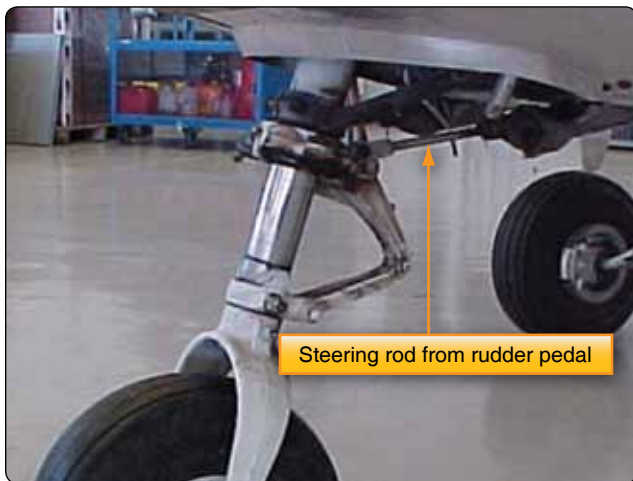
Figure 13-50. Nose wheel steering on a light aircraft often uses a push-pull rod system connected to the rudder pedals.
