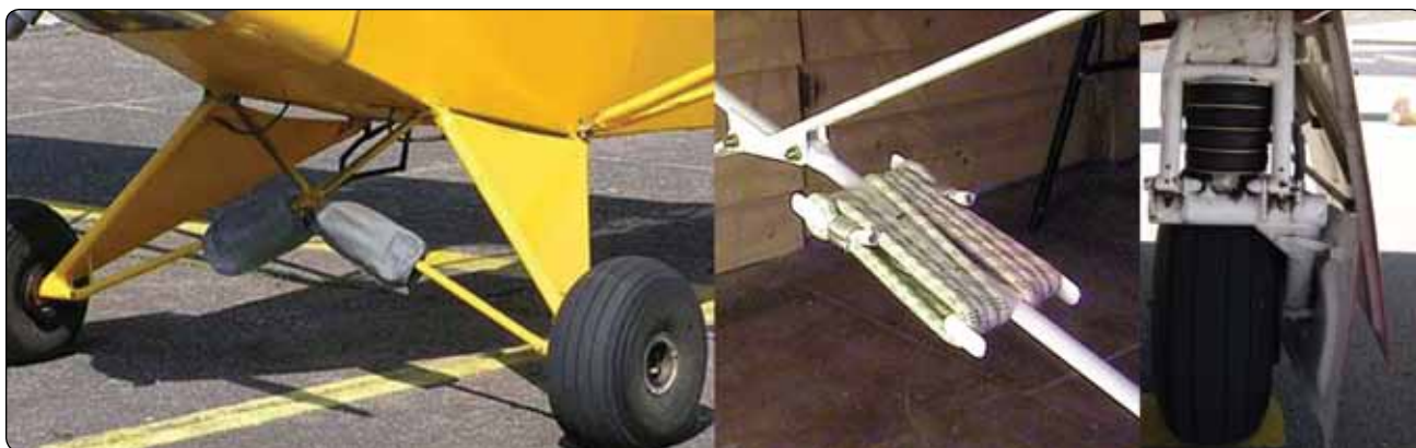
Figure 13-15. Piper Cub bungee cord landing gear transfer landing loads to the airframe (left and center). Rubber, donut-type shock transfer is used on some Mooney aircraft (right).
