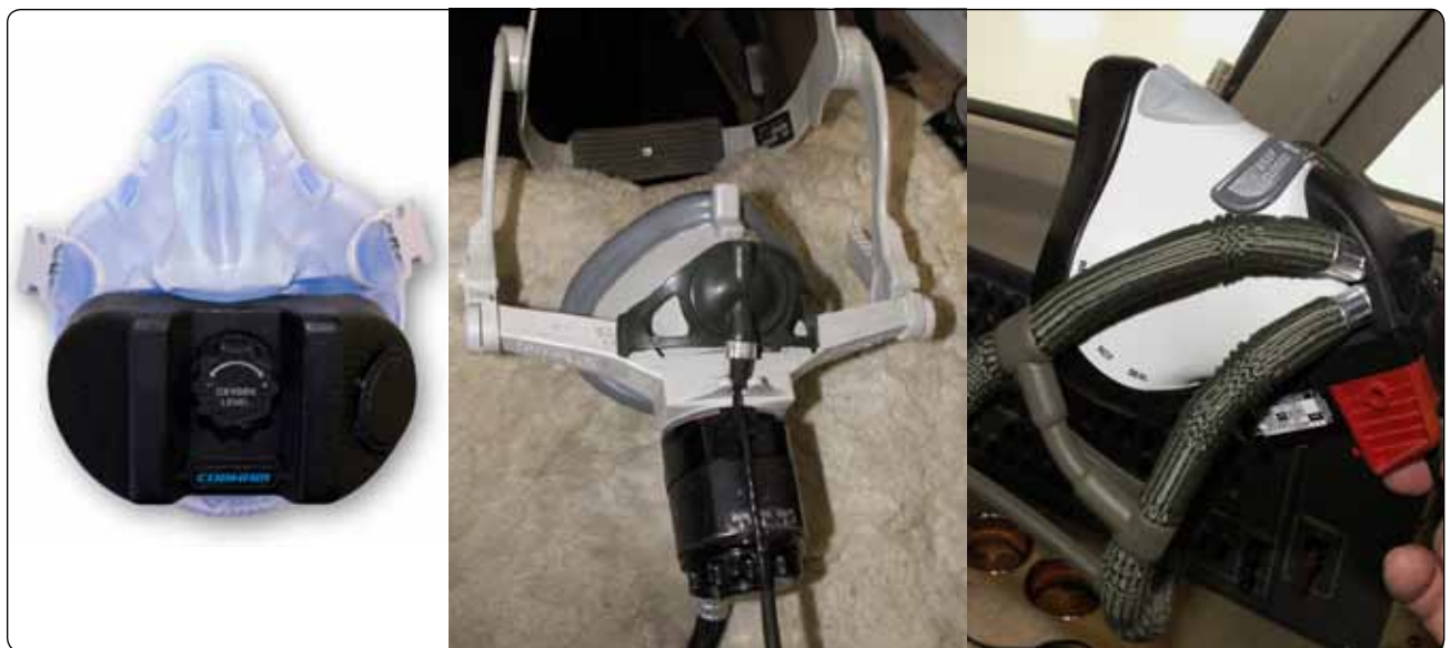
Figure 16-22. A mask-mounted version of a miniature diluter-demand regulator designed for use in general aviation (left), a mechanical quick-donning diluter-demand mask with the regulator on the mask (center), and an inflatable quick-donning mask (right). Squeezing the red grips directs oxygen into the hollow straps.
