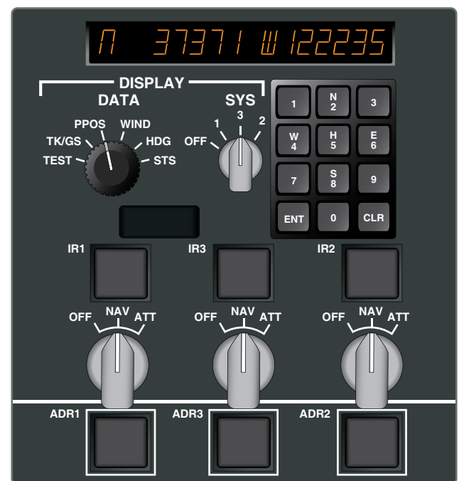
Figure 11-155. An interface panel for three air data and inertial reference systems on an Airbus. The keyboard is used to initialize the system. Latitude and longitude position is displayed at the top.
