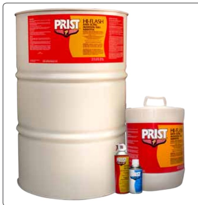
Figure 14-10. Fuel anti-icing products, such as Prist®, act as antifreeze for any free water in aircraft fuel. They dissolve in the water and lower its freezing point to prevent ice crystals from disrupting fuel flow.
