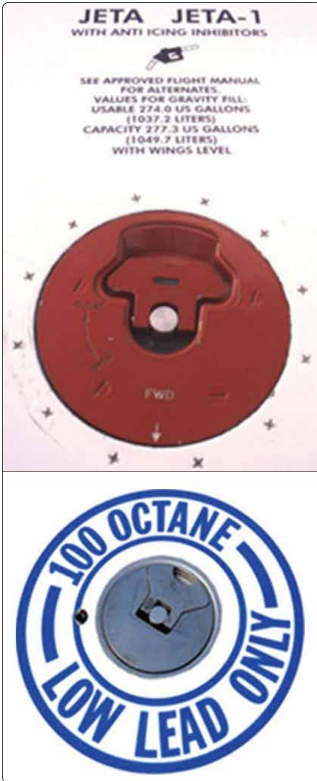
Figure 14-98. All entry points of fuel into the aircraft are marked with the type of fuel to be used. Never introduce any other fuel into the aircraft other than that which is specified.
