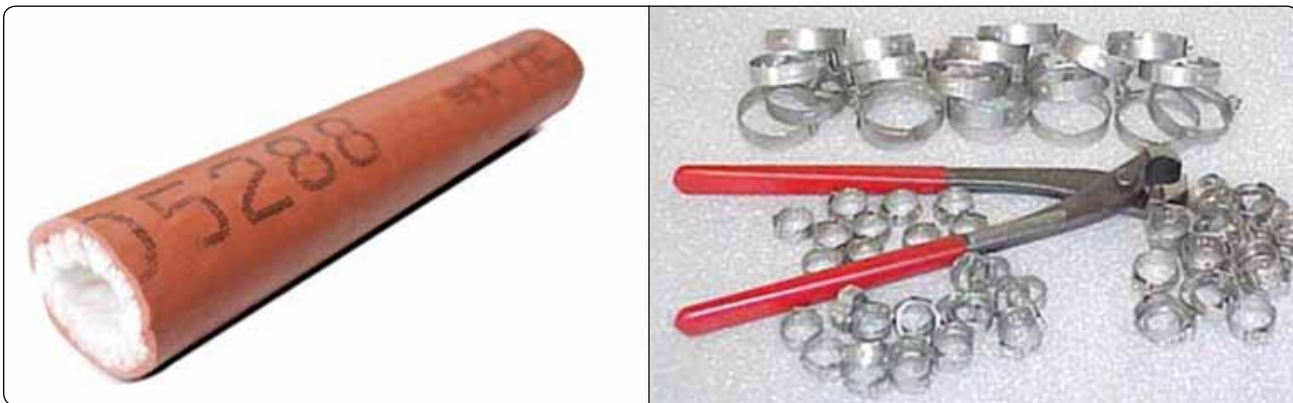
Figure 14-37. Exterior fuel hose wrap that protects from fire, as well as abrasion, shown with the clamps and pliers used to install it.
