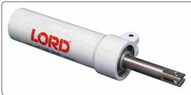
Figure 13-56. A non-hydraulic shimmy damper uses a rubber piston with lubricant that dampens via motion against the inner diameter of the unit housing.
