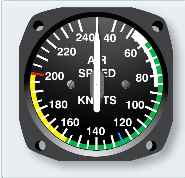
Figure 10-137. An airspeed indicator makes extensive use of range markings.
