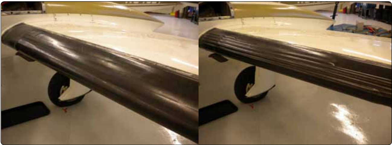
Figure 15-31. Deicing boots inflated (left) and deflated (right).
