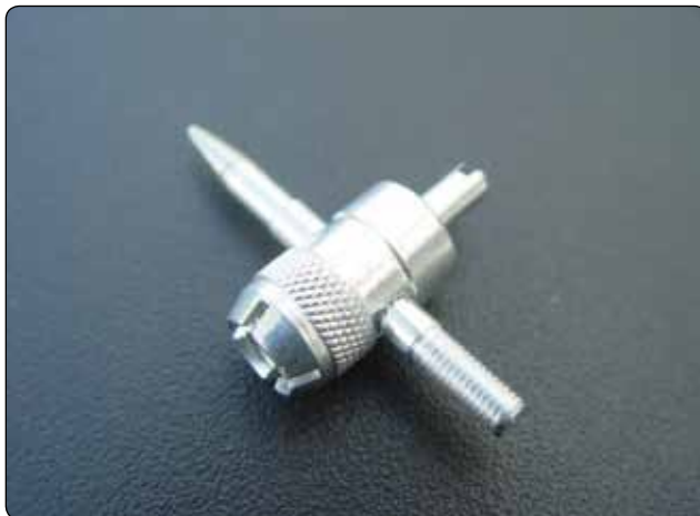
Figure 13-27. This valve tool features internal and external thread chasers, a notched valve core removal/installation tool, and a tapered end for depressing a valve core or clearing debris.
