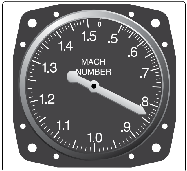
Figure 10-45. A Machmeter indicates aircraft speed relative to the speed of sound.
