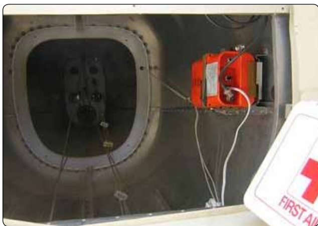
Figure 11-149. An emergency locator transmitter (ELT) mounting location is generally far aft in a fixed-wing aircraft fuselage in line with the longitudinal axis. Helicopter mounting location and orientation varies.
