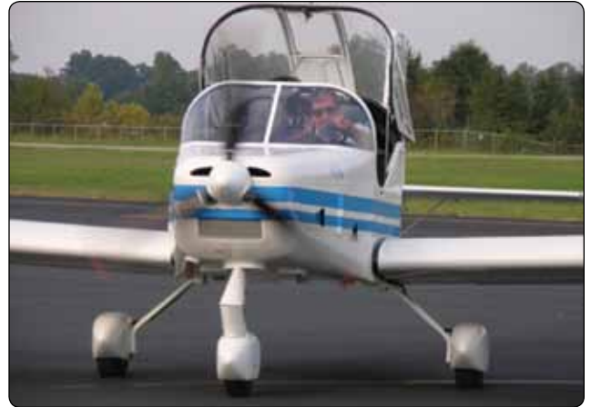
Figure 13-13. Non-shock absorbing struts made from steel, aluminum, or composite material transfer the impact forces of landing to the airframe at a non-damaging rate.
