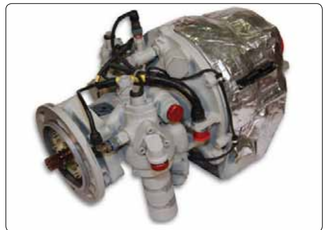
Figure 12-5. Hydraulic power pack.
