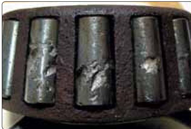
Figure 13-65. Spalling is a chipped away portion of the hardened surface of a bearing roller or race.
