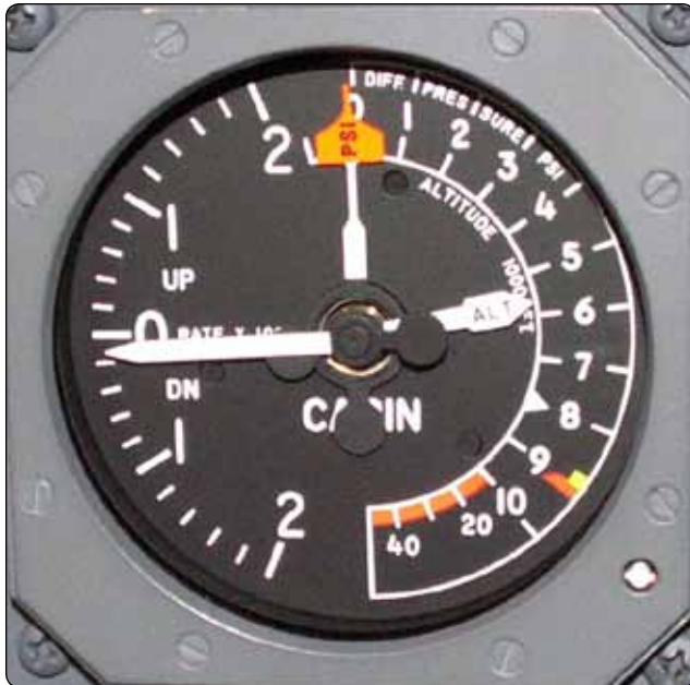
Figure 16-57. This cabin pressurization gauge is a triple combination gauge. The long pointer operates identically to a vertical speed indicator with the same familiar scale on the left side of the gauge. It indicates the rate of change of cabin pressure. The orange PSI pointer indicates the differential pressure on the right side scale. The ALT indicator uses the same scale as the PSI pointer, but it indicates cabin altitude when ALT indicator moves against it.
