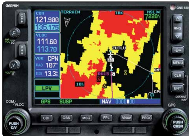
Figure 11-153. A GPS unit integrated with NAV/COM circuitry.
