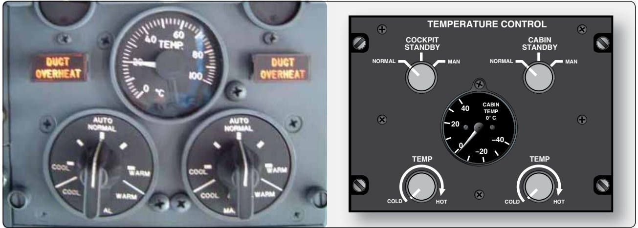
Figure 16-70. Typical temperature selectors on a transport category aircraft temperature control panel in the cockpit (left) and a business jet (right). On large aircraft, temperature selectors may be located on control panels located in a particular cabin air distribution zone.
