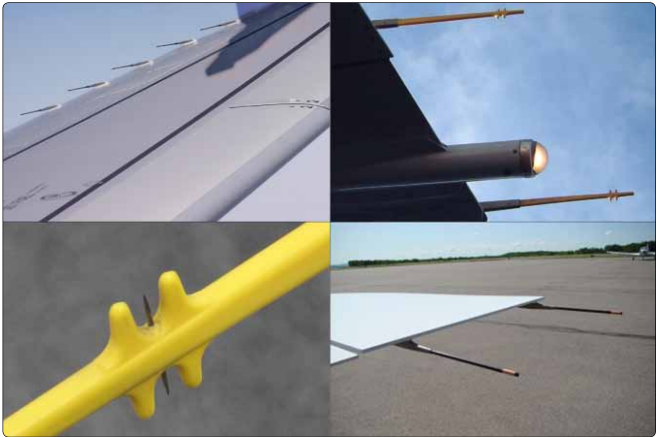
Figure 11-160. Static dischargers or wicks dissipate built up static energy in flight at points a safe distance from avionics antennas to prevent radio frequency interference.
