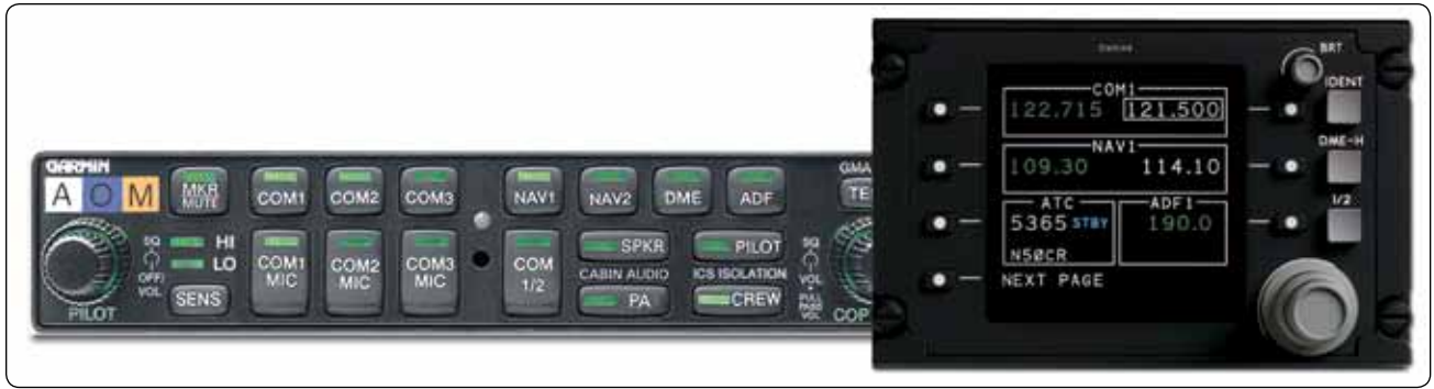
Figure 11-73. An audio panel in a general aviation aircraft integrates the selection of several radio-based communication and navigational aids into a single control panel (left). A digital tuner (right, Image © Rockwell Collins, Inc.) does the same on a business class aircraft and allows the frequency of each device to be tuned from the same panel as well.
