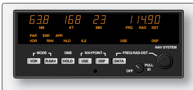
Figure 11-124. RNAV unit from a general aviation aircraft.
