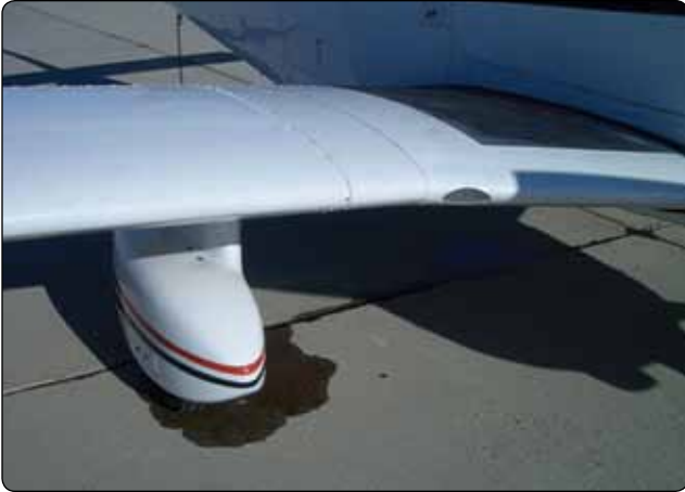
Figure 13-120. The cause of all aircraft brake leaks must be investigated, repaired, and tested before releasing the aircraft for flight.
