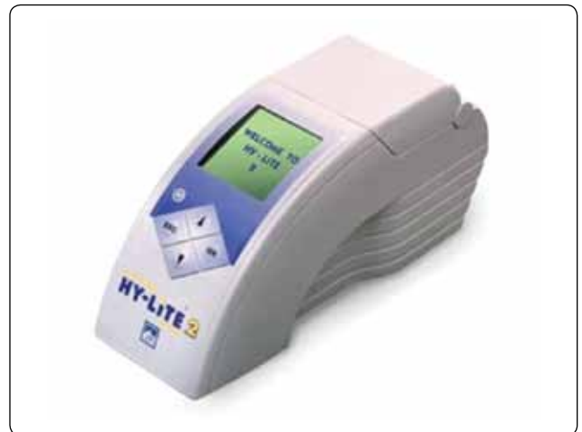
Figure 14-100. A capture solution is put into a 1 liter sample of fuel and shaken. The solution is then put into the analyzer shown to determine the level of microorganisms in the fuel.
