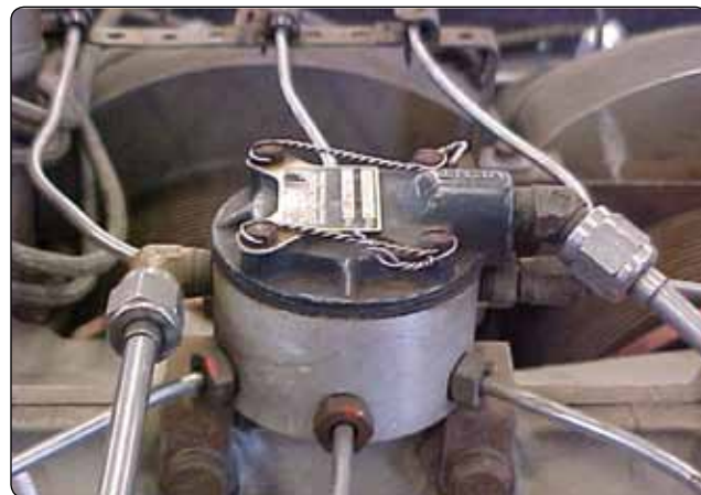
Figure 14-16. A fuel distribution manifold for a fuel-injected engine.
