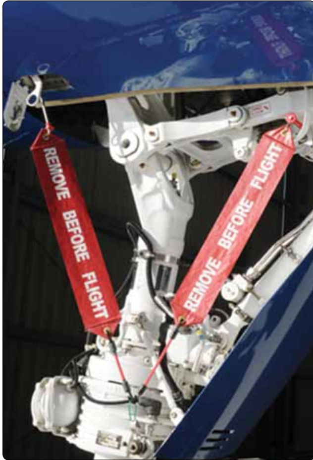
Figure 13-42. Gear pin ground lock devices.
