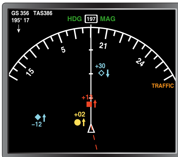
Figure 11-133. TCAS information displayed on a multifunction display. An open diamond indicates a target; a solid diamond represents a target that is within 6 nautical miles of 1,2000 feet vertically. A yellow circle represents a target that generates a TA (25-48 seconds before contact). A red square indicates a target that generates an RA in TCAS II (contact within 35 seconds). A (+) indicates the target aircraft is above and a (-) indicates it is below. The arrows show if the target is climbing or descending.
