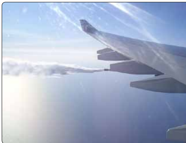
Figure 14-5. Fuel being jettisoned free of the airframe on a transport category aircraft.
