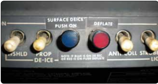
Figure 15-19. Wing deice switch.
