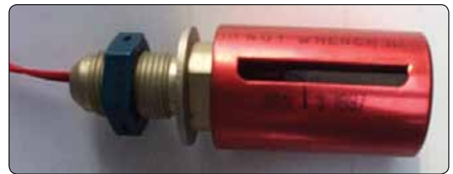
Figure 14-104. A float switch installed in a fuel tank can close the refueling valve when the tanks are full during pressure fueling of an aircraft. Other more sophisticated automatic shutoff systems exist.
