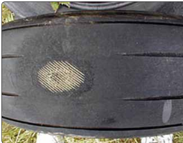
Figure 13-140. Landing with the brake on causes a tire flat spot that exposes the under tread and requires replacement of the tire.
