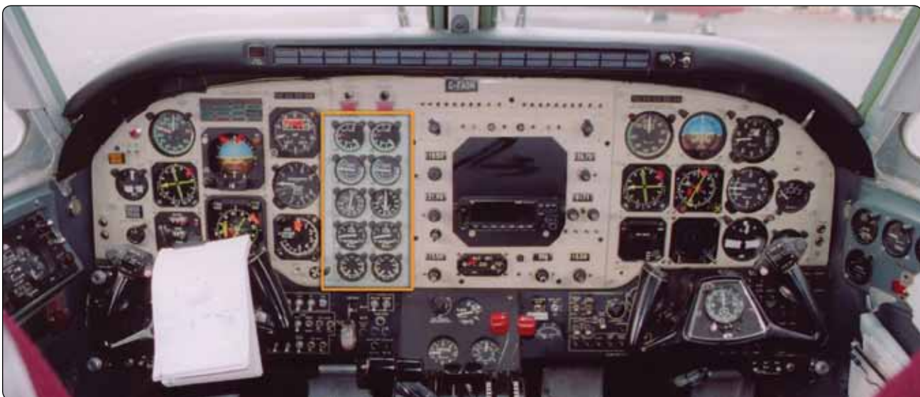
Figure 10-7. An engine instrumentation located in the middle of the instrument panel is shared by the pilot and co-pilot.
