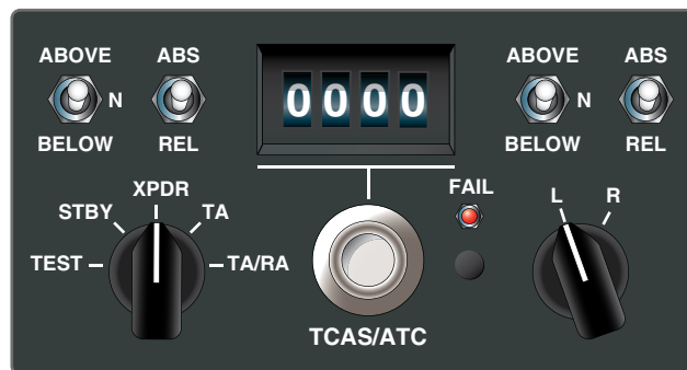
Figure 11-134. This control panel from a Boeing 767 controls the transponder for ATC use and TCAS.
