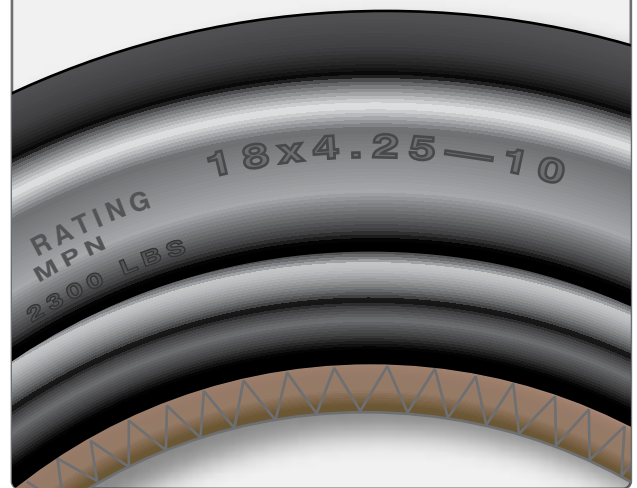
Figure 13-127. A Type VIII or three-part nomenclature tire is identified by 3 parameters: overall diameter, section width, and rim diameter. They are arranged in that order with the first two separated by an "X" and the second two separated by a "-." For example: 18 X 4.25—10 designates a tire that is 18 inches in diameter with a 4.25-inch section width to be mounted on a 10-inch wheel rim.
