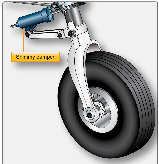
Figure 13-21. A shimmy damper helps control oscillations of the nose gear.
