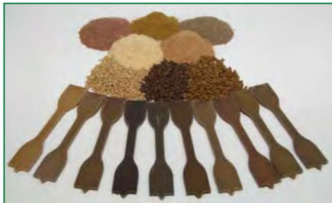
Wood properties influence the color and other characteristics of wood-plastic composites.
