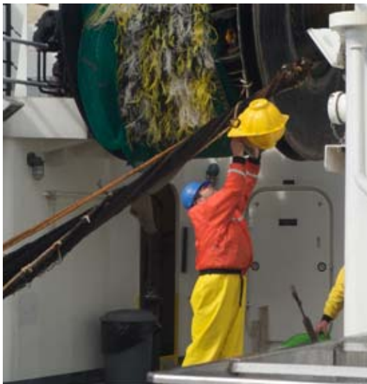
This is one of the glass floats encased in plastic that can withstand the pressure of the deep waters.
