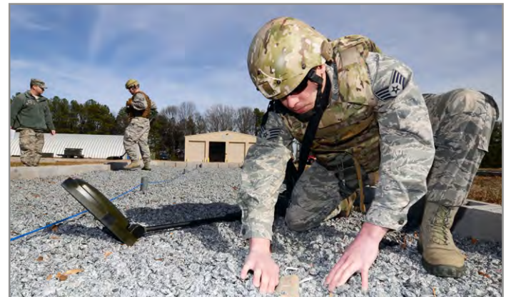
Reservists from the 94th Civil Engineer Squadron, Explosive Ordnance Disposal Flight, train with the Minehound VMR2 Ground Penetrating Radar (GPR) metal detector during an exercise at the Air Force Reserve Command Expeditionary Combat Support Training Certification Center here, Jan. 24. (photo by Don Peek)
