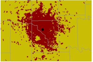
This will occur only with weather returns that are sufficiently strong to dominate the ground returns. For example, you will not see this effect with stratiform precipitation.
