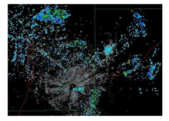
RDA Build 11.1 significantly improved the problem of isolated missed detections within mountainous areas. This change **only** affects the areal coverage of ground clutter identified by CMD. It does **not** change the amount of suppression applied by GMAP. It also does not change CMD's relationship with moving clutter. For example, CMD will **not** detect traffic on roads or returns from wind turbines.
