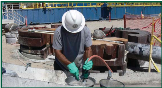
Collecting groundwater samples from Well ER-20-4
