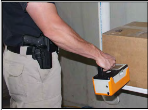
Using a RIID to determine if material is illicit
