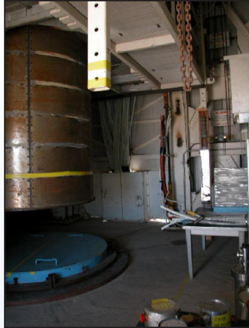
Left: The bottom portion of the Ice Box that would have been used to provide cooling by way of dry ice and circulation fans for the area immediately around the nuclear device.
