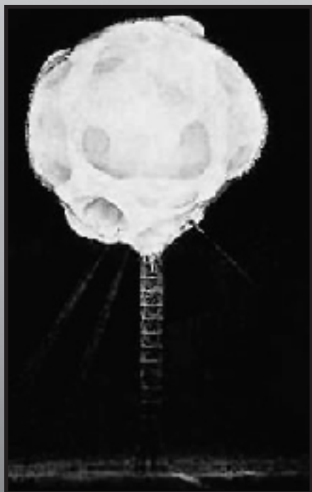
A rapatronic photo captures a tower test during Tumbler-Snapper immediately after detonation, but before the "rope trick" is visible.
