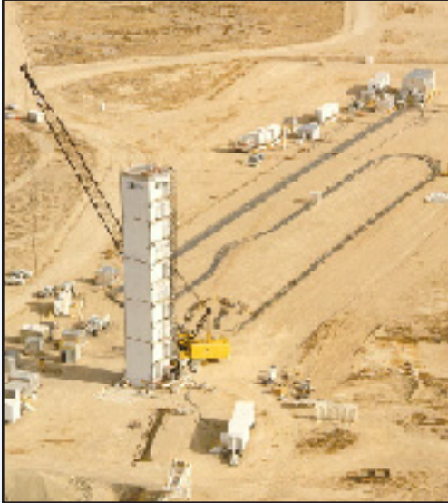
An aerial view of the emplacement tower, diagnostic cables and diagnostic trailers used during an underground nuclear test.
