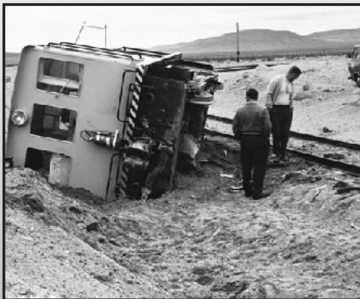
The derailed locomotive lies 180 degrees from its direction of travel as investigators inspect the site.
