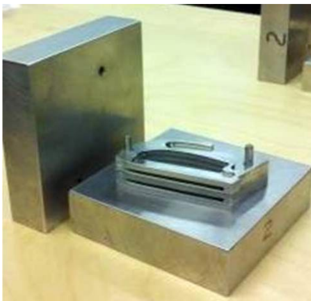
FIGURE 4. Spar-Shell™ vane insert manufacturing trial
