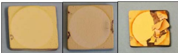
FIGURE 6. APS TBC coated coupons after laser flux testing. Left photo: René N5/A1D/APS YSZ/ZrO312; air at ~1,482°C, 50 1-hr cycles (Test 1–3). Middle photo: René N5/LPPS MCrAlY/APS YSZ/ZrO312; air at ~1,482°C, 50 1-hr cycles (Test 1–4). Right photo: René N5/A1D/APS YSZ/ZrO312; steam at ~1,482°C, 49 1-hr cycles (Test 1–5).
