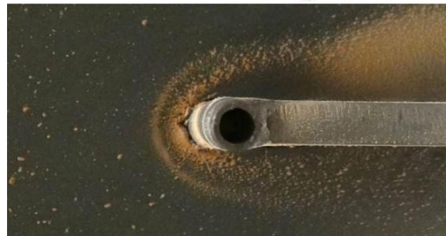
FIGURE 4. Deposition model predictions of endwall deposition pattern compared with experimental validation of same
