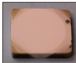
Test No. 2-5: Coupon tested in steam at 1450-1460 C for 50 1 hr cycles
