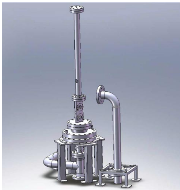
FIGURE 4. Overall integration of the test section and approach flow module with existing high pressure test facility infrastructure
