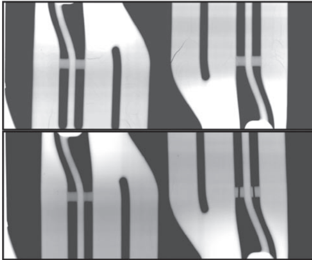
FIGURE 3. Original process cores (top) - show cracks and internal defect lines versus improved process cores (bottom) – internal surfaces show a significant improvement
