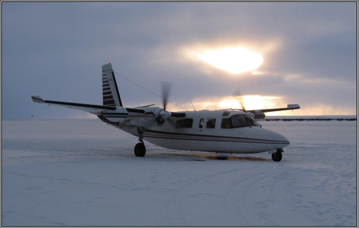
Figure 2. COMIDA 2010 survey aircraft, Turbo Aero Commander 690A, call sign N222ME, chartered from Northern Commanders, Spokane, Washington. Photo by Janet Clarke (SAIC).
