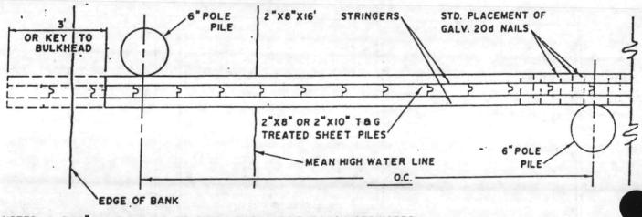
NOTES: I. 7/16" DIA. GALV. BOLTS SHALL BE PLACED THROUGH STRINGERS AND SHEET PILES AT EACH BUTT JOINT AND AT EACH POLE PILE. BOLTS SHALL NOT BE PLACED MORE THAN 8 FEET APART.
