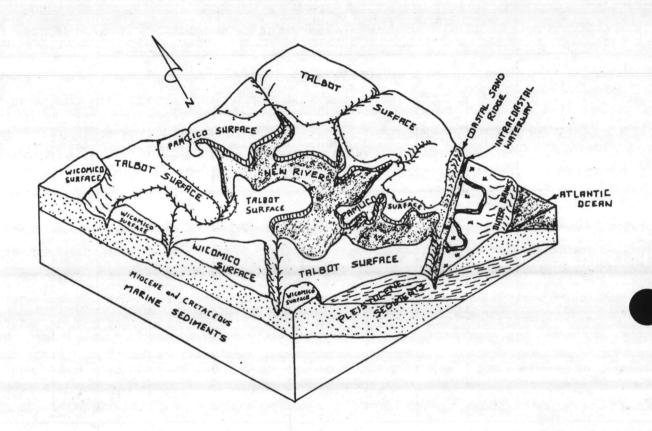
FIGURE 3: Elevations of geomorphic surfaces of the Camp Lejeune area: Pamlico 0-25 feet, Talbot 25-45 feet, Wicomoco 45-70 feet.
