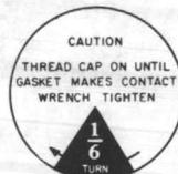
3. Unit is shipped with valve stem(s) frontseated, and caps installed. Replace stem caps after system is opened to refrigerant flow (backseated). Replace caps finger tight and tighten additional 1/6 turn with wrench. See sticker on valve cap.
