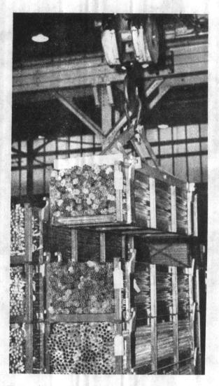
Figure 5-69. Crane positioning rack into storage.
