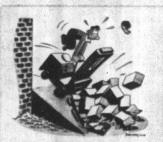
Don't descend ramps with load in front ... drive down backwards at slow speed.
