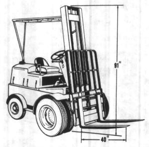
Figure 4-8. Truck, forklift, pneumatic tires, 4,000-pound, 144-inch lift.
