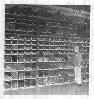
Figure 5-66. Storage of materials in pigeonhole type racks.
