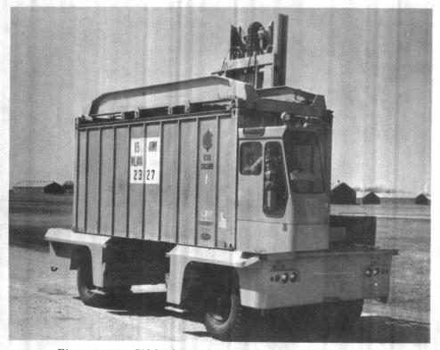
$Figure \ 3\text{--}135. \quad Side loader \ truck \ equipped \ with \ top lift \ attachment.$
