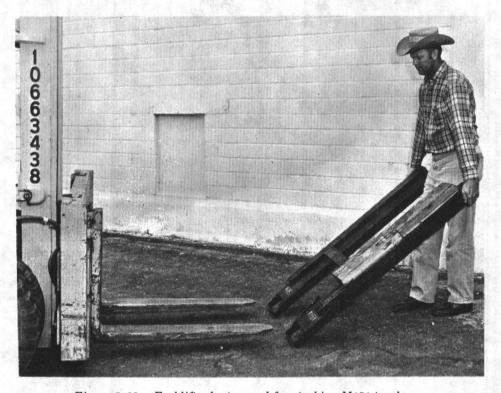
Figure 5-28. Forklift adapter used for stacking M151 trucks.
