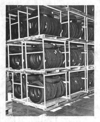
Figure 4-53. Support sets used for tire storage.
