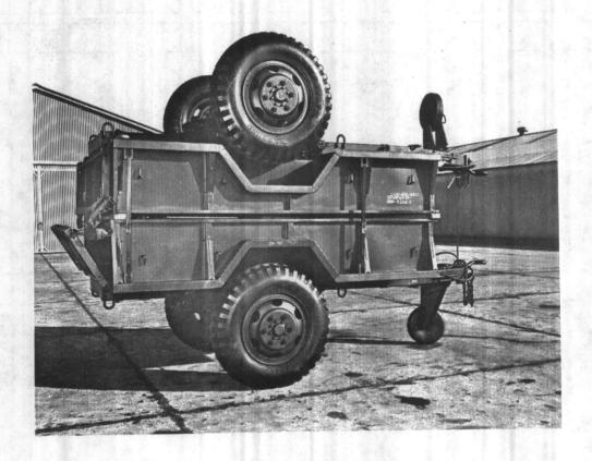
Figure 5-20. Inverted trailers ready for storage.
