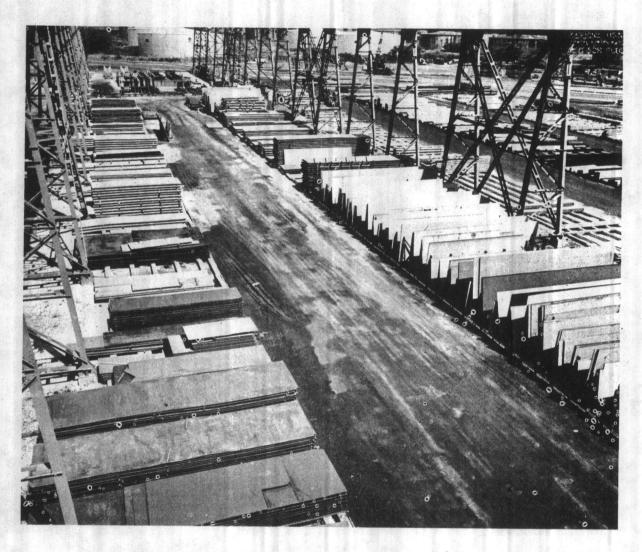
Figure 5-61. Storage of heavy plate and structural shapes.
