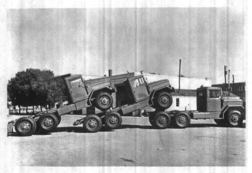
Figure 5-35. Truck tractors piggybacked for driveaway shipment.
