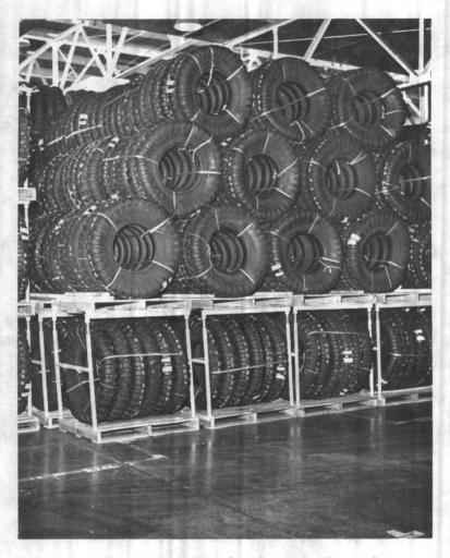
Figure 5-54. Tires stacked atop a base layer of pallets and support sets. Note the 6-inch extension on the support set uprights.
