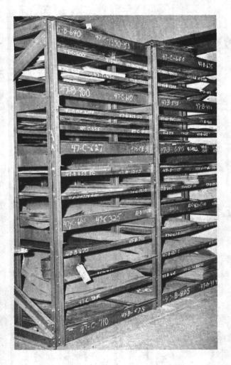
Figure 5-60. Lightweight sheet or strip racks.
