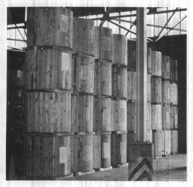
Figure 5-80. Small cable reels properly dunnaged for safe efficient stacking.
