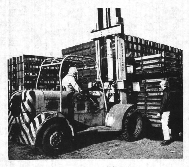
Figure 5-70. Fork truck operation in open storage.
