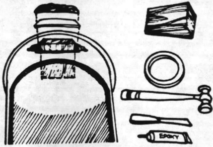
Sequential Wedge Plugging Steps
