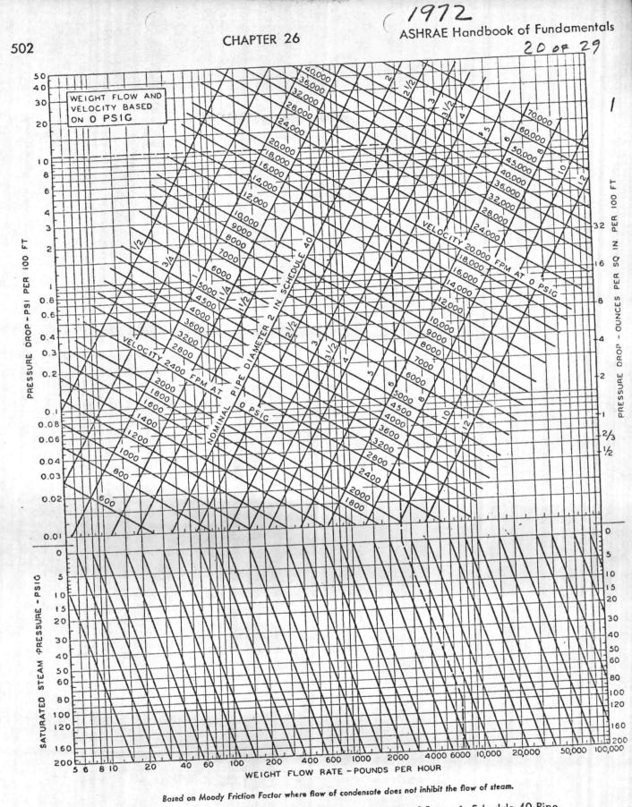
Fig. 5 .... Basic Chart for Weight-Flow Rate and Velocity of Steam in Schedule 40 Pipe Based on Saturation Pressure of 0 Psig
