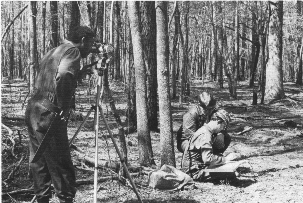
COLLECTING DATA FOR 3-P FOREST INVENTORY. THE DENDROMETER PROVIDES EXACT TREE MEASUREMENTS.
