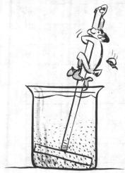
8. Stop the stirring apparatus and allow samples in beakers to settle for 30 minutes. 16 Observe the floc settling characteristics. A hazy sample indicates poor coagulation. Properly coagulated water contains floc particles that are well-formed and dense, with the liquid between the particles clear. Describe results as poor, fair, good, or excellent.
