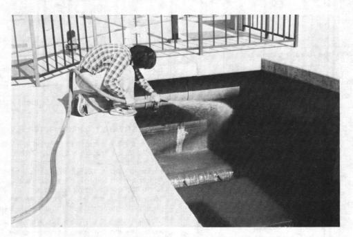
Operator hosing down filter sidewalls during backwash (NOTE: Operator is too close to edge and could fall in — should be behind guardrails)
