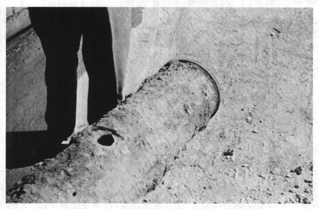
Corrosion at corporation stop hole caused by joining two dissimilar metals
