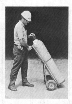
Fig. 7.18 Hand truck for chlorine cylinder (Courtesy of PPG Industries)
