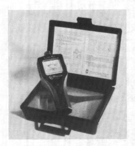
Portable Chlorine Leak Detector (Permission of Leak-Tec Division American Gas & Chemical Co., Ltd.)
