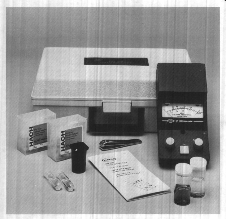
Fig. 7.34 Direct reading colorimeter for free chlorine residuals (Permission of the Hach Company)
