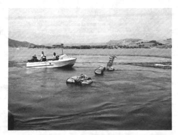
Fig. 3.12 Reaeration-destratification system in operation
