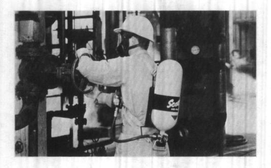
Fig. 7.25 Self-contained breathing apparatus (Courtesy of PPG Industries)
