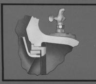
OPTIONAL IMPELLER WEARING RINGS Can be mounted on impeller without additional machining of impeller. Locked on impeller hub with stainless steel set screws.
