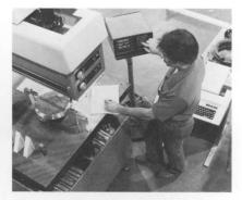
Value components are computer quality-checked and tested on coordinate measuring devices to ensure consistent high quality.
