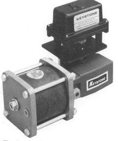
The limit switch has two SPDT camoperated switches which are adjustable throughout the 90° travel range. The limit switch meets NEMA 4 or NEMA 7 design requirements and is rated at 10A for 120V/240V service. The limit switch can be mounted directly on air-to-air or springreturn models.
