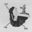
impeller with impeller wearing ring
