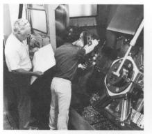
All valves are machined on precision Computer Numerical Controlled (CNC) equipment.
