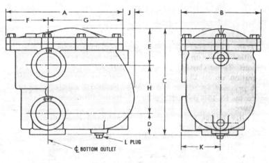
FIGURE 2 – Models 66C, 77H, 88J, 200C, and 200H Float-Thermostatic Trap Dimensions – All Pressure Classes .
