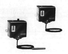
Operate electric dampers, valves, and compressor or fan motors to provide temperature or limit control of air conditioning systems and refrigeration units. Models with 20 ft (6 m) capillary operates from the coldest one foot long section making it ideal for coil freeze-up protection. L480B also used as frost alarm. UL Listed.
