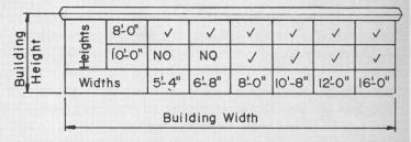
Building Lengths-Any Multiple Of 16" Increments (Minimum Length Is Equal To Building Width)
