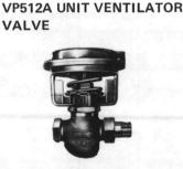
Normally-open, single seated, straightthrough or angle globe valve for proportional control of either steam or hot water in unit ventilators. Bronze body in 1/2 to 1-1/4 NPT sizes. Nominal Body Rating: 150 psi (1034 kPa). Molded neoprene diaphragm operator. Control Air Pressure: 25 psi (172 kPa). Operating Range: 3 to 8 or 6 to 11 psi (21 to 55 or 41 to 76 kPa), factory set, with Cv Ratings from .63 to 16. Ambient Temperature Limit: 160 F (71 C).
