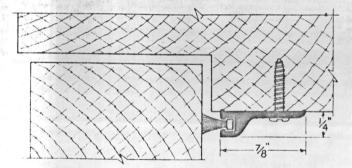
309AW EXTRUDED ALUMINUM AND WOOL PILE (Wool pile works well
