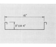
Roof panels shall be 16" wide with a smooth surface between the interlocking side ribs. The interlocking ribs shall be a minimum 3" high, and shall be turned upward. All roof panels shall be factory punched for connection at the eave line of the building.
