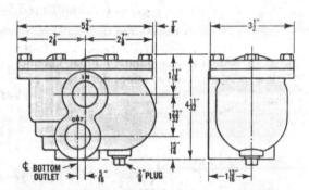
FIGURE 1 — Model 55A Float-Thermostatic Trap Dimensions For All Pressure Classifications.
