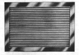
Offers maximum free area. Completely sight proof. Widely used for exhaust and return air grilles where concealment of duct desirable. Ruggedly constructed of closely spaced v-shaped louvers parallel to long dimension, rigidly mounted in a flange type frame. Rattle-free, even if door is slammed.
