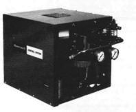
Condition air supply systems for pneumatic controls by cooling control air and condensing and removing oil, water vapor and other contaminants from the system. Designed to dehydrate to a 35 to 39 F (2 to 4 C) dew point at normal operating tank pressures.
