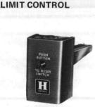
Safety device which breaks line-voltage contacts as air temperature reaches predetermined cut-out level where fire protection is needed.
