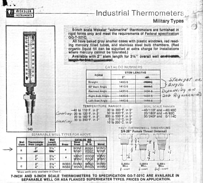
WHEN ORDERING: Specify (1) Thermometer Catalog No. (2) Range; (3) if required, specify separable well Catalog No. from table above.
