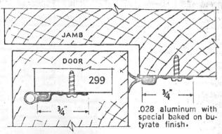
304A ALUM. and VINYL FINGERS, aluminum color. 304G ALUM. and VINYL FINGERS, gold color. 304D ALUM. and VINYL FINGERS, duranodic color. 299A ALUM. and VINYL BULB, aluminum color. 299G ALUM. and VINYL BULB, gold color. 299D ALUM. and VINYL BULB, duranodic color. Stock sets = 36 x 80 (and 84), 72 x 80 (and 84).
