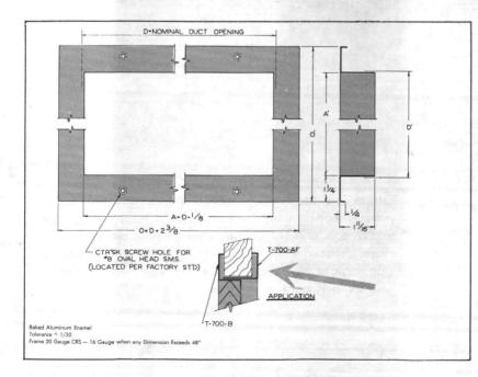
The T-700 B Auxiliary Frame is available for use with the T-700 B Door Grille. Frame telescopes over door grille. Adjusts grille to fit any door thickness from 1%" to  $2\frac{1}{2}$ " and gives a finished appearance to installation.
