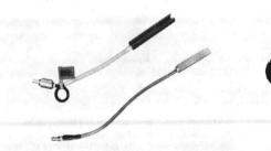
Direct-acting, proportional type sensors used with RP908 Controller to control pneumatic valves and damper operators. May be used with calibrated gage for continuous temperature indication. Sensing Range: Nonadjustable, 50 to 100 F (10 to 38 C). When used with the SSP129A DewProbe, senses 103 to 153 F (40 to 68 C) cavity temperature range. Dewpoint temperature range is 40 to 75 F (4 to 24 C).
