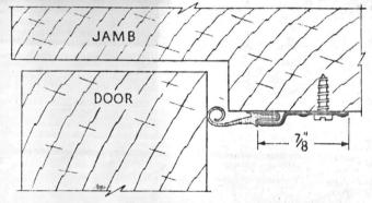
399AV PAINTED ALUMINUM (alum. color) Specially designed vinyl compensates for variations in gap around wood door.
