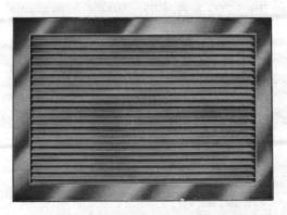
Offers maximum free area. Are completely sightproof. Widely used for exhaust and return air grilles where concealment of duct desirable. Constructed of closely spaced v-shaped louvers parallel to long dimension, rigidly mounted in a channel type frame. Rattlefree even if door is slammed.
