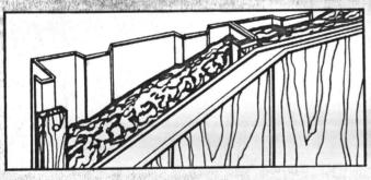
MARK I — For an easy-to-install, economical wall system where condensation control and a hard-surface interior are not critical requirements, Parkline's Mark I wall is the quality solution. Semirigid fiberglass, 1½ inches thick, faced with a white embossed vinyl is retained in place between the panel ribs with a white PVC rib retainer. U. value is 0.20; R value is 4.9.
