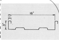
Wall panels shall be 16" wide with a 3" deep inward turned interlocking side rib. Wall panels shall contain two 11/16" deep by 3-1/8" wide fluted recesses, each starting 2-7/16" from the panel edge.
