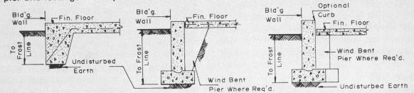
Wire mesh reinforcing is recommended in the floor slab under any condition. Additional reinforcing such as rods, may be required to satisfy strength requirements and to prevent cracks due to uneven settlement of soil.
