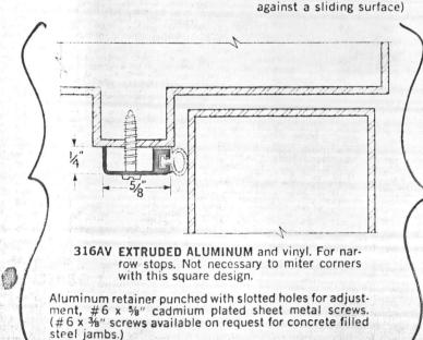
Extruded aluminum strips available in gold anodized or duranodic finish on special order.
