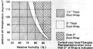
11/2" Thick Duct Wrap 2" Thick Duct Wrap Over 2" Duct Wrap
