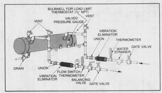
FIGURE 15 - Evaporator Water Piping Components.
