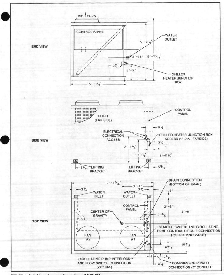
FIGURE 4 - Unit Dimensions and Connections. CGAB C20.
