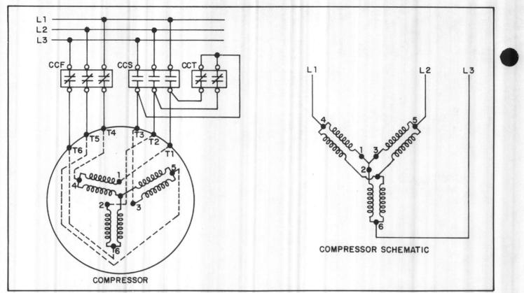
Figure 3 - High Speed Operation (Parallel Connected)
