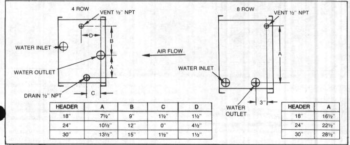
FIGURE 37 - Coll Type P8 Connections with Drain and Vent Locations (18", 24", and 30" Headers)
