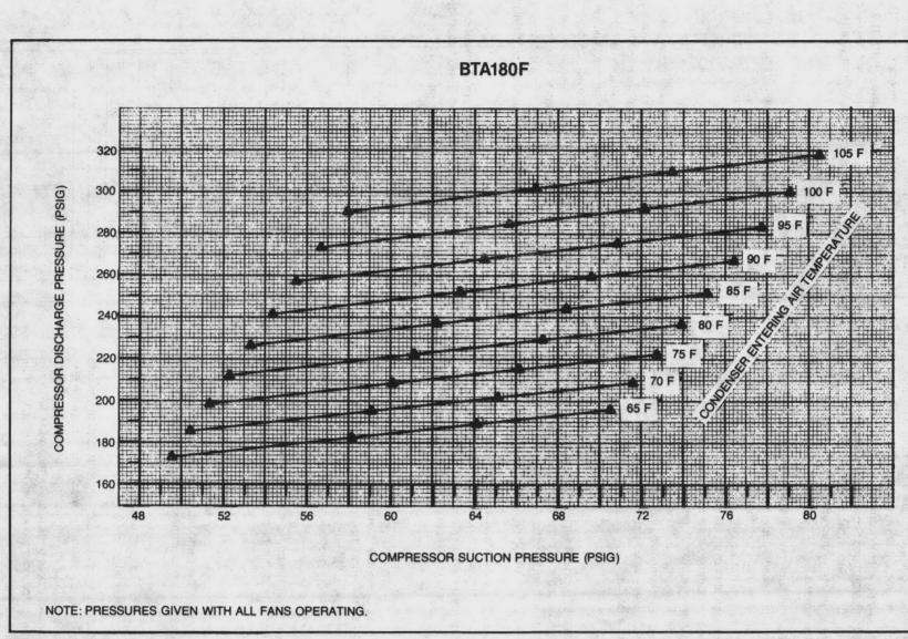
Figure 13 - BTA180F Operating Pressures
