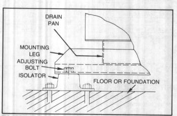
FIGURE 3 - Anchoring the Unit
