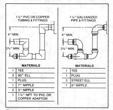
Figure 6 — Details of Two Typical Condensate Drain Line Trap Assemblies
