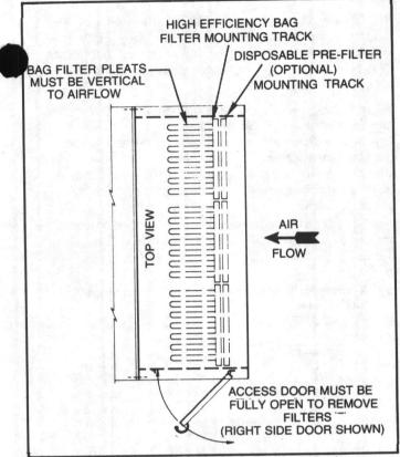
FIGURE 21 - Filter Mounting Track Location (Top View)
