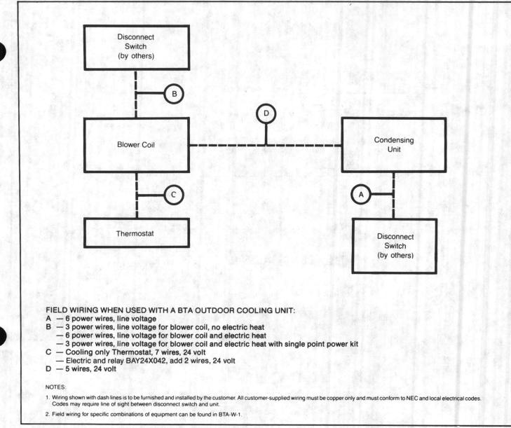
Figure 7 — Typical Electrical Connections by Customer for a BTA180,240C with a BWV/BWH180,240B
