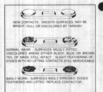
Figure 6 - Compressor Contactor Replacement Guide
