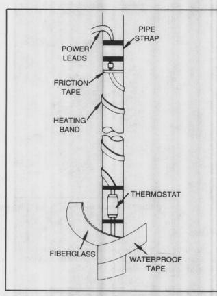
FIGURE 16 - Installing Chilled Water Piping Heater Cable.
