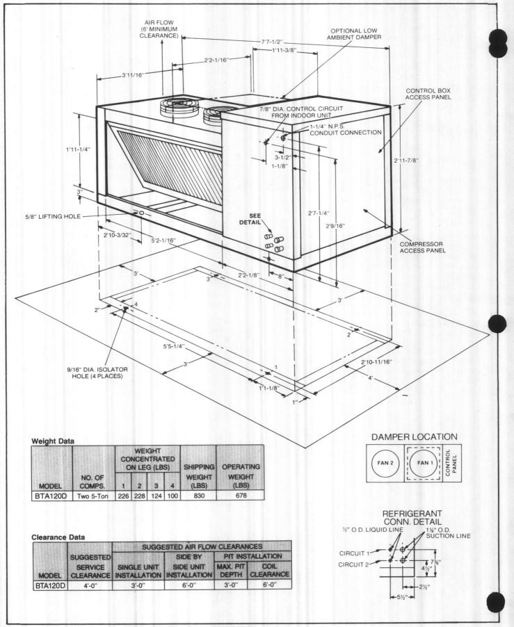
Figure 1 - Dimensions, Weights, and Clearances for BTA120D Units
