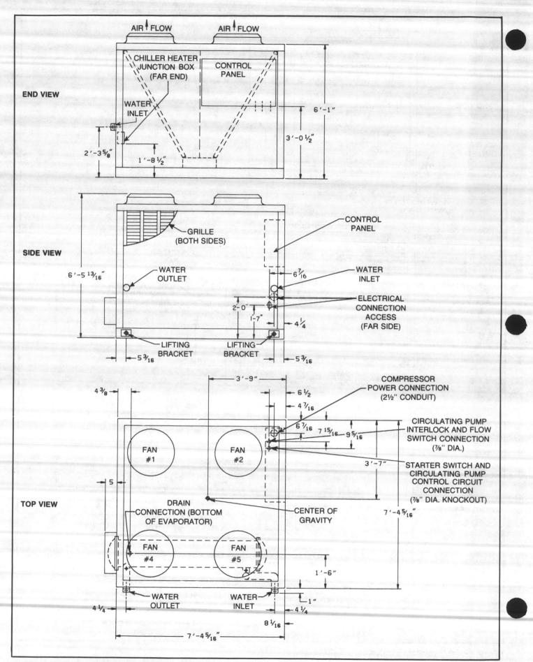
FIGURE 7 - Unit Dimensions and Connections. CGAB C40.
