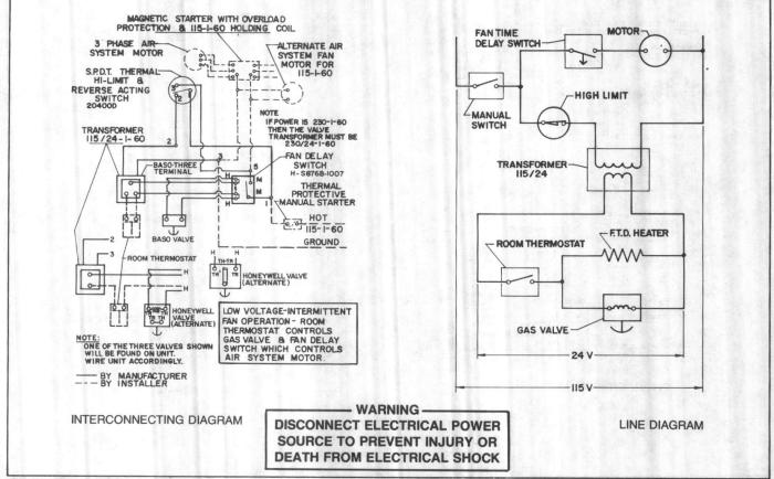
FIGURE 10 - Duct Furnace Wiring Diagram, Single Stage Standing Pilot With Fan Time Delay Relay
