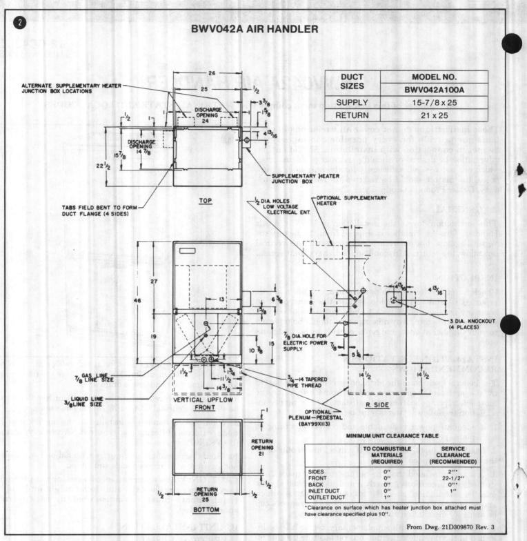
c. If a return duct is connected to the air handler, it must be the same dimensions as shown in outline drawing (see Figure 2).
