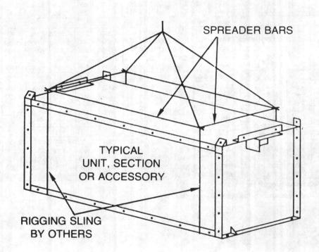
FIGURE 1 - Recommended Rigging Procedure
