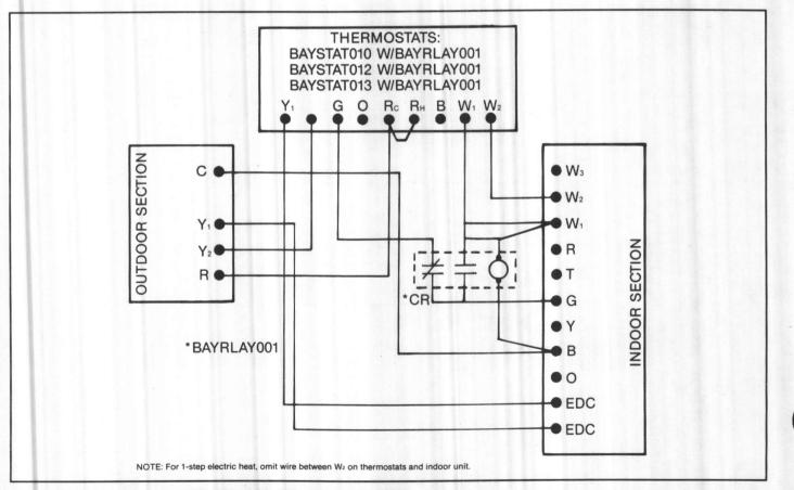
Figure 16 - Field Wiring for BTA120D With BTE120B Air Handler BTA-IN-5 18
