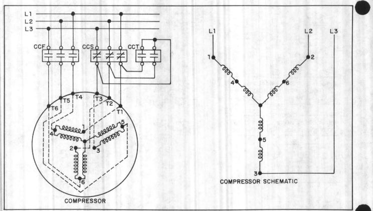
Figure 4 - Low Speed Operation (Series Connected)
