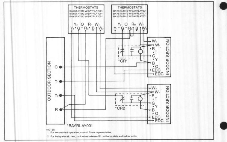
Figure 12 - Field Wiring for BTA150D and BTA180D With Two (2) BWE090C Air Handlers
