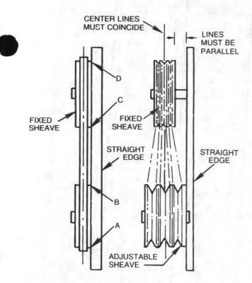
Figure 53 - Sheave Alignment
