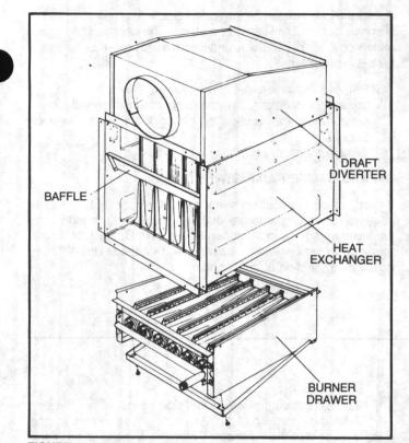
**FIGURE 12 - Duct Furnace Components**
