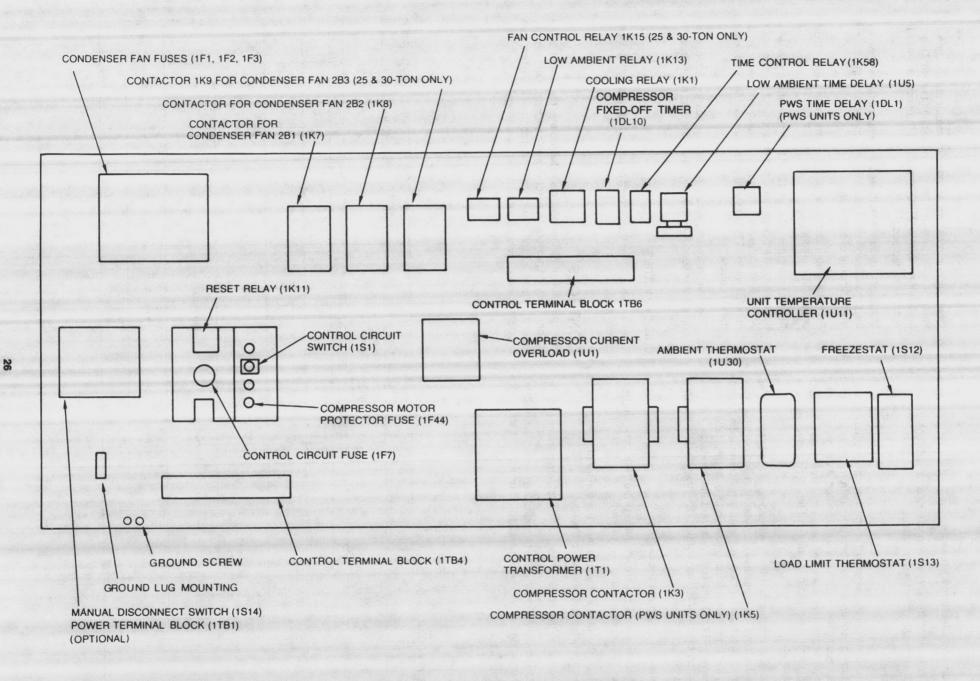
FIGURE 20 - Typical Control Panel Layout. CGAB C20, C25 and C30.
