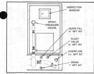
FIGURE 33A - Sprayed Coil Unit Tank Connections
