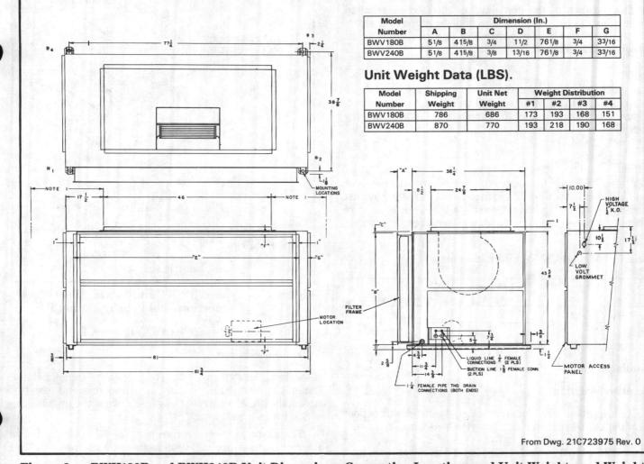
Figure 2 — BWH180B and BWH240B Unit Dimensions, Connection Locations and Unit Weights and Weight Distribution.
