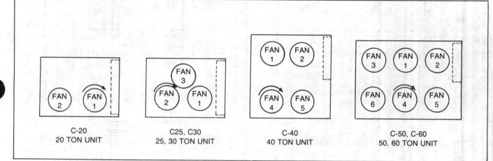
FIGURE 23 - CGAB Condenser Fan Locations.
