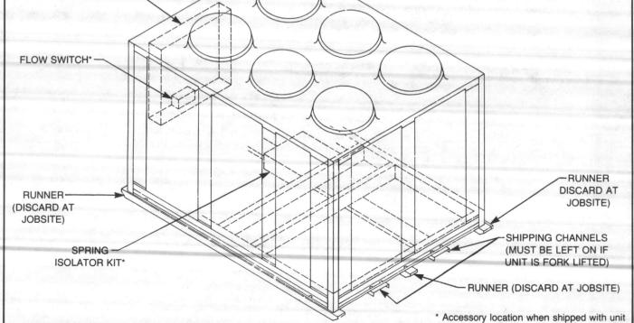
FIGURE 3 - Shipping Package. CGAB C50 and C60.
