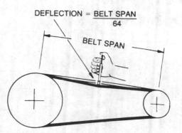
Figure 55 - Belt Tension Measurement
