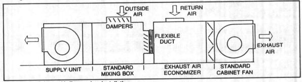
FIGURE 22 - Exhaust Air Economizer Installation
