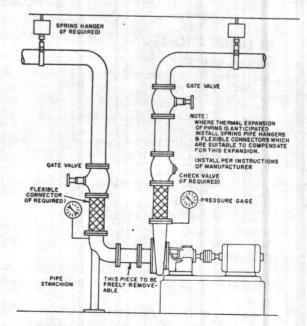
Fig. 3-Typical Installation-Vertical Piping
