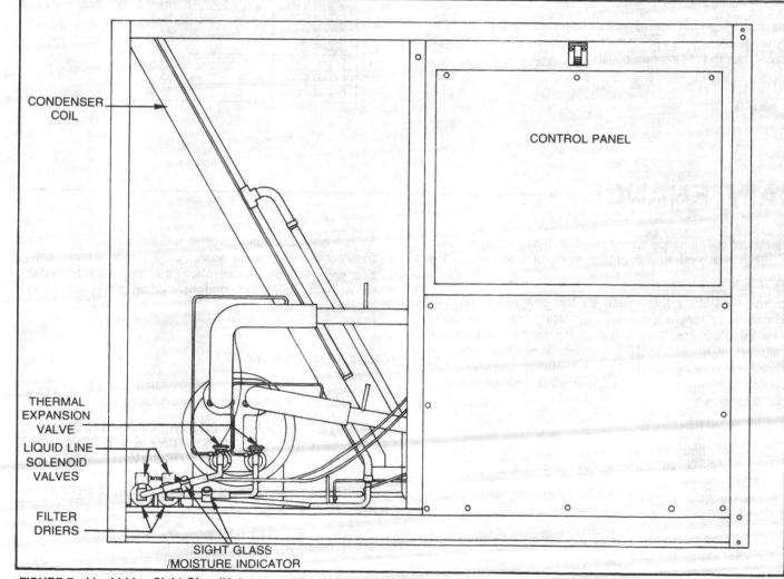
FIGURE 7 - Liquid Line Sight Glass/Moisture Indicator Locations (CGAB-C60 Shown)
