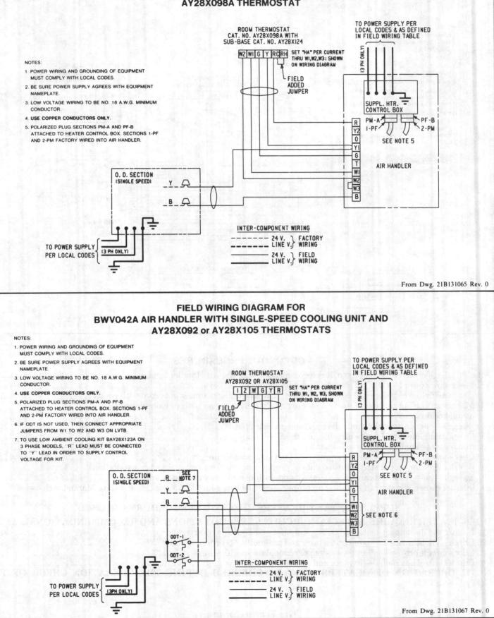
FIELD WIRING DIAGRAM FOR **BWV042A AIR HANDLER WITH WEATHERTRON® HEAT PUMP**
