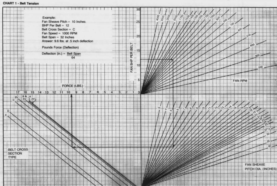
For belt cross-section types not given in Chart 1, refer to Table 6 and use the following equations to calculate correct belt tension:
