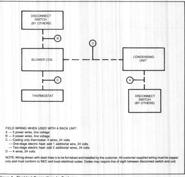
Figure 8 - Electrical Connections by Customer
