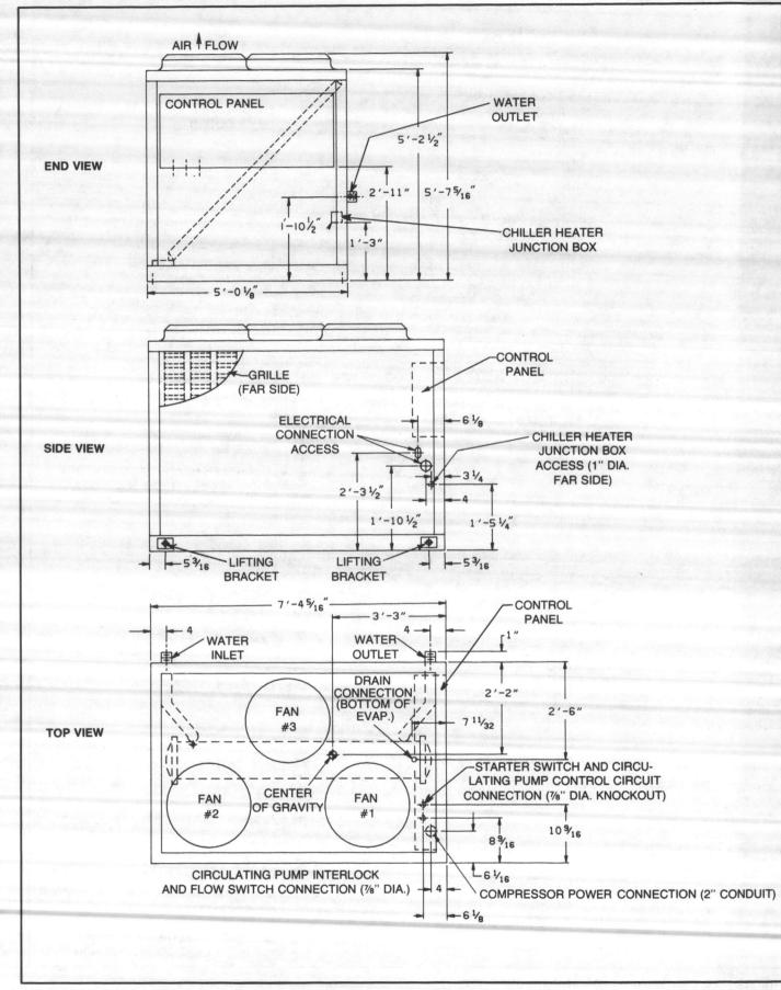
FIGURE 5 - Unit Dimensions and Connections. CGAB C25.
