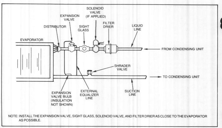
Figure 7 - Diagram of Refrigerant Piping Components in Liquid Line
