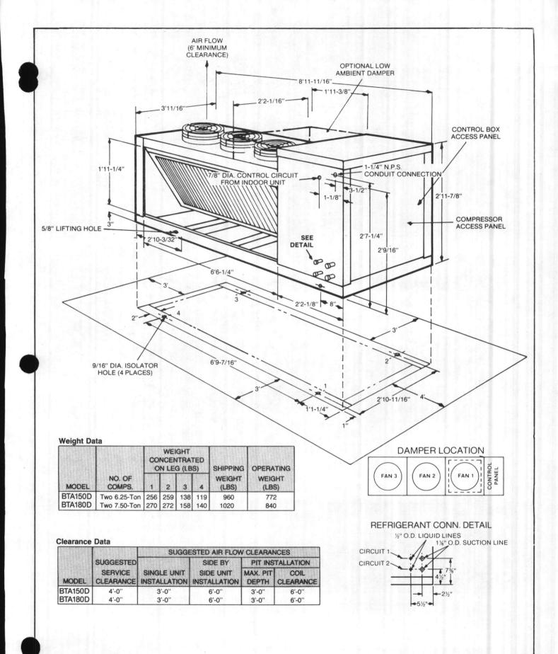
Figure 2 - Dimensions, Weights, and Clearances for BTA150D and 180D Units
