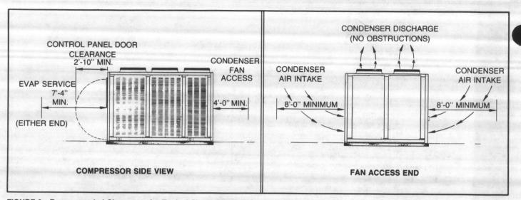
FIGURE 9 - Recommended Clearances for Typical Single CGAB C60 Installation.
