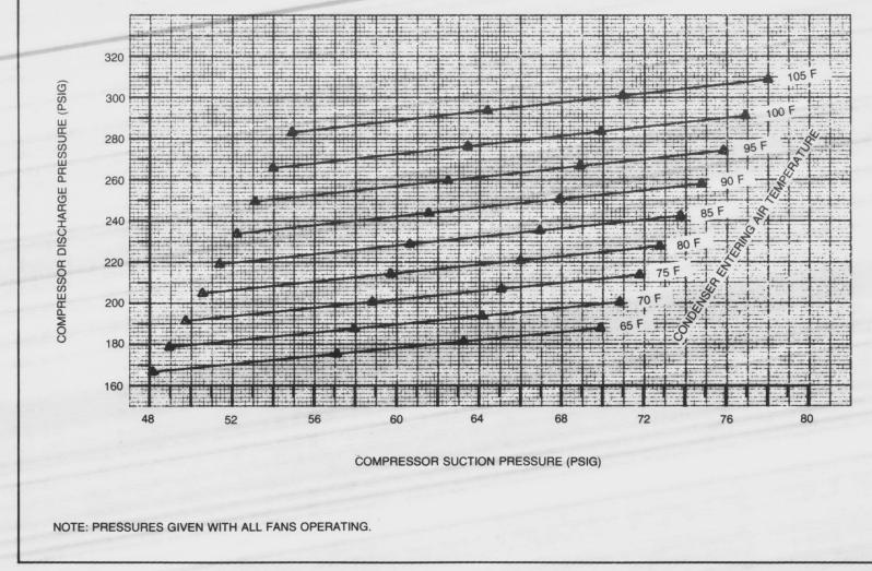
Figure 10 · BTA120D Operating Pressures
