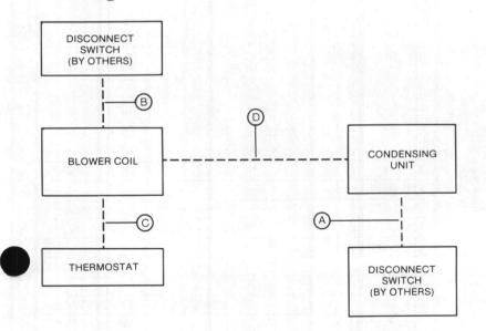
Field Wiring when used with a BTA Outdoor Cooling Unit:
