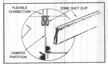
FIGURE 30 - Zone Duct Clip Installation
