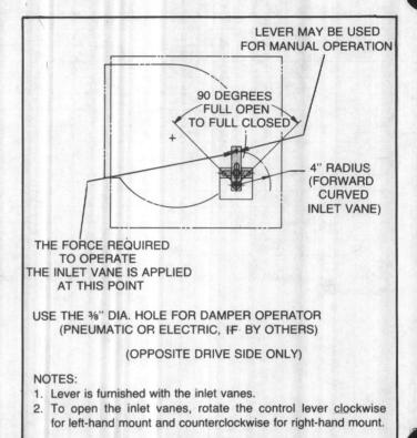
FIGURE 25 - Inlet Vane Operation
