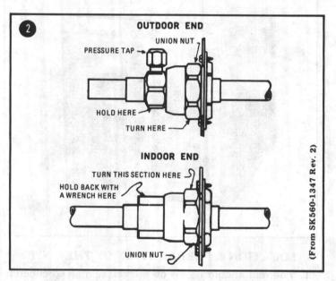
Additional tire-valve type pressure taps are provided on the cabinet of outdoor unit for access to the compressor suction and discharge.
