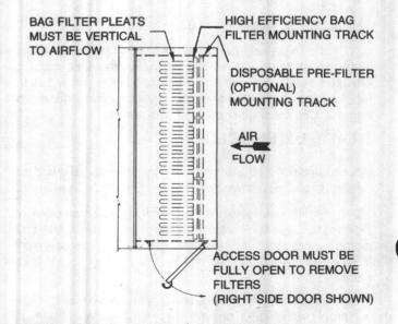
FIGURE 1 - Filter Mounting Track Location (Top View)
