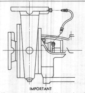
Before filling system with water, assemble external circulation tube to pump casing as follows:
