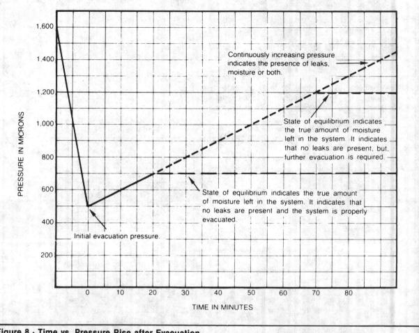
Figure 8 · Time vs. Pressure Rise after Evacuation
