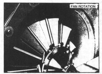
FIGURE 27 - Airfoil Inlet Vanes
