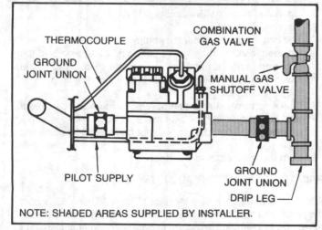
FIGURE 7 - Pipe Installation, Standard Controls
