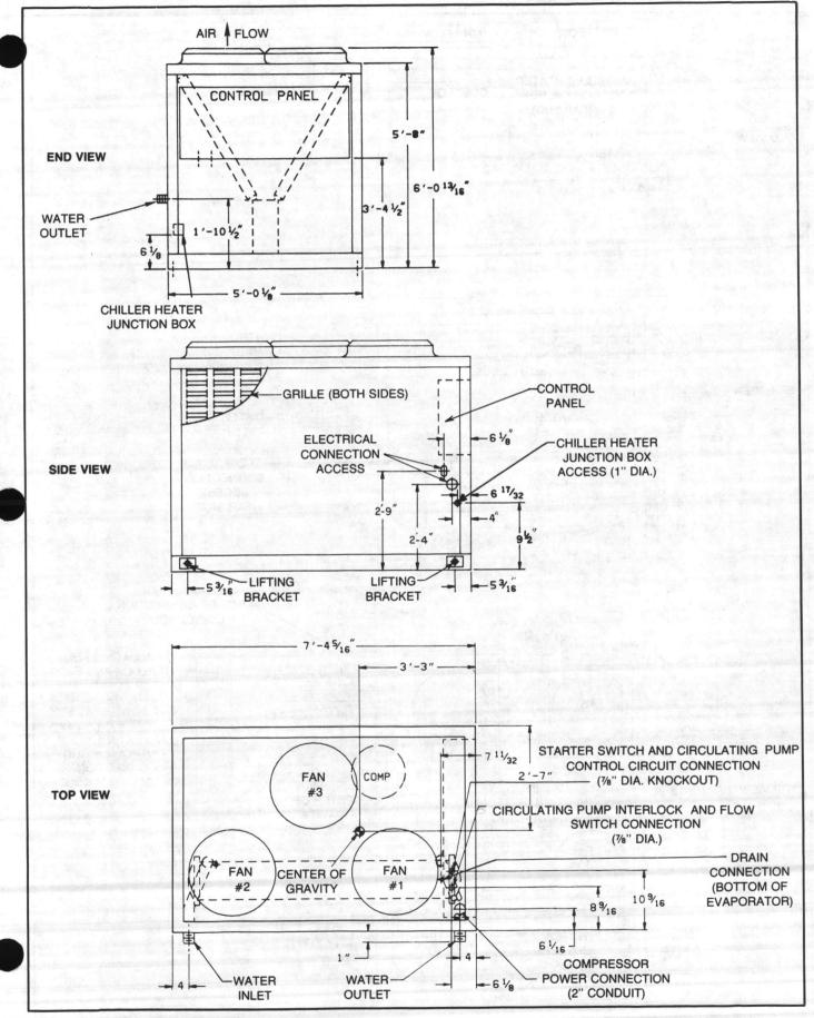
FIGURE 6 - Unit Dimensions and Connections. CGAB C30.
