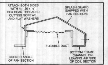
FIGURE 8 - Splash Guard Installation
