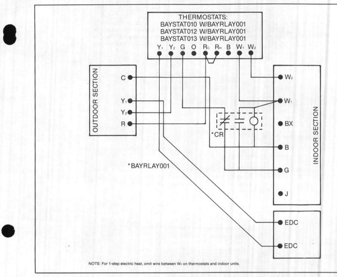
Figure 17 - Field Wiring for BTA150D, BTA180D and BTA180F With the BWV180B, BWH180F Air Handlers
