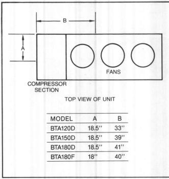
Figure 5 - Unit Center of Gravity Information
