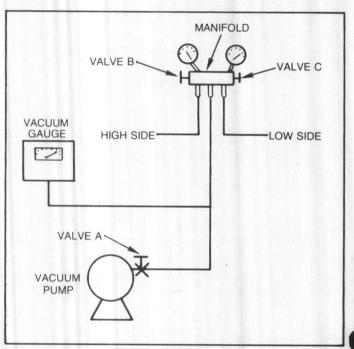
Figure 7 · Vacuum Pump Hook-Up
