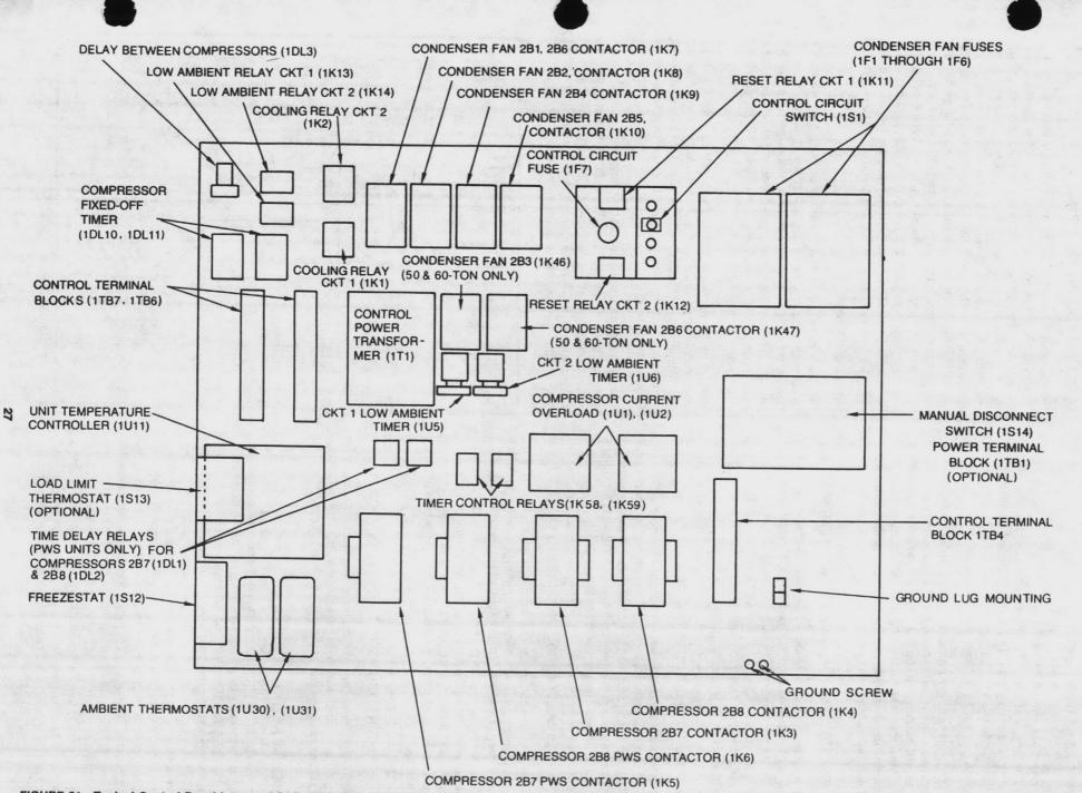
FIGURE 21 - Typical Control Panel Layout. CGAB C40, C50 and C60.
