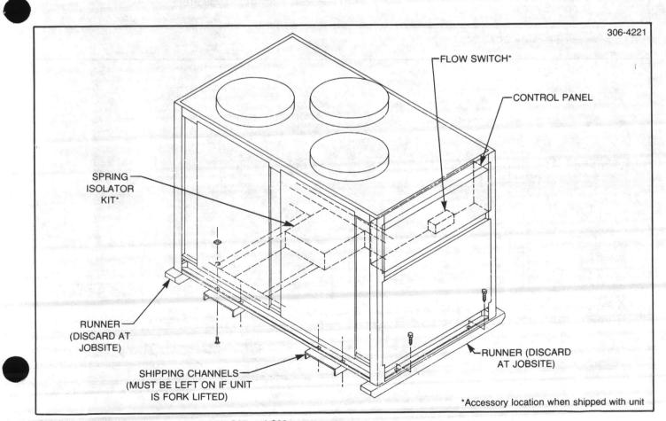
FIGURE 1 - Shipping Package. CGAB C20, C25 and C30.
