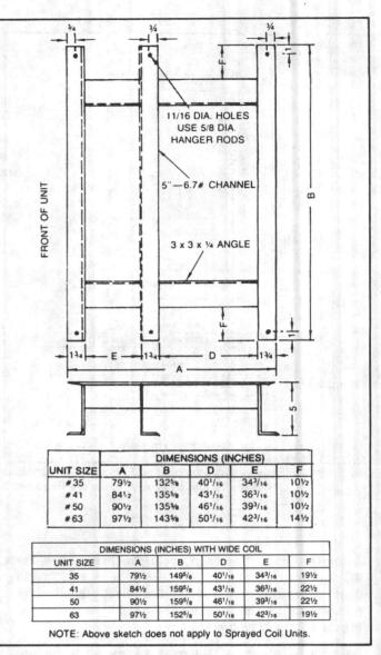
FIGURE 12 - Ceiling Suspension Mounting Frame and Dimensions for Unit Sizes 35 to 63
