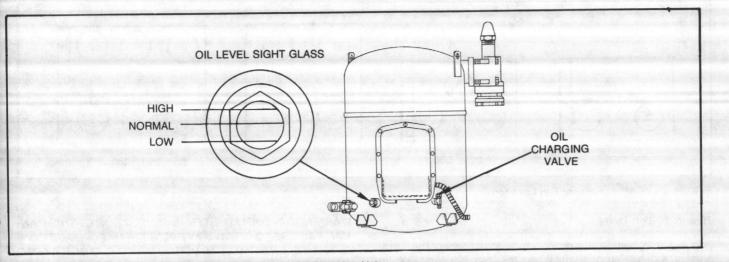
FIGURE 5 - Model K Compressor Oil Level Sight Glass, Oil Charging Valve
