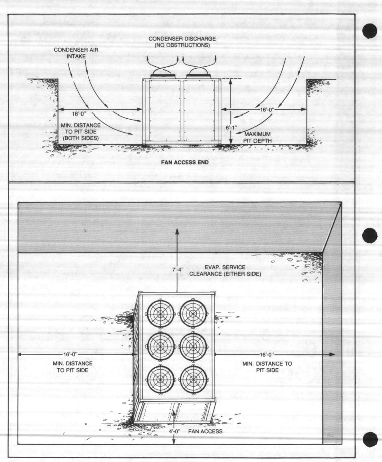
FIGURE 11 - Recommended Clearances for Typical CGAB C60 Pit Installation.
