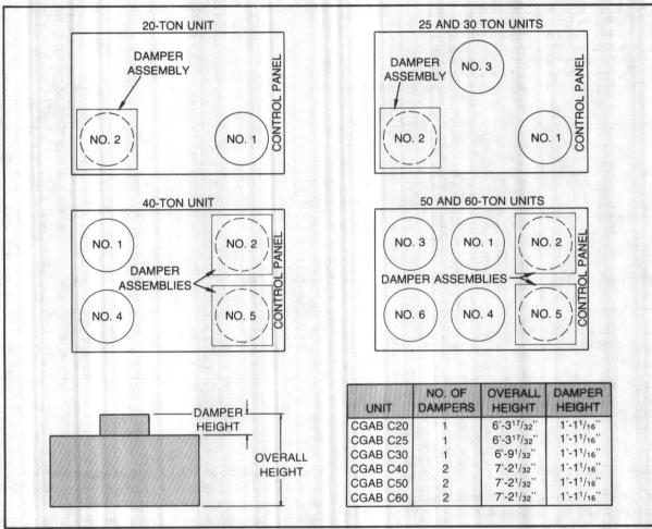
FIGURE 24 - CGAB Low Ambient Dampers.
