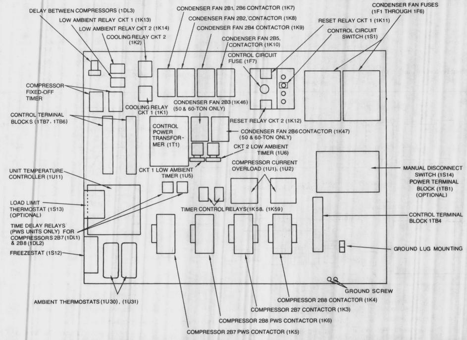
FIGURE 3 — Control Panel Layout for CGAB-C40, C50 and C60
