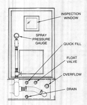
FIGURE 12 - Sprayed Coil Unit Tank Connections
