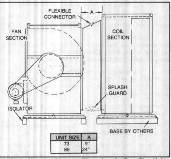
FIGURE 7 - Mounting Clearance Dimensions for Draw-Thru Units Sizes 73-86
