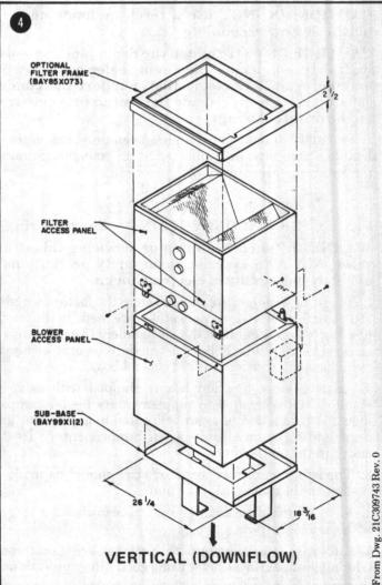
It is recommended that a 1/2'' flange be provided on the duct. After the duct is installed, tab location is shown by dimples on unit discharge. Position duct and match-drill to tabs to assure proper engagement of sheet metal screws. After duct is secured, seal around discharge to prevent air leakage.
