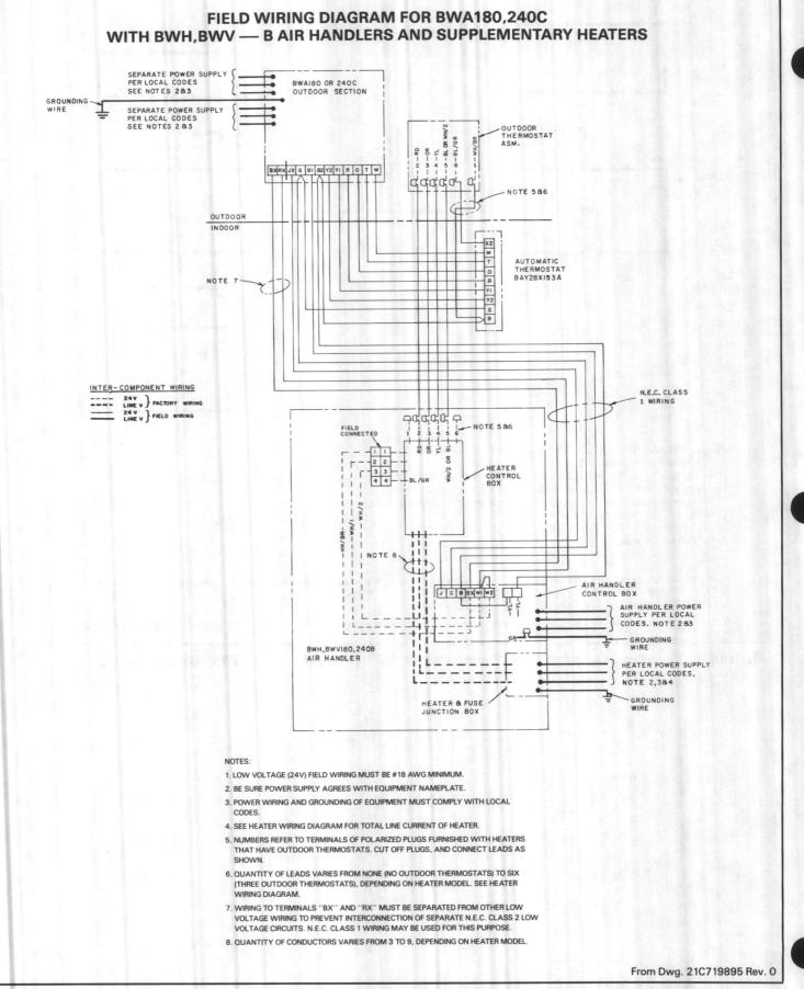
Figure 10 — Typical Interconnecting Wiring for BWA with BWV/BWH Air Handler, Thermostat, and Electric Heat
