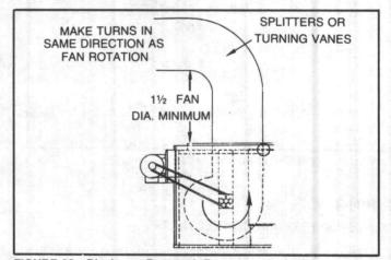
FIGURE 28 - Discharge Ductwork Recommendations
