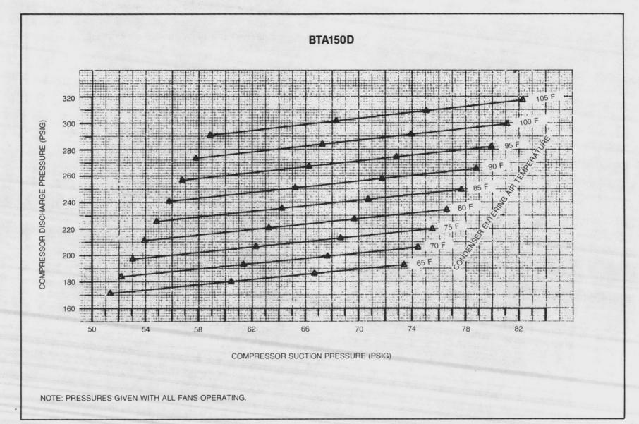
Figure 11 · BTA150D Operating Pressures
