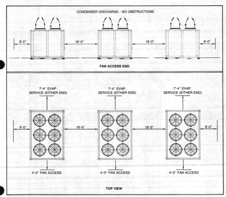
FIGURE 10 - Recommended Clearances for Typical Multiple CGAB C60 Installation.
