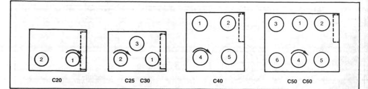
FIGURE 4 - CGAB Condenser Fan Locations
