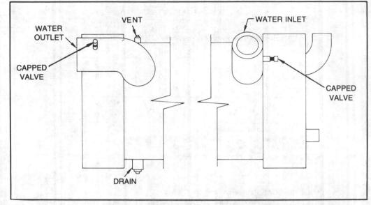
FIGURE 19 - Typical Evaporator Components. Measure Water Pressure Drop at Capped Valves.
