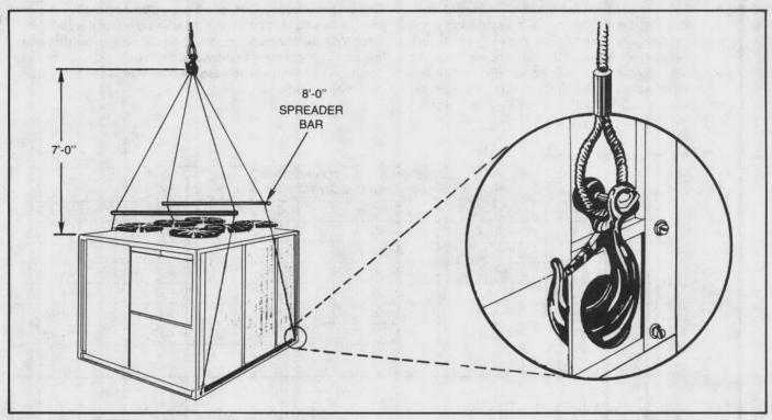
FIGURE 12 - Unit Properly Rigged for Crane or Helicopter Lift.
