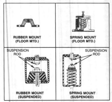
Figure 3 — Typical BWH-BWV Floor and Suspension Type Vibration Isolators
