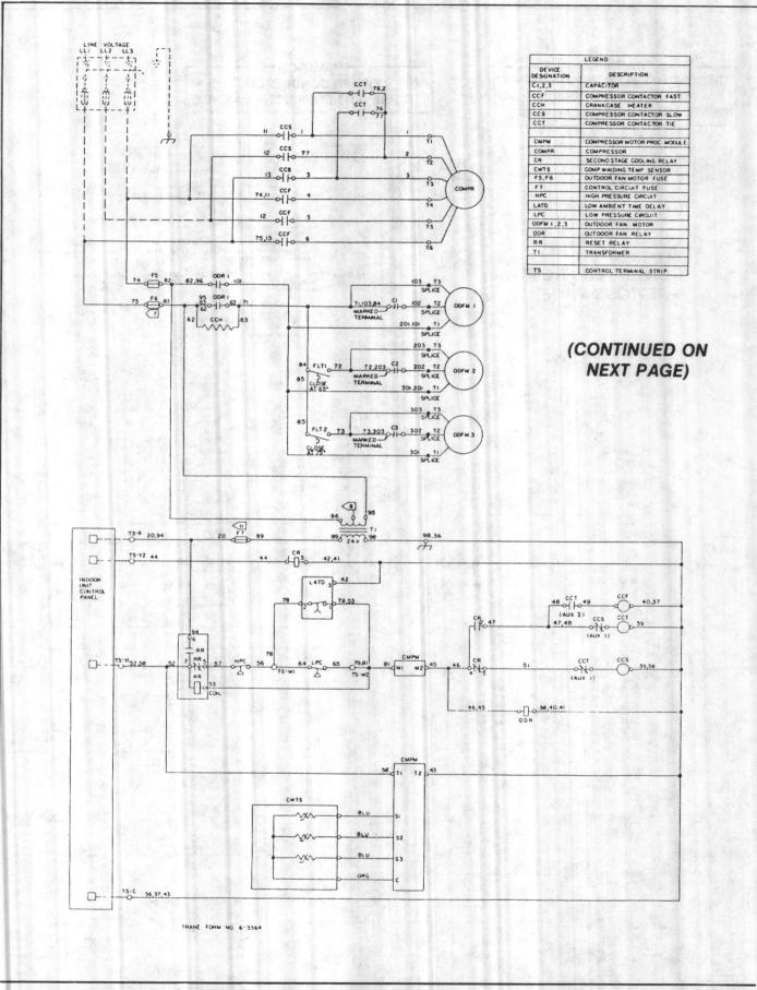
Figure 2 - Typical Unit Wiring Diagram (15 Ton Single Compressor Unit Shown)
