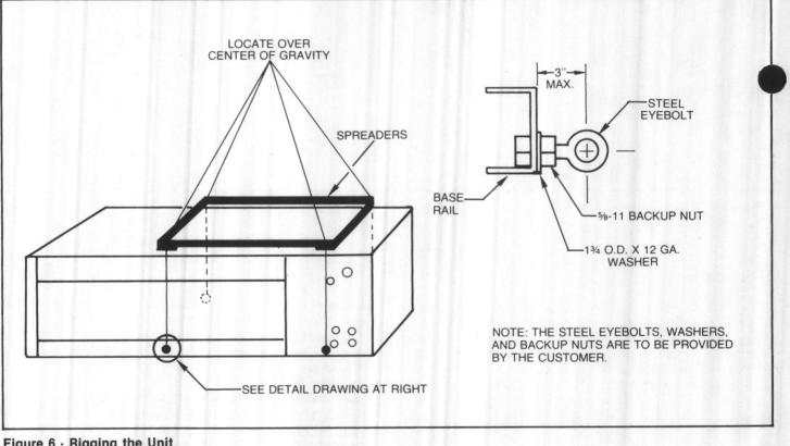
Figure 6 · Rigging the Unit
