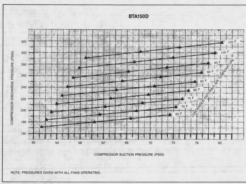
Figure 11 - BTA150D Operating Pressures
