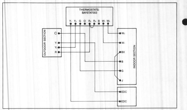
Figure 15 - Field Wiring for BTA150D, BTA180D and BTA180F With the BWV180B, BWH180B Air Handlers With Electric Heat
