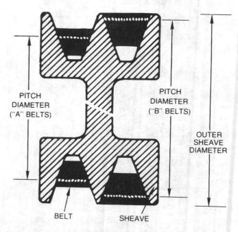
Figure 54 - Fan Sheave Pitch Diameter
