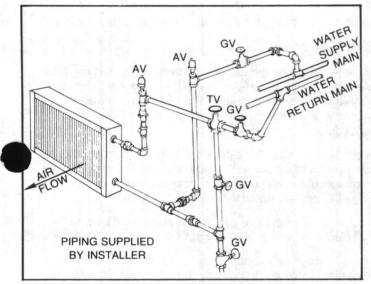
FIGURE 46 - Typical Piping for Type WC Water Coil
