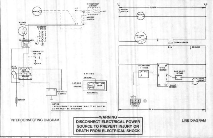
FIGURE 11 - Duct Furnace Wiring Diagram, Single Stage Intermittent Pilot Ignition
