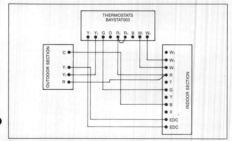
Figure 10 - Field Wiring for BTA120D with BTE120B Air Handler With Electric Heat
