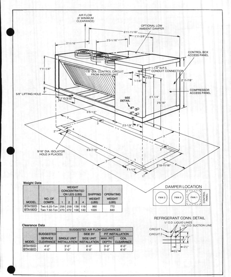
Figure 2 - Dimensions, Weights, and Clearances for BTA150D and 180D Units
