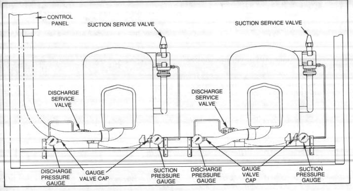
FIGURE 6 - Location of Optional Suction and Discharge Pressure Gauges
