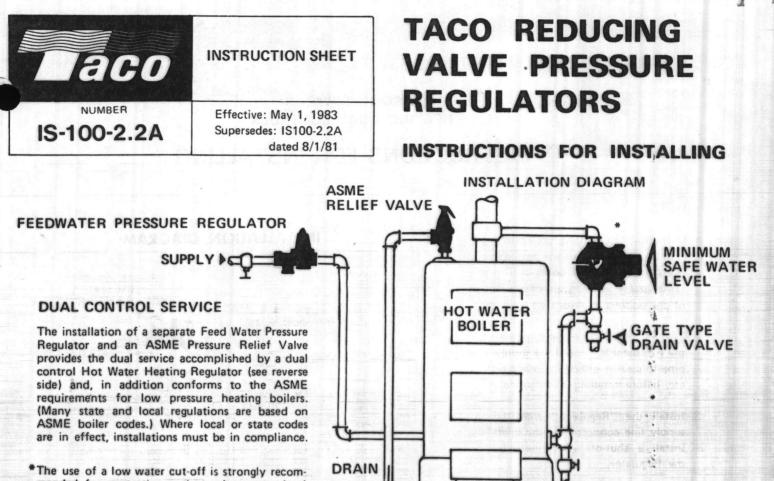
The use of a low water cut off is strongly recommended for protection against a low water level condition in the boiler which could result from continuous firing should controls become inoperative or a break occur in the return piping.
