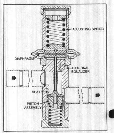
FIGURE 22 - Hot Gas Bypass Valve.
