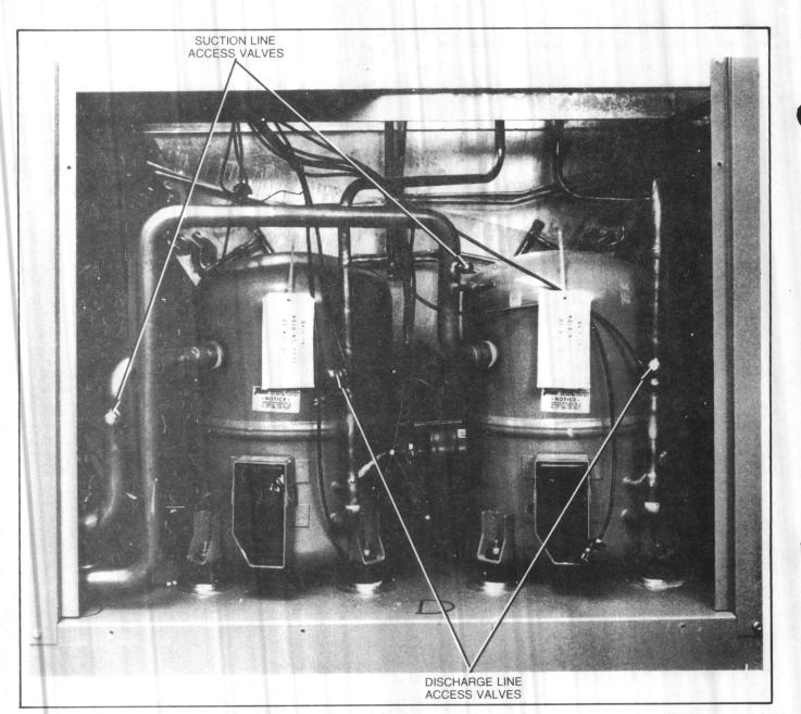
Figure 9 - Compressor Suction and Discharge Access Valves (Dual Compressor Unit Shown)
