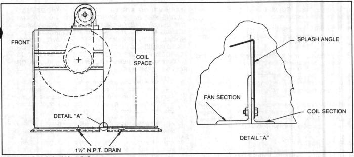
FIGURE 9 - Splash Angle Installation
