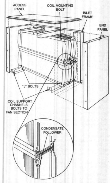
FIGURE 11 - Draw-Thru Coil Section Details with View of Condensate Follower
