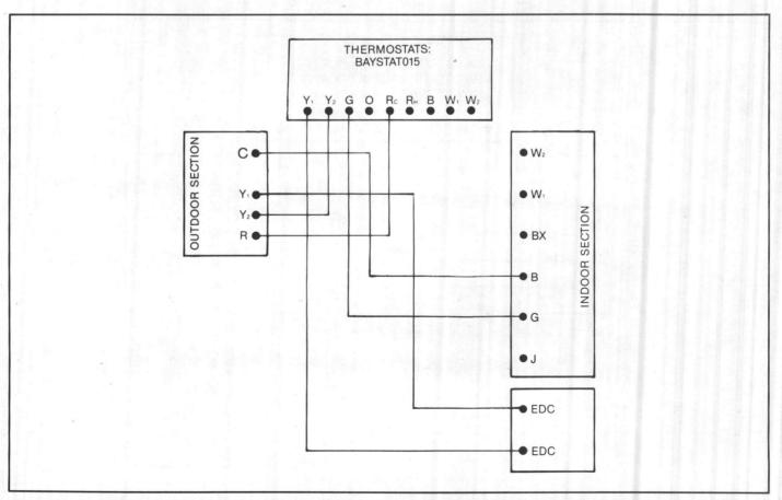
Figure 14 - Field Wiring for BTA150D, BTA180D and BTA180F With the BWV180B, BWH180B Air Handlers Without Electric Heat
