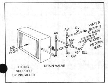
FIGURE 47 - Typical Piping for Type W, Two-Row Water Coil
