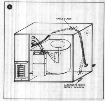
21. When these air handlers are equipped with supplementary heaters in a field converted configuration (rear blower access), assemble cable clamp removed in E-10 around power wiring and attach to air handler cabinet with (1) screw in location shown in figure 4.
