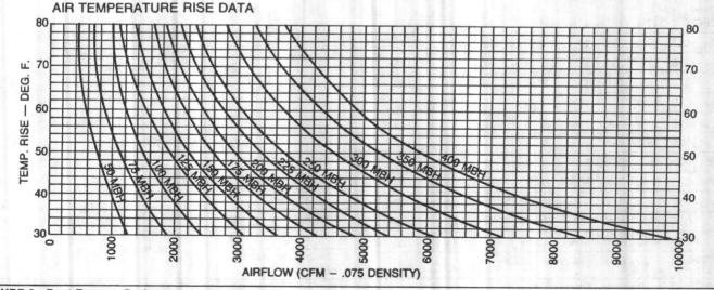
FIGURE 2 - Duct Furnace Performance Data Curve
