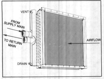
Figure 50A - Typical Piping for 2-Row, Type WL and DL Water Coil with Drain and Vent Locations.
