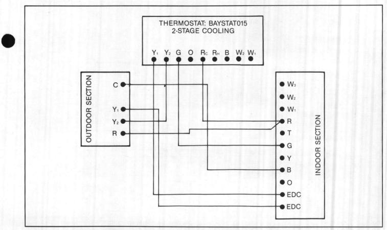
Figure 9 - Field Wiring for BTA120D with BTE120B Air Handler No Electric Heat
