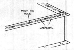
FIGURE 14 - Installation of Gasketing on the Damper Section
