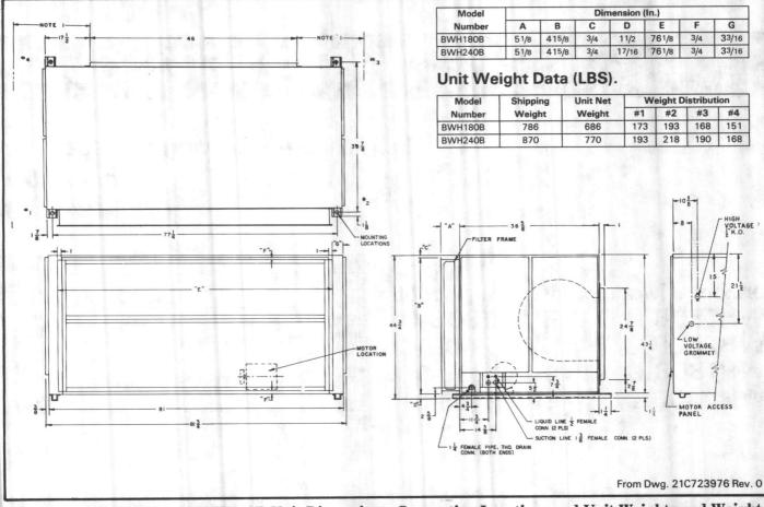
Figure 1 — BWV180B and BWV240B Unit Dimensions, Connection Locations and Unit Weights and Weight Distribution
