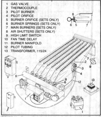
FIGURE 13 - Burner Components
