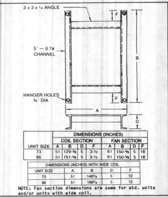
FIGURE 13 - Ceiling Suspension Mounting Frame and Dimensions for Unit Sizes 73 and 86 (Two Frames are Required for Each Unit)
