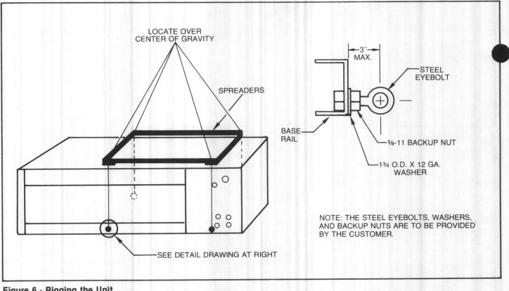
Figure 6 - Rigging the Unit
