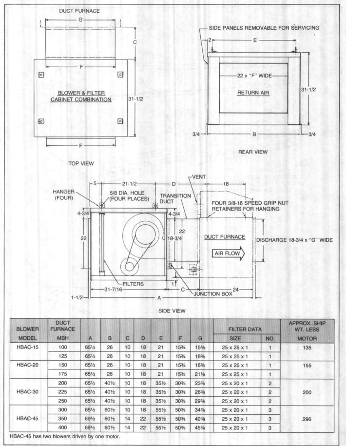
FIGURE 4 - Blower Assembly Dimensions
