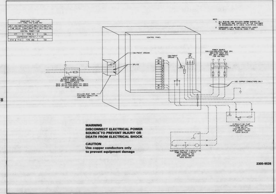
FIGURE 18 - Typical Field (Customer) Wiring. CGAB C40 C50 and C60.
