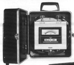
Typical portable differential readout pressure meters.
