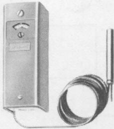
**HYDRONIC CONTROLLERS FOR LIMITING OR REGULATING TEMPERATURES OF BOILER WATER OR LIQUID IN TANKS. CAN ALSO SENSE DUCT OR OUTSIDE AIR TEMPERATURE.**
