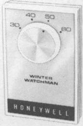
USED AS A FREEZE WARNING DEVICE. COMPLETES CIRCUIT TO HOUSEHOLD LAMP ON TEMPERATURE FALL, INDICATING FAILURE OF HEATING PLANT.
