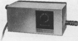
USED WITH F51 IN-PLACE WASH ELECTRONIC AIR CLEANER. TIMER CONTROLS INTERNAL WATER AND DETERGENT VALVES FOR AUTOMATIC WASH AND RINSE OF ELECTRONIC CELLS.
