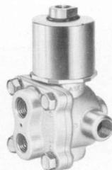
Four way, high-flow, direct acting slide valves can be used without concern for minimum pressure differential when controlling double acting cylinders, actuators, or other similar devices.
