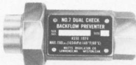
**Ordering Code:** No. 7 can be ordered with various combinations of inlet/outlet (A) sizes, (B) thread types, (C) connection types. A letter "U" is used in prefix to the thread/connection designation and denotes union connection. **Example:** (3/4"x 3/4" - 7-U2-2) valve has 3/4" NPT thread female union inlet connection x 3/4" NPT thread female outlet connection.
