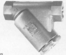
Strainers have stainless steel construction. Bodies ASTM A-316 Grade CF8M. Bottom cap 1/4"- 1/2" 316 stainless steel, 1/4"- 2" CF8M. Steam 600 psi @ 905°F. Liquids 1440 psi @ 100°F.
