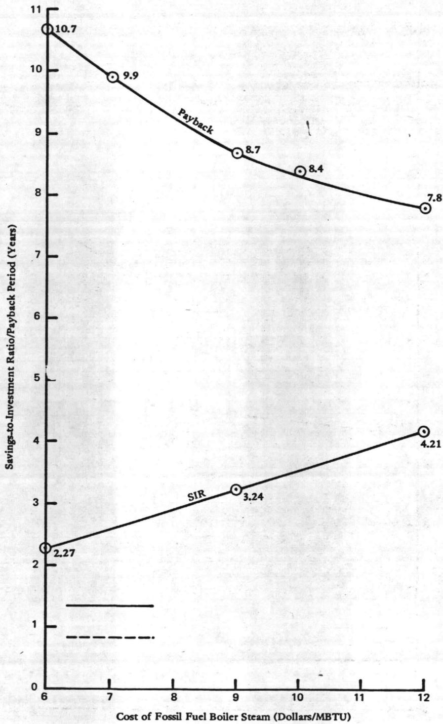
Figure 4. Savings to investment ratio (SIR) and payback period versus cost of fossil fuel boiler steam.
