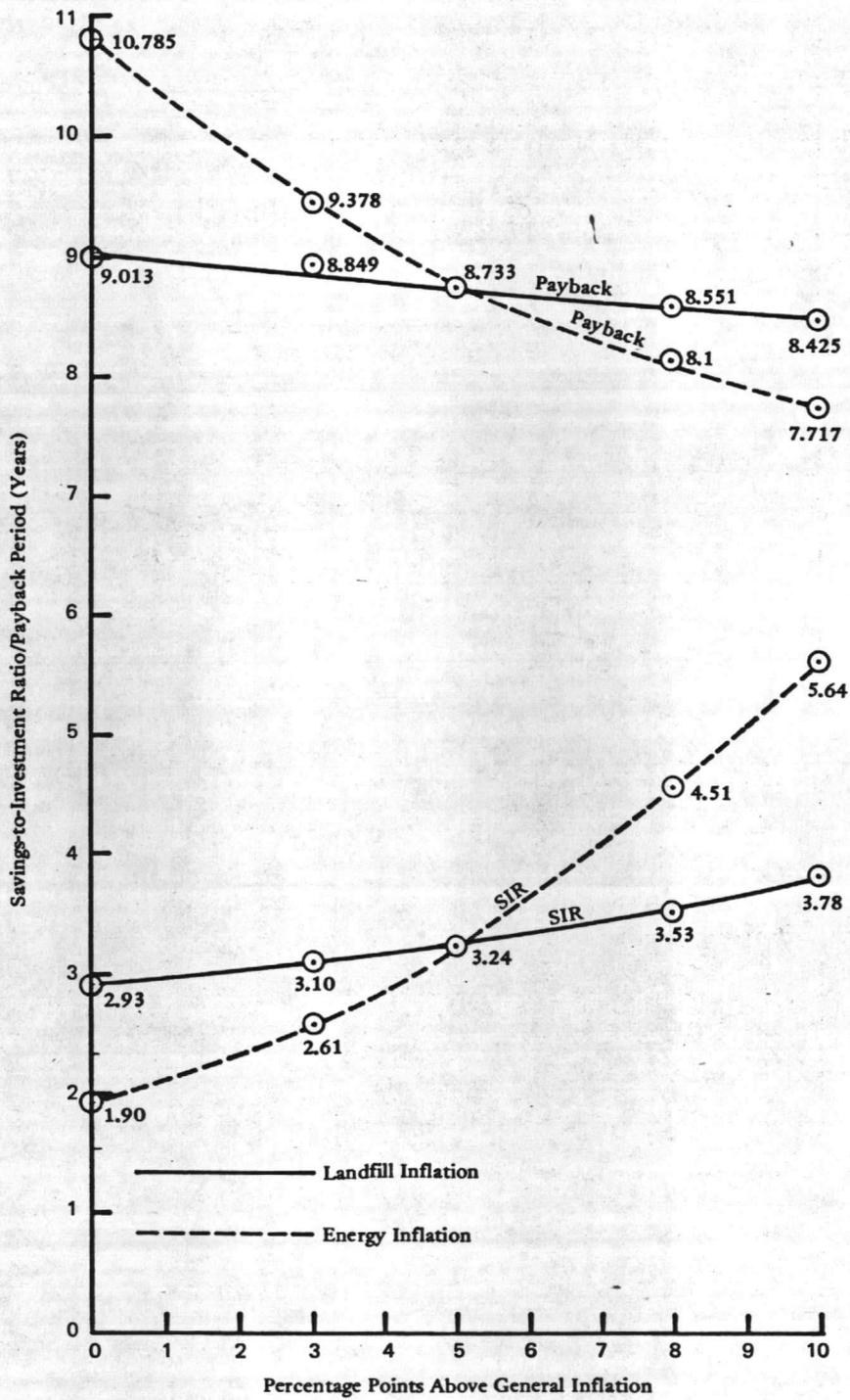
Figure 6. Savings to investment ratio (SIR) and payback period versus differential energy and landfill inflation rates.
