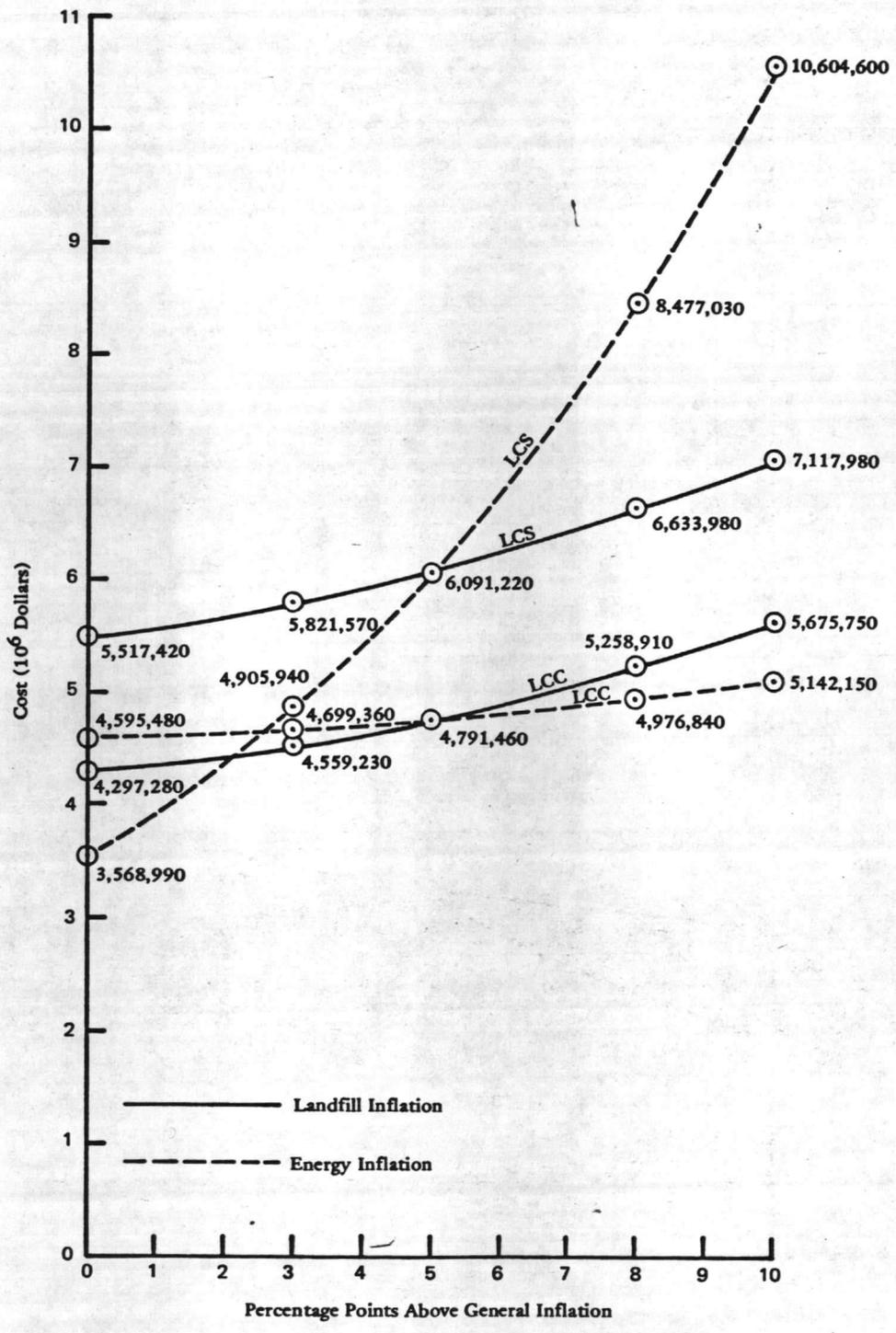
Figure 5. Discounted life cycle cost (LCC) and savings (LCS) versus differential energy and landfill inflation rates.
