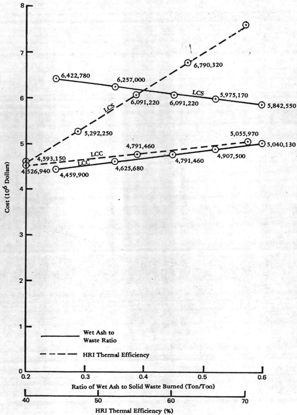
Figure 7. Discounted life cycle cost (LCC) and savings (LCS) versus ratio of wet ash to solid waste and HRI thermal efficiency.
