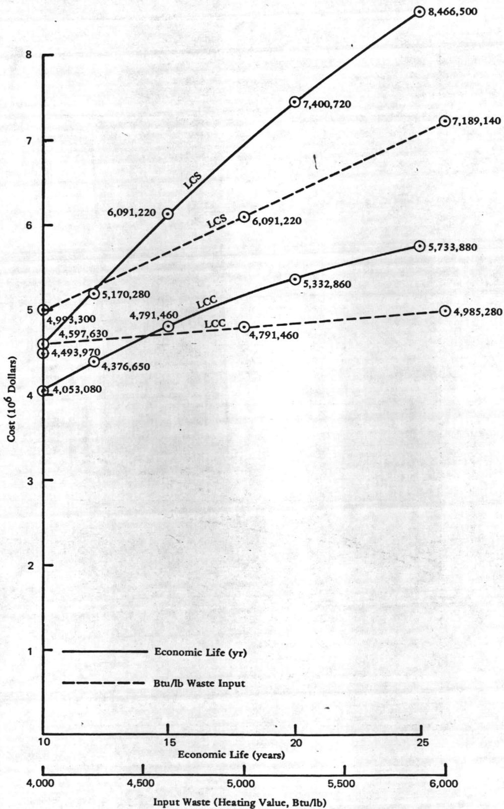
Figure 11. Discounted life cycle cost (LCC) and savings (LCS) versus economic life and input waste heating value.
