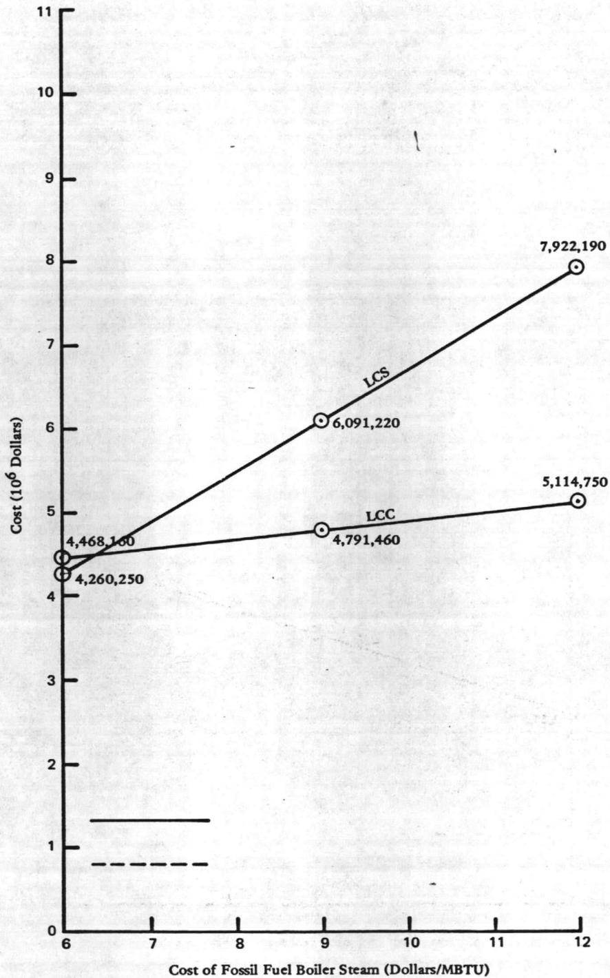
Figure 3. HRI life cycle cost (LCC) and savings (LCS) versus cost of fossil fuel boiler steam.
