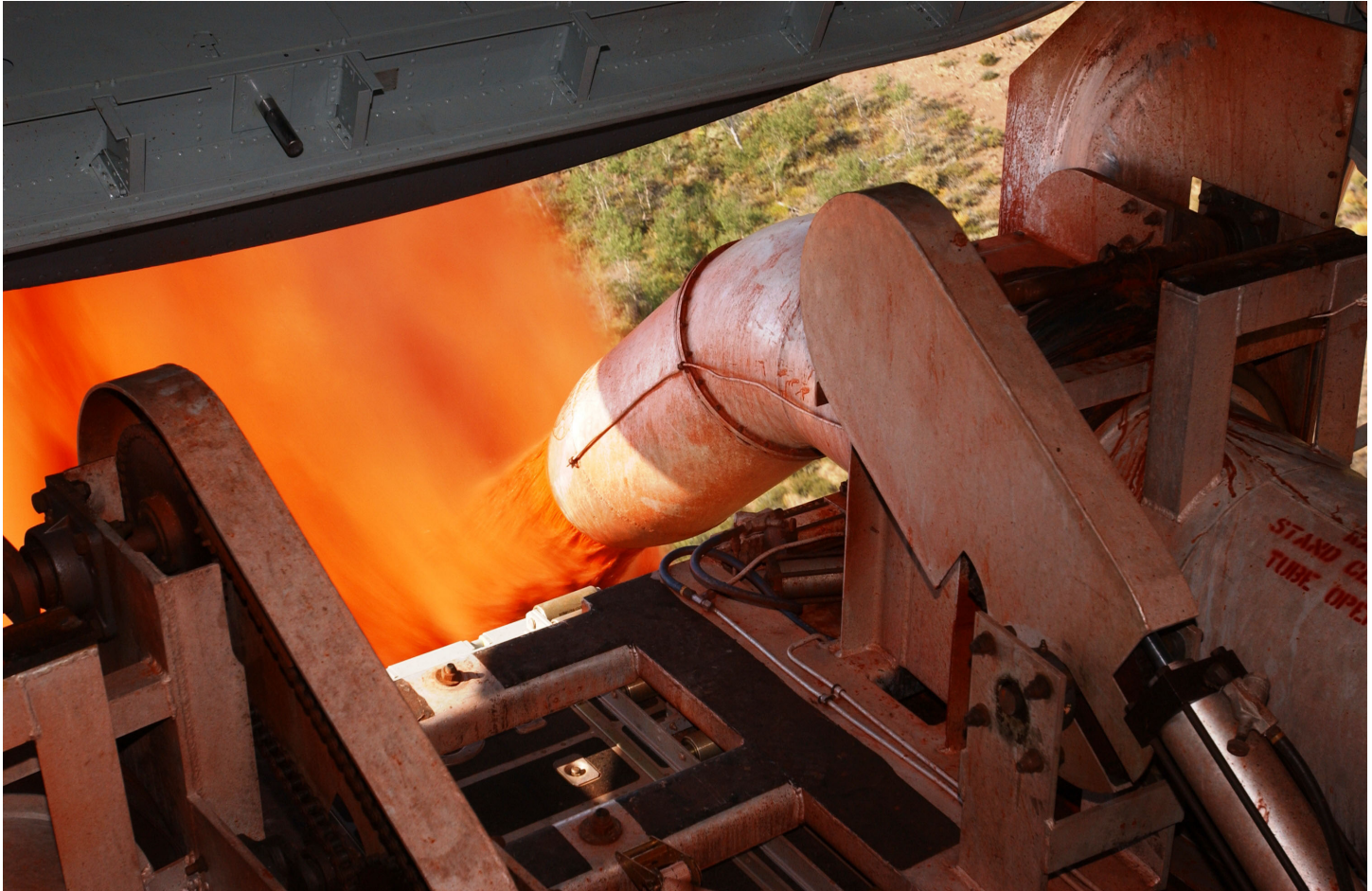
A Peterson Air Force Base, Colo, C-130 Hercules dispenses fire retardant liquid during a Modular Airborne Firefighting System mission in Klamath Falls, Ore. in August 2006. A MAFFS unit can discharge its load--3,000 gallons weighing 28,000 pounds--in a little over five seconds. (U.S. Air Force photo/Tech Sgt. Lee Harshman)
