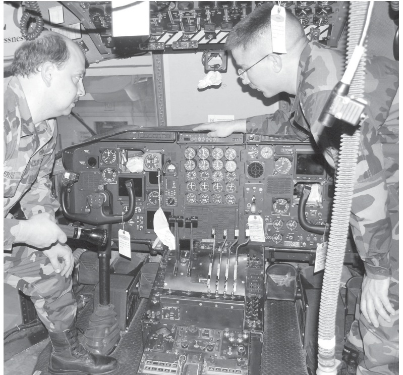
Tech. Sgts. Howard Ertle (left) and Jason Wiley, 302nd Maintenance Squadron aircraft maintenance journeymen, inspect the instrument panel of a C-130 aircraft during an annual isochronical inspection. (U.S. Air Force photo by Tech. Sgt. David D. Morton)
