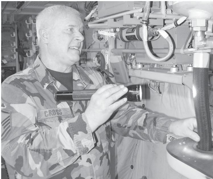
Master Sgt. Richard Cross, 302nd Maintenance Squadron aircraft maintenance journeyman inspector, inspects the hydraulic lines on one of a C-130 aircraft during an annual isochronal inspection. (U.S. Air Force photo by Tech. Sgt. David D. Morton)
