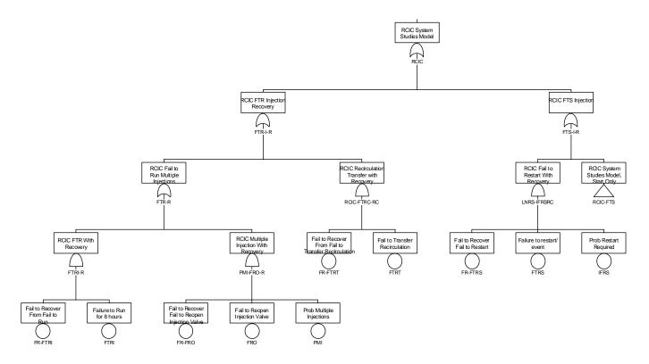
Figure 1. Unreliability model of RCIC system for an 8-hour mission.
