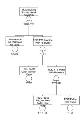
Figure 2. Unavailability model of RCIC system for a start only mission.
