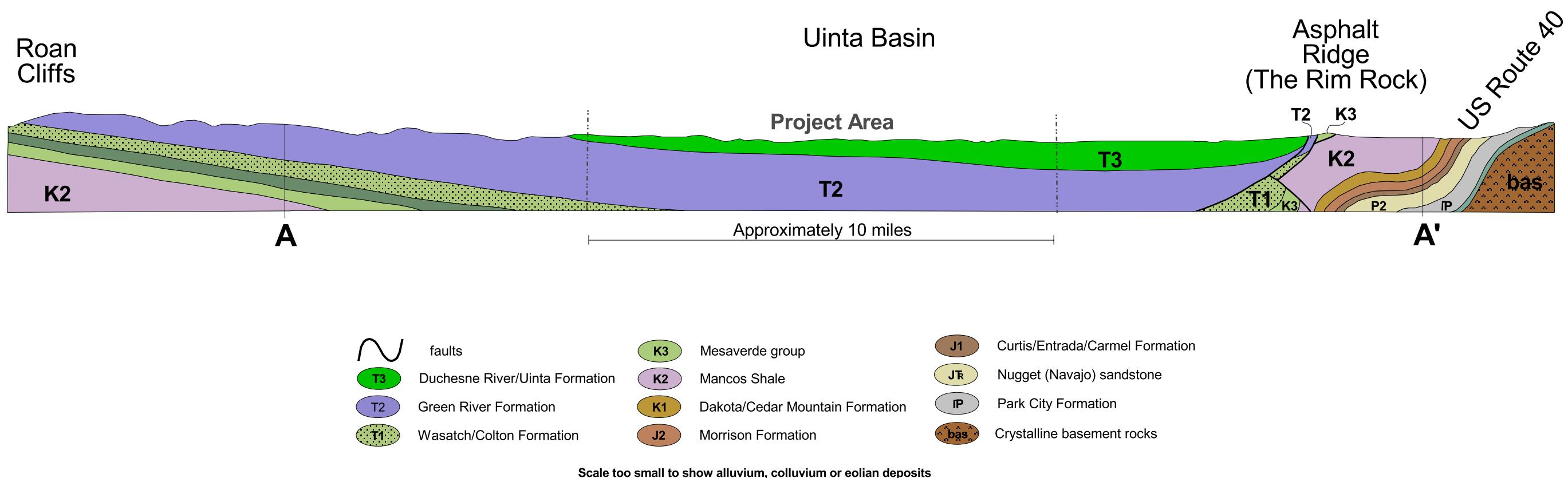
Figure 3.1-3. Geologic Cross-section.
