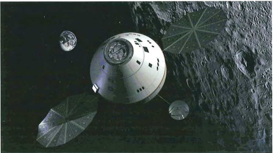
NASA's Constellation Program is getting to work on the new spacecraft that will return humans to the moon and be capable of delivering crews and cargo to the space station. The new spacecraft will be similar in shape to the Apollo spacecraft but significantly larger. The tried-and-true conical form is the safest and most reliable for re-entering Earth's atmosphere. This artist's rendering represents a concept of the Orion Crew Exploration Vehicle in orbit with the moon and Earth in the background. (jsc2008e097002)
