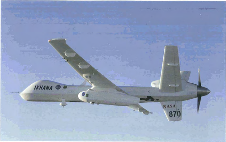
With its thermal-infrared sensor pod under its left wing, NASA's Ikhana unmanned aircraft cruises over California during the Western States Fire Mission. (ED07-0186-13)
