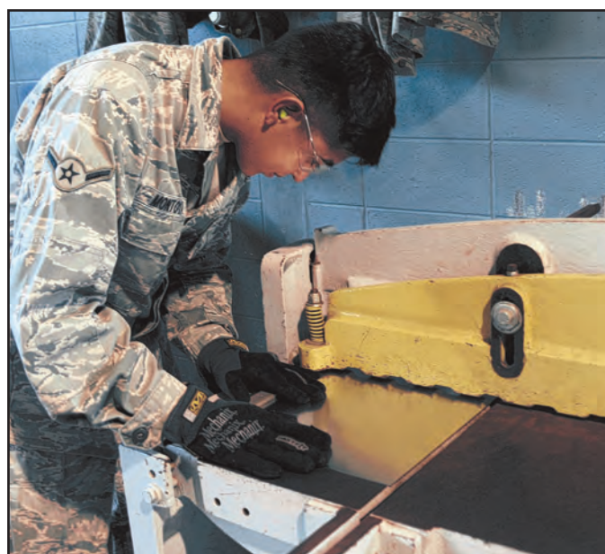
Top, Airman Oscar Montoya cuts sheet metal to make a model air conditioning duct.
