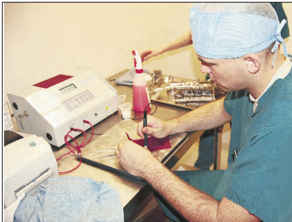
Photo by Steve Pivnick Airman 1st Class Karol Kowalczyk, 81st Surgical Operations Squadron, electrochemically etches a two-dimensional bar code on a surgical instrument March 26 in central sterile supply. With the bar codes instruments can be individually tracked and information is readily available, such as when they were last used or sterilized and in which surgical package they are located.
