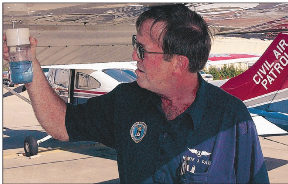
Photos by Staff Sgt. Tanya Holditch First Lt. Monte David, CAP Diamondhead Composite Squadron pilot, checks the aircraft's fuel for water during the preflight inspection of the Cessna 172 Skyhawk.
