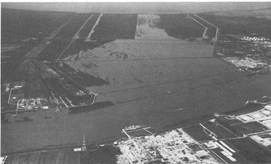
BONNET CARRE SPILLWAY. The above photo of the Bonnet Carre Spillway was taken during the flood of 1973, when the control structure was opened to relieve pressure on the mainline levee system. The Mississippi River is in the foreground, and at the foot of the floodway is Lake Ponchartrain.
