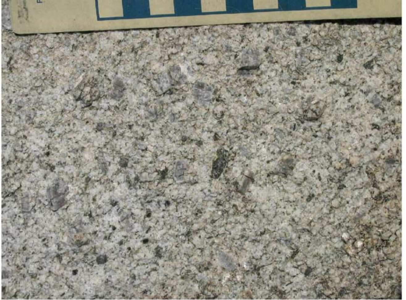
Figure 3.3 Porphyritic granite of the Jurassic Yerington batholith, showing large purplish K-feldspar phenocrysts, mafic crystals (hornblende and biotite) and a small, fine-grained mafic xenolith (just right of center) in a medium-grained, equigranular matrix. Scale in cm. From 3 to 5 m above floor of pluton in the southeast part of Luhr Hill.
