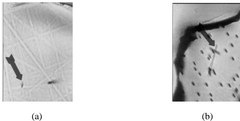
Figure C.1. Transmitted light photomicrographs taken at 1562.5x magnification of two apatite crystals from the same sample that exhibit low natural fission-track densities. (a) not irradiated with ^{252}\text{Cf} fission fragments (arrow indicates a natural fission track).
