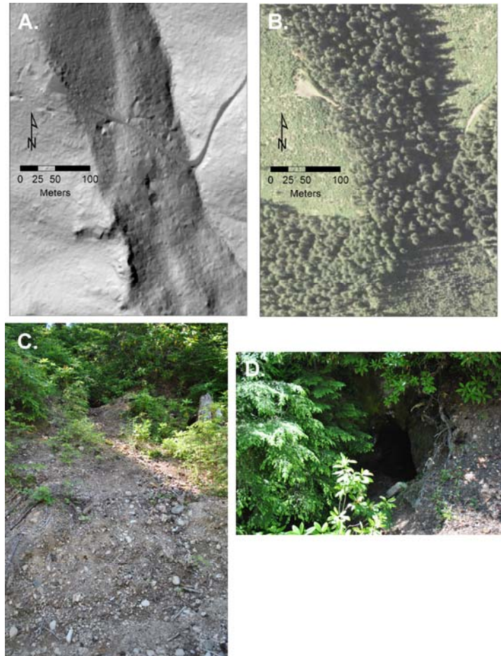
Figure 10. A. Hillshade of LiDAR-derived DEMs from the Blue River mining district, Oregon. B. National Agricultural Imagery Program (NAIP) photograph of the area in A. C, D. Field photographs of minor prospect shown in the center of A. and B.
