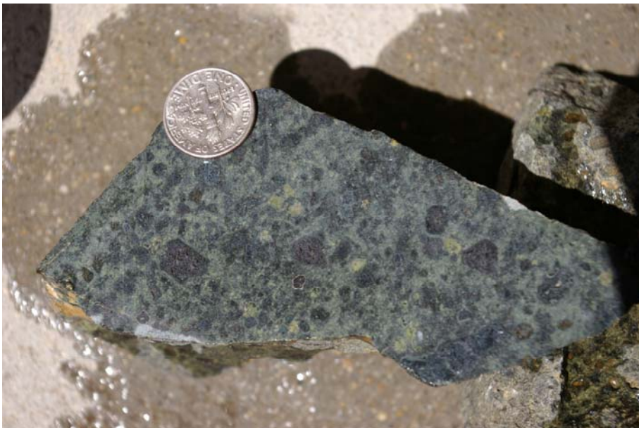
Figure 8. Pyroxene Porphyry from Copper Queen mine dump. Sample CQ06-30. Note large euhedral pyroxenes and green altered phenocrysts.
