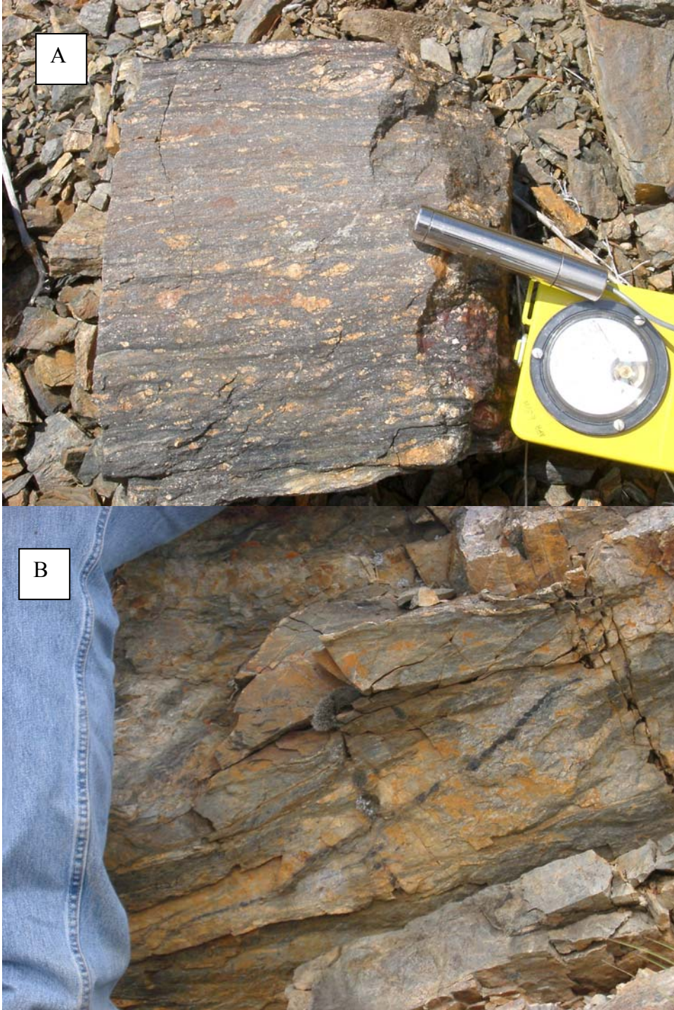
Figure 20. Lucky Horseshoe mine. Top photo (A) shows cataclasite with radioactive thorium ore. Black color is due to biotite and hematite. Tan-colored clasts are feldspar and/or apatite. Bottom Photo B shows some of the tan alkali feldspar veins which are peripheral, especially in the hanging wall of the deposit. Thin sections and geochemical analyses indicate the tan veins have both Na and K feldspars.
