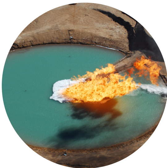
LNG experiment at Sandia's outdoor lake facility
