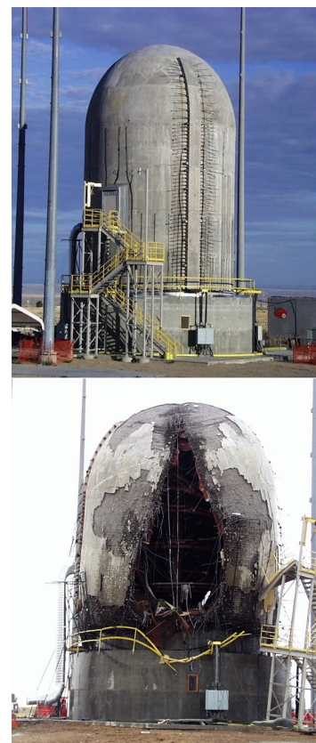
The largest nuclear reactor containment vessel model ever tested to failure
