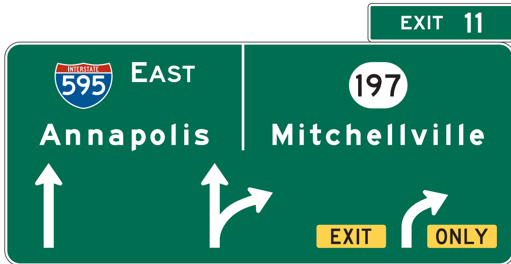
Figure 2E-3. Overhead Arrow-per-Lane Guide Sign for a Multi-Lane Exit with an Option Lane
