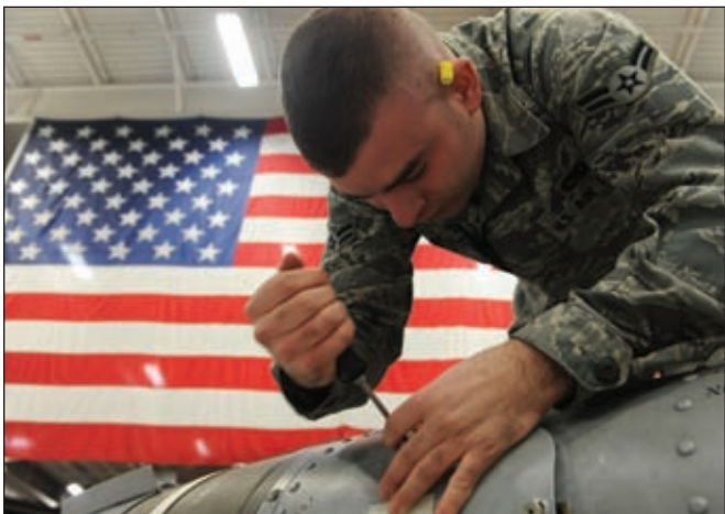
Airman 1st Class Benjamin Koch, 509th Aircraft Maintenance Squadron 13th Ammunitions load crew member, closes the fuse access cover on a mock GBU-31, Jan. 25.
