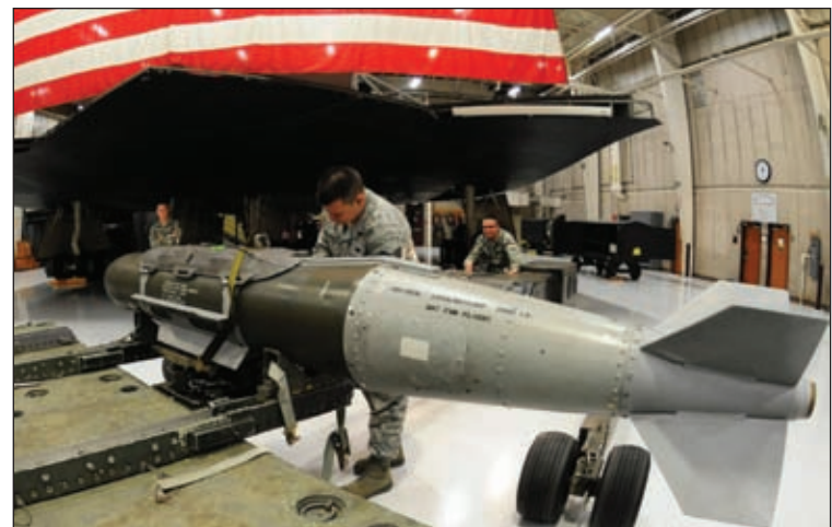
Staff Sgt. Stephan Capkovic, 131st Aircraft Maintenance Squadron load crew team member, ensures the mock GBU-31 is safely picked up by the bomb-lift truck, Jan. 25.
