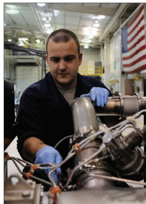
Staff Sgt. Cole Adams, 509th Maintenance Squadron aerospace ground equipment mechanic, tightens bolts on a -95 air start cart gas turbine compressor here Jan. 31. The gas turbine is an internal combustion engine that uses air as the working fluid. The engine extracts chemical energy from fuel and converts it to mechanical energy using the gaseous energy of the working fluid to drive the engine and propeller, which, in turn, propel the aircraft.
