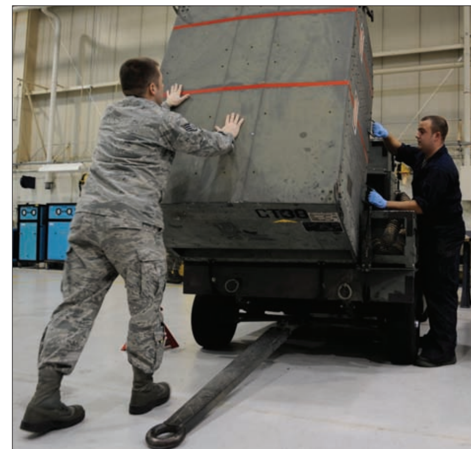
Staff Sgt. Cole Adams (right) and Calvin Grosz (left), 509th Maintenance Squadron aerospace ground equipment mechanics, lift the top off of a -95 air start cart gas turbine compressor for routine maintenance here Jan. 31. The gas turbine is an internal combustion engine that uses air as the working fluid.
