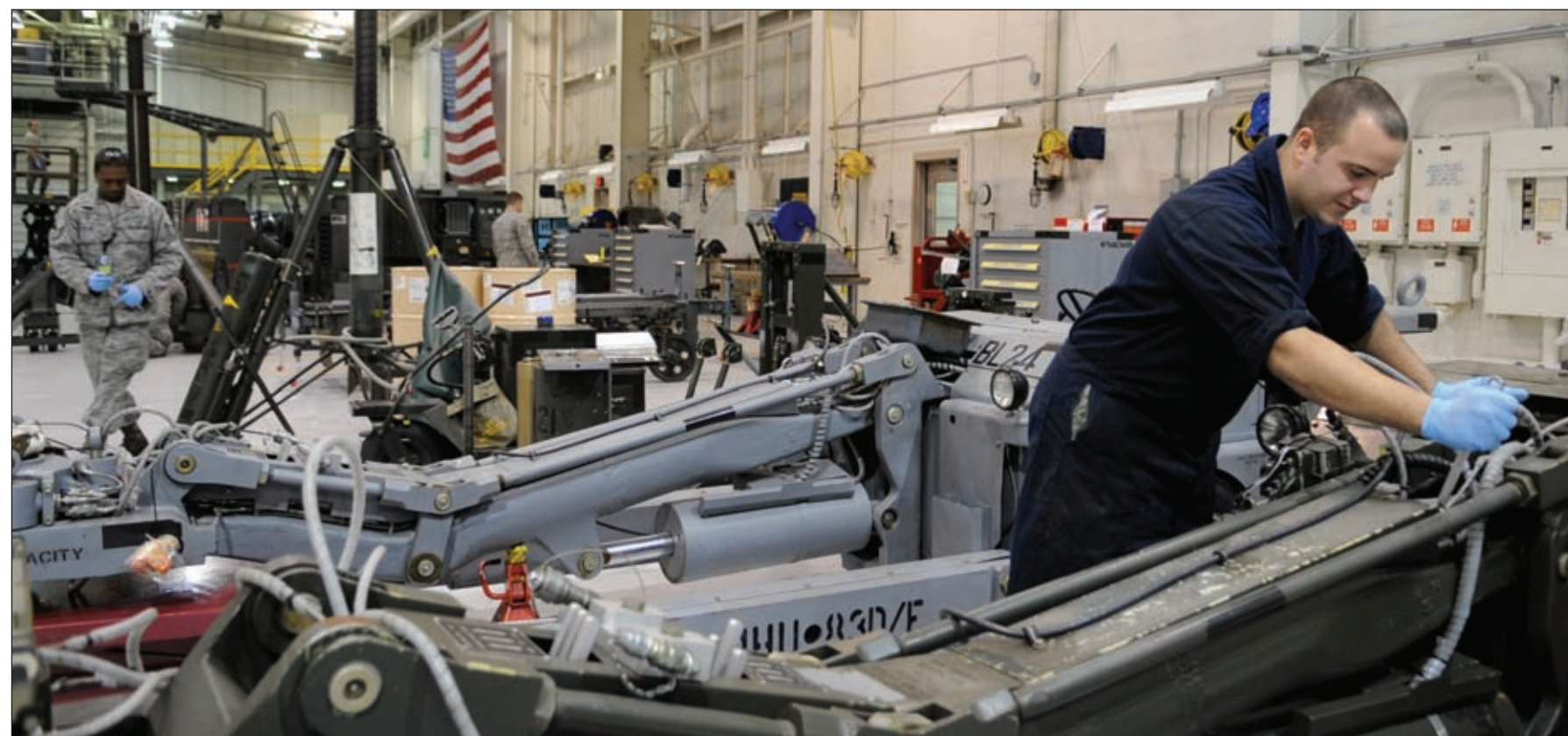
Staff Sgt. Cole Adams, 509th Maintenance Squadron aerospace ground equipment mechanic, ensures everything works properly on the MHU-83 bomb lift, also known as a Jammer, here Jan. 31. Adams has worked on bomb lifts for over four years and is his favorite piece of equipment to work on.
