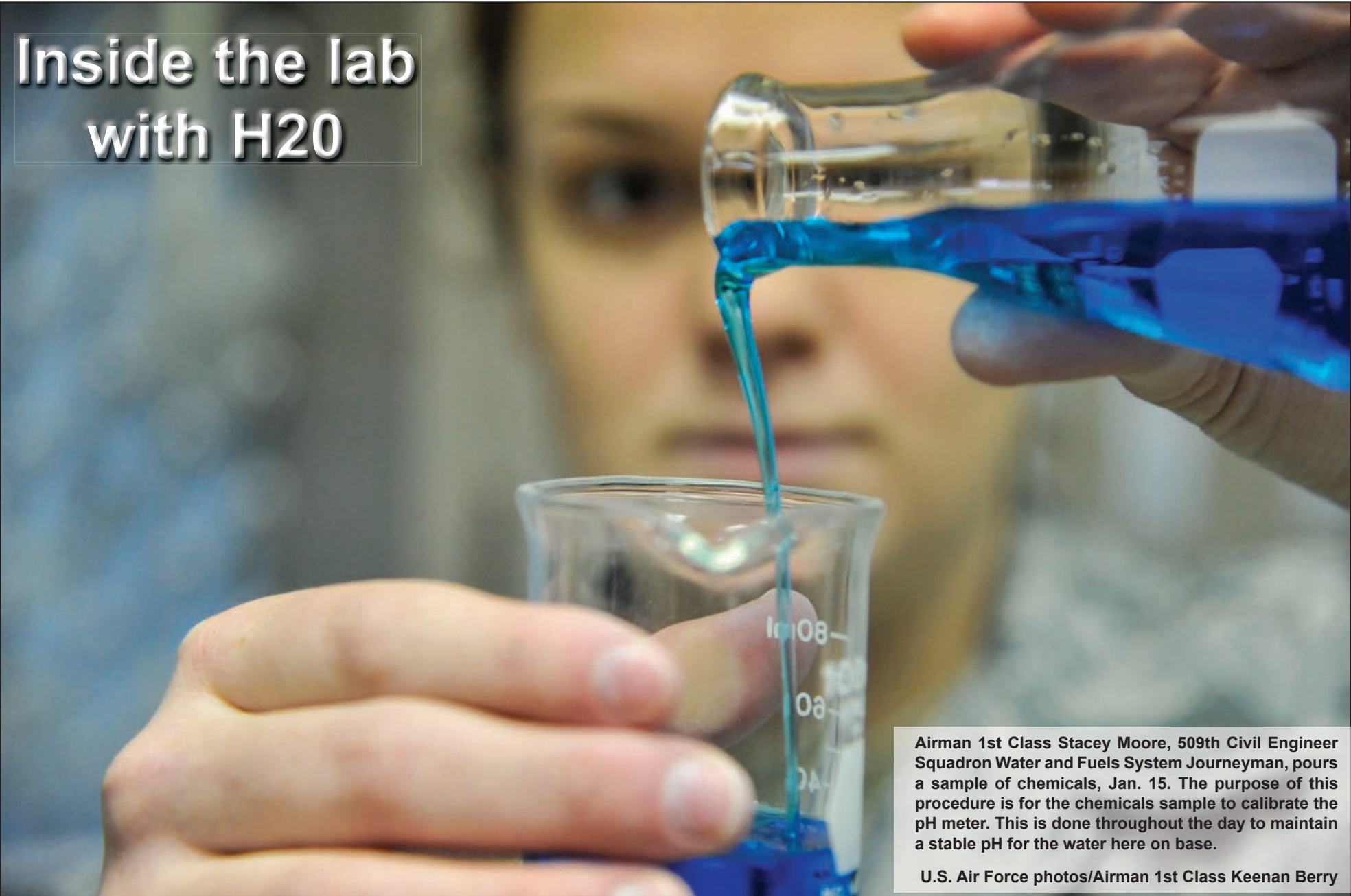
Airman 1st Class Stacey Moore, 509th Civil Engineer Squadron Water and Fuels System Journeyman, tests a water sample, Jan. 15. This procedure is used to gather total hardness of water sample to check if any changes are needed to the chemicals that go into the water.
