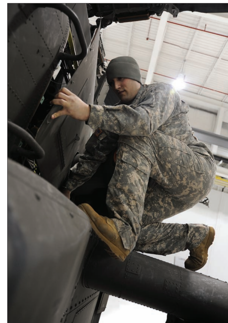
U.S. Army Specialist Jonathan Reed, 1-135th Attack Reconnaissance Battalion AH-64D Apache Longbow crew chief, closes a panel on an AH-64D Apache Longbow during a daily inspection, Jan. 16. Inspecting components in panels is part of the daily inspection Apache crew chiefs must complete.
