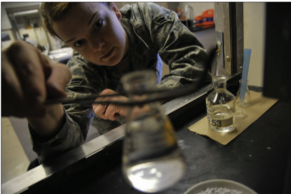
Airman 1st Class Stacey Moore, 509th Civil Engineer Squadron Water and Fuels System Journeyman, retrieves a water sample for testing purposes, Jan. 15. Airman Moore is prepares samples for testing in the lab. Tests need to be made to make sure pH levels are balanced and stabled.
