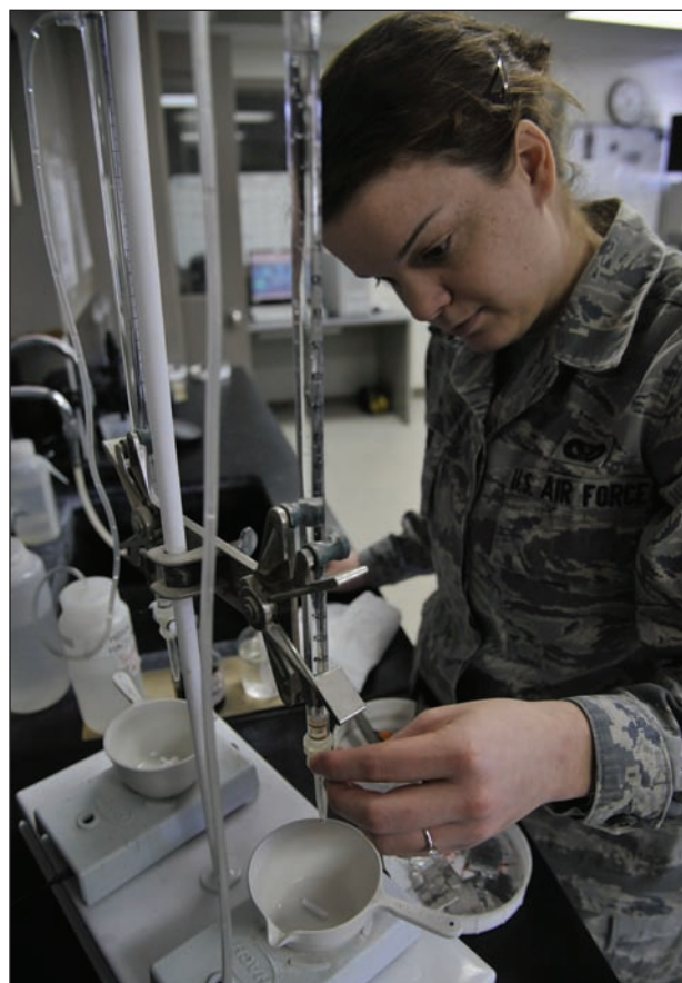
Airman 1st Class Stacey Moore, 509th Civil Engineer Squadron Water and Fuels System Journeyman, rinses the pH stick with a water sample, Jan.15. By rinsing the pH stick with the same water sample, the pH reading will be as accurate as possible.
