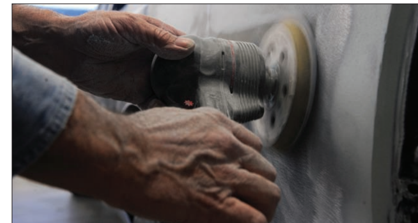
A member of the 509th Logistics Readiness Squadron vehicle maintenance shop sands the back of a truck in the auto body section, Nov. 20. Vehicle maintenance has its own body shop to repair government vehicles that may be involved in accidents, and they also have the tools to repaint the vehicles.
