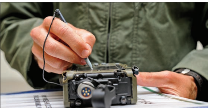
Maj. Joseph Knothe, 509th Operations Support Squadron assistant director of operations, performs an operational inspection on a key loader July 3. The key loader will assist Knothe in acquiring secure communications with comrades in the event of an in-flight emergency.
