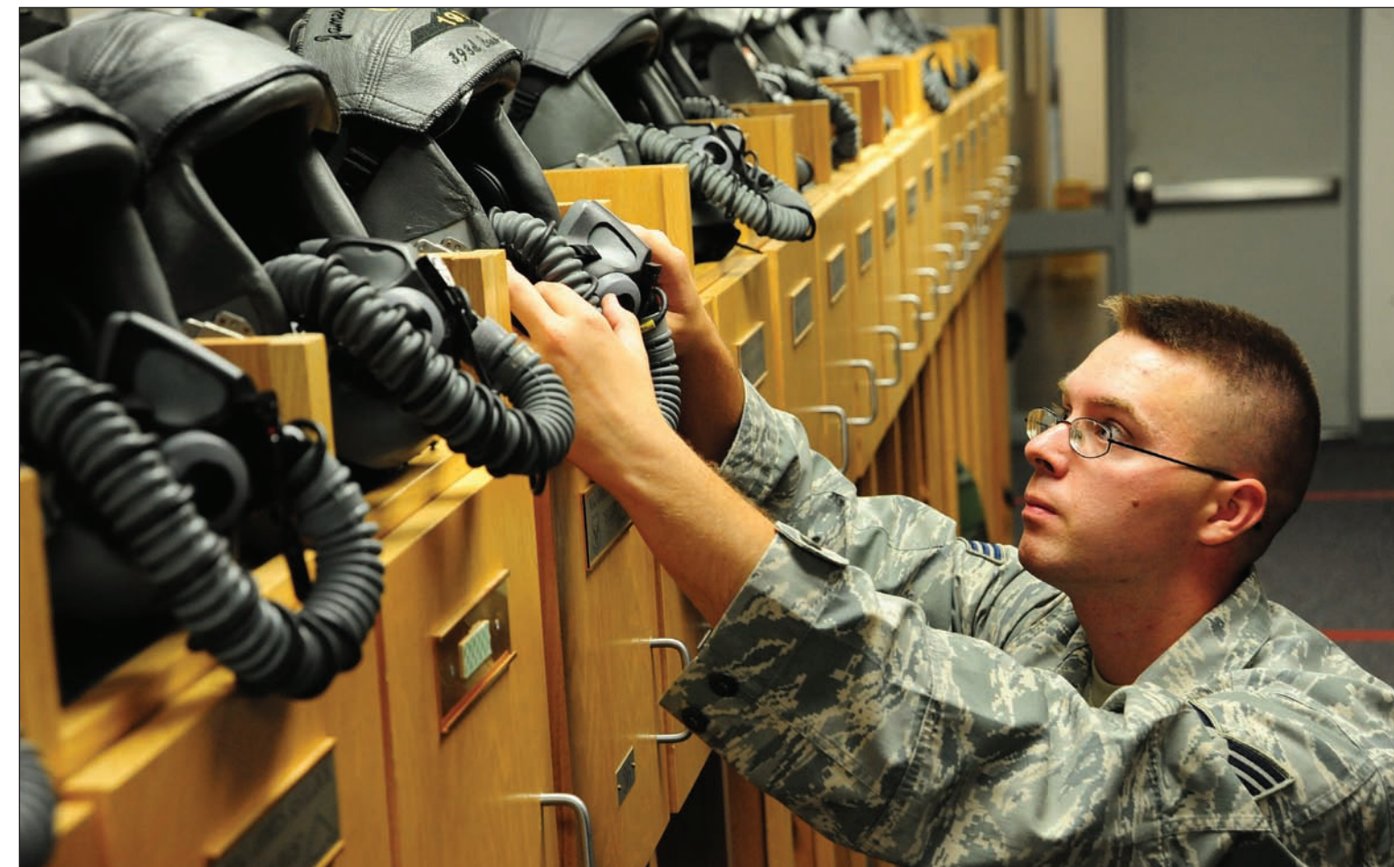
Senior Airman Justin Dunford, 509th Operations Support Squadron Aircrew Flight Equipment journeyman, tests the operational capabilities of an oxygen mask July 3. Technicians perform pre-flight, post-flight and 30-day safety checks of the helmets to ensure they can be used at a moment's notice.
