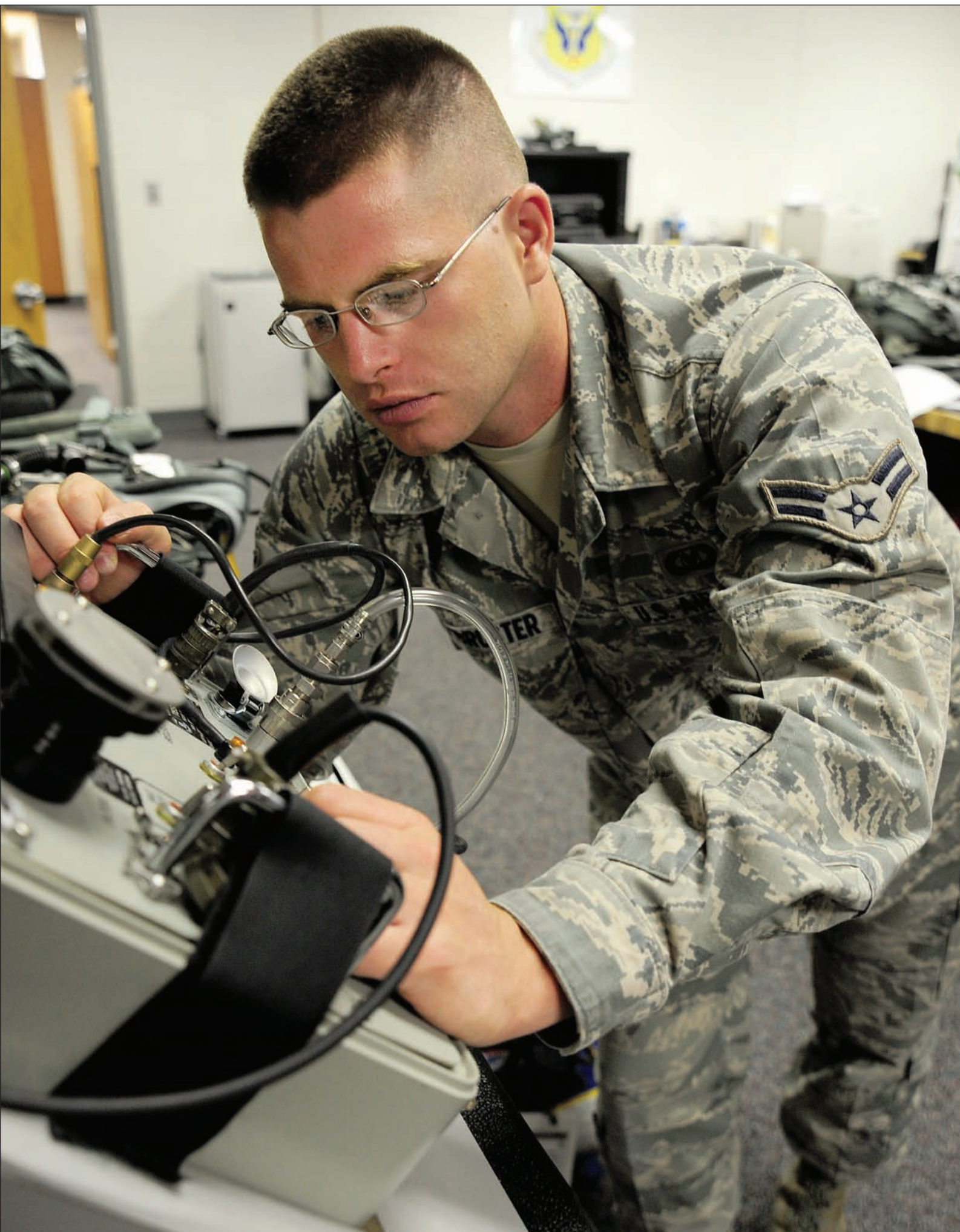
Senior Airman Justin Dunford, 509th Operations Support Squadron Aircrew Flight Equipment journeyman, tests the operational capabilities of an oxygen mask July 3. Technicians perform pre-flight, post-flight and 30-day safety checks of the helmets to ensure they can be used at a moment's notice. See pages 8-9 for story and more photos.
