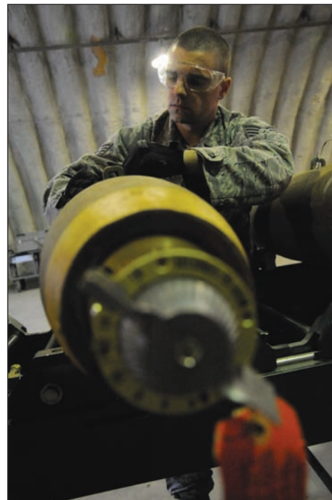
Senior Airman Brady Curtis-Quackenbush, munitions technician, builds bombs for a live-employment exercise with the A-10 Thunderbolt II aircraft assigned to the 442nd Fighter Wing. The munitions technicians are assigned to the 442nd Maintenance Squadron, part of the 442nd FW, Air Force Reserve unit at Whiteman Air Force Base, Mo.
