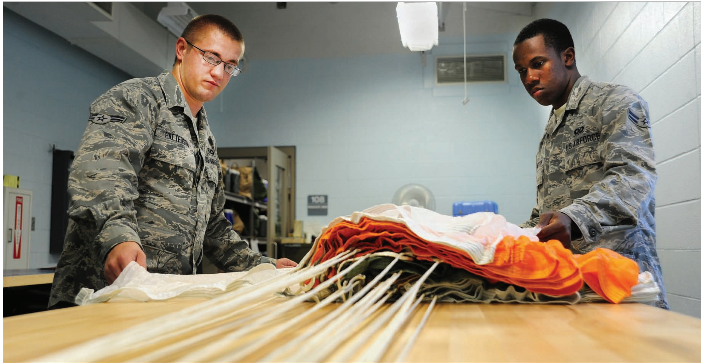
Airman 1st Class Anthony Patterson and Airman 1st Class Dalvin Washington, 509th Operations Support Squadron Aircrew Flight Equipment apprentices, perform maintenance as part of a checklist for packing parachutes July 9. The checklist must be completed when packing parachutes to ensure the parachute is packed correctly and safely.
