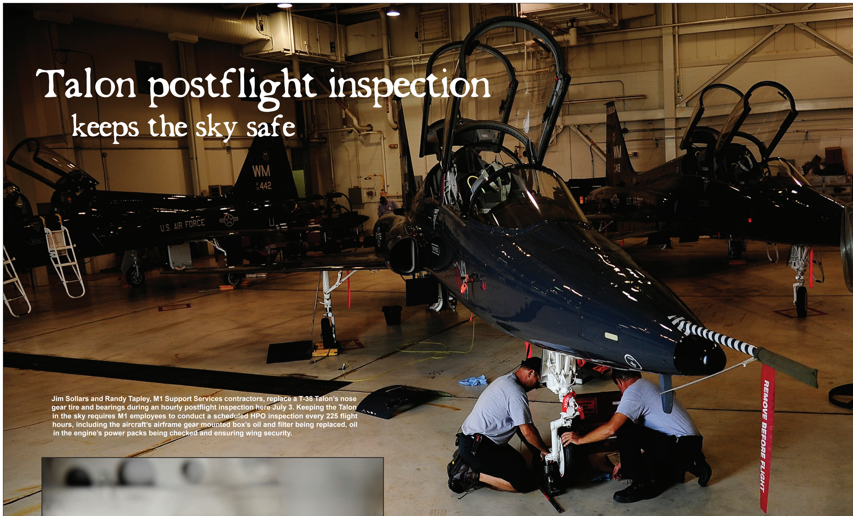
Jim Sollars, M1 Support Services contractor, places a new tire on a T-38 nose gear during an hourly postflight inspection July 3. An HPO inspection is conducted when a Talon accrues 225 flight hours.
