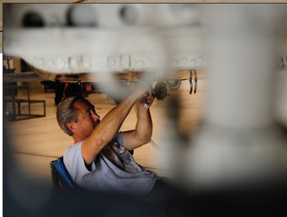
Jim Sollars, M1 Support Services contractor, closes an airframe gear mounted box of a T-38 Talon with safety wire after replacing the oil and filter July 3.
