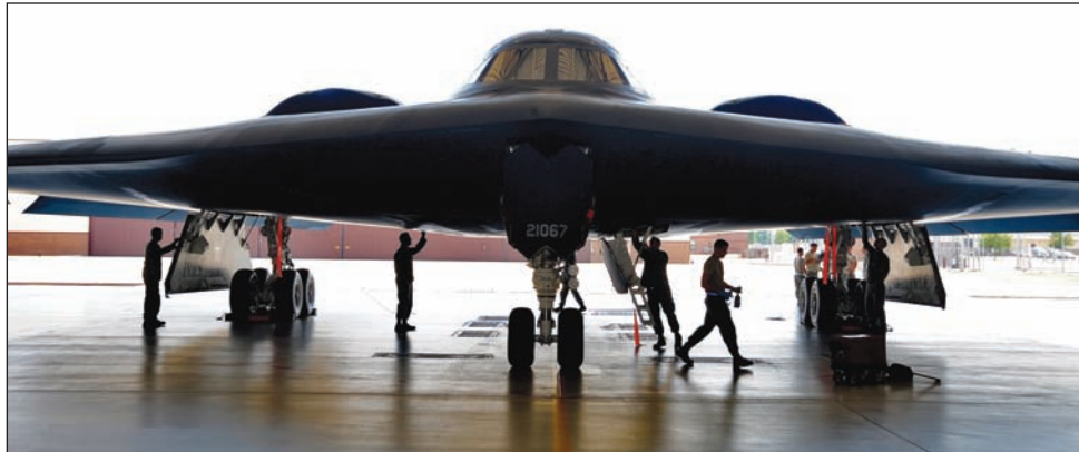
U.S. Air Force photo/Senior Airman Nick Wilson Crew chiefs from the 509th Aircraft Maintenance Squadron and the 131st Bomb Wing perform a phase inspection a B-2 Spirit, July 12. Every 1000 flight hours the B-2 must be 'phased' in search of any discrepancies that could cause major damage.
