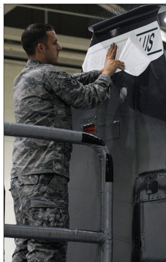
Tech. Sgt. Chad Coshenet, 509th Maintenance Squadron, low observable technician, places a stencil on the T-38 Talon Static Display June 11. The T-38 underwent scheduled maintenance and painting.
